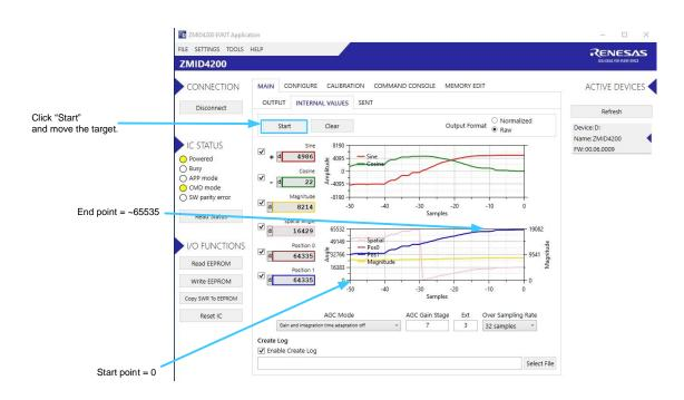
Figure 14. Output Calibration Verification
