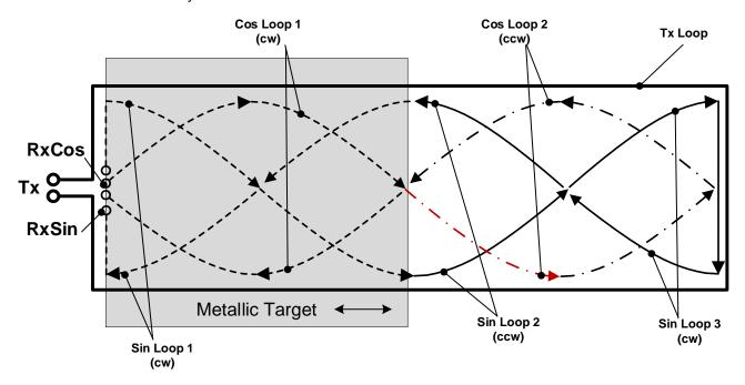
Figure 2. Current Paths and Shapes for Coils - Example for Linear Position Sensing
