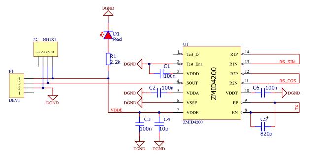
Figure 5. ZMID4200 Transmitter LC Tank
