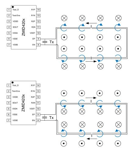
Figure 1. Tx Loop Magnetic Field
