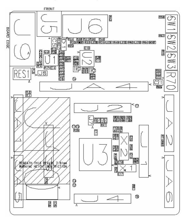
Figure 11-1: Component Placement
