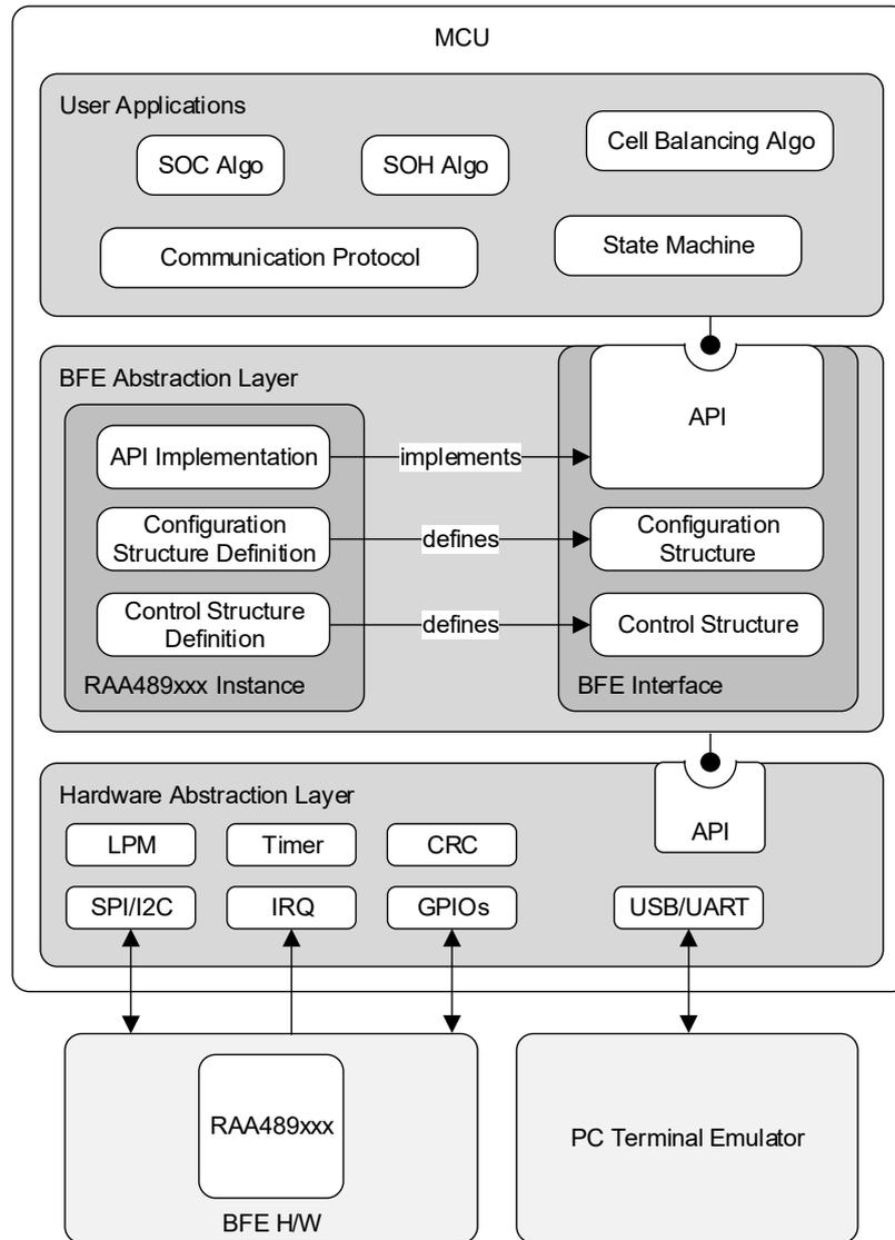
Figure 2. General Software Structure with BFE API
