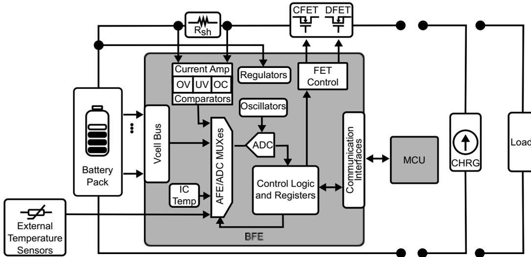
Figure 1. General Block Diagram of Battery Management System
