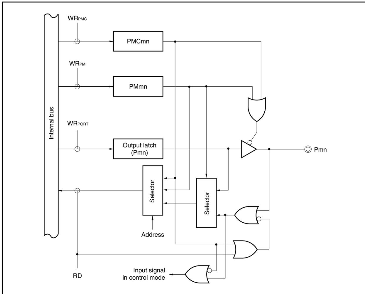
Figure 4-3. Block Diagram of Type A-2 (1/2)
