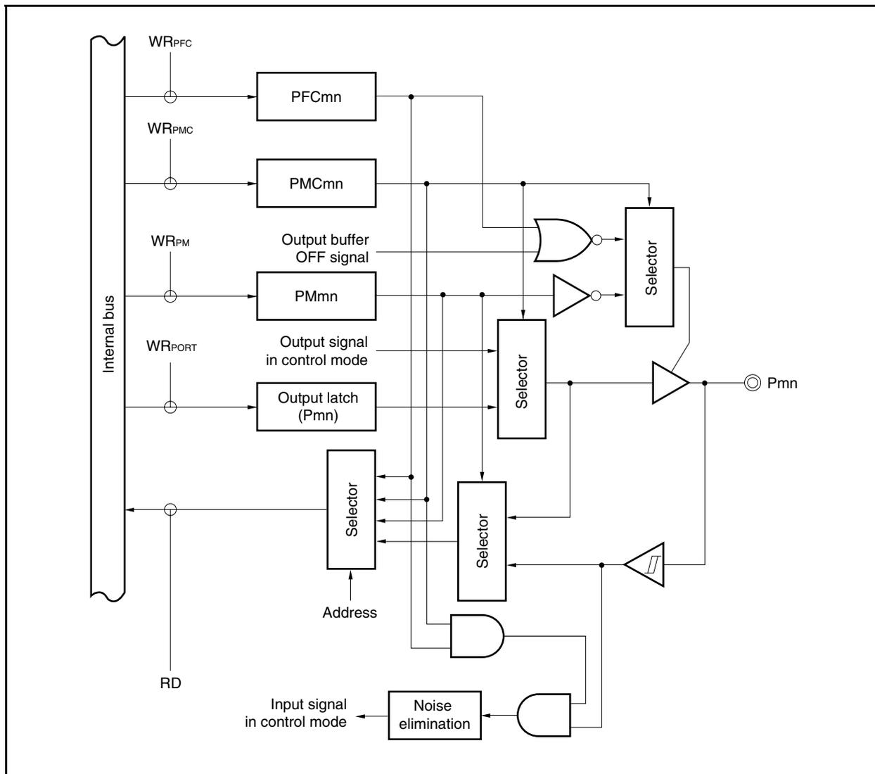
Figure 4-6. Block Diagram of Type A-5
