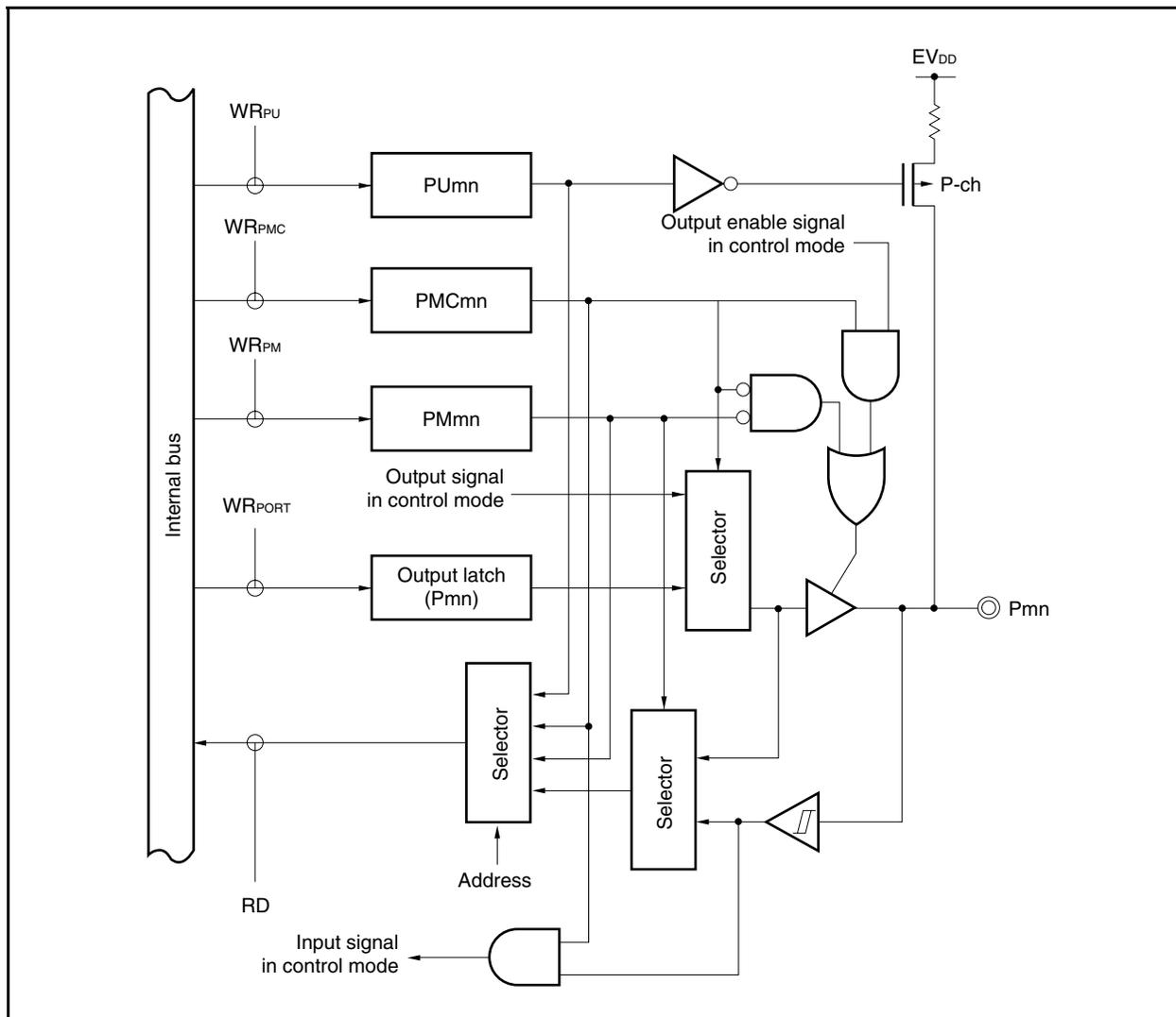
Figure 4-14. Block Diagram of Type D-1
