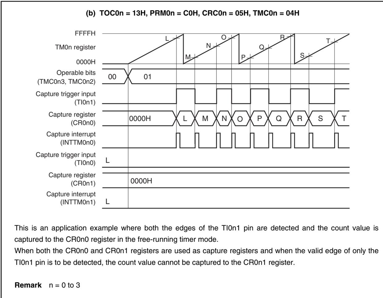
Figure 7-29. Example of Register Settings in Free-Running Timer Mode (1/2)
