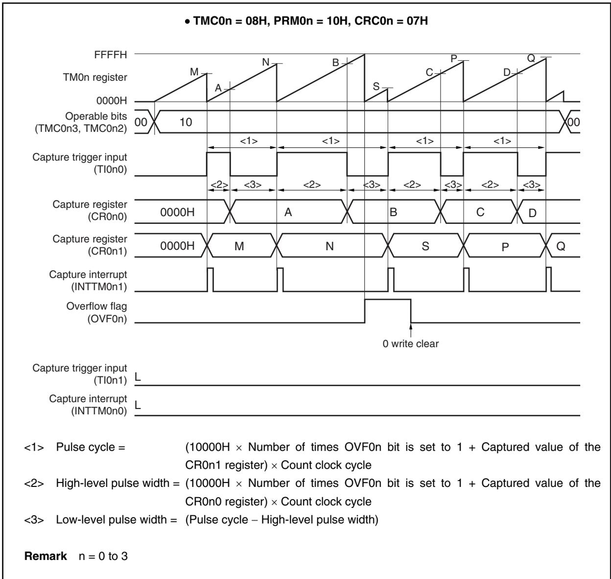
Figure 7-42. Example of Register Settings for Pulse Width Measurement (1/2)
