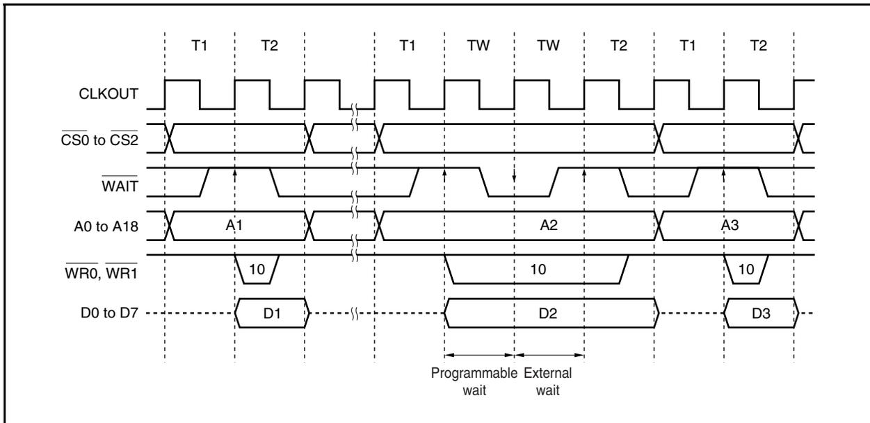
Figure 5-8. Address Wait Timing (Bus Read, Bus Size: 16 Bits, 16-Bit Access)
