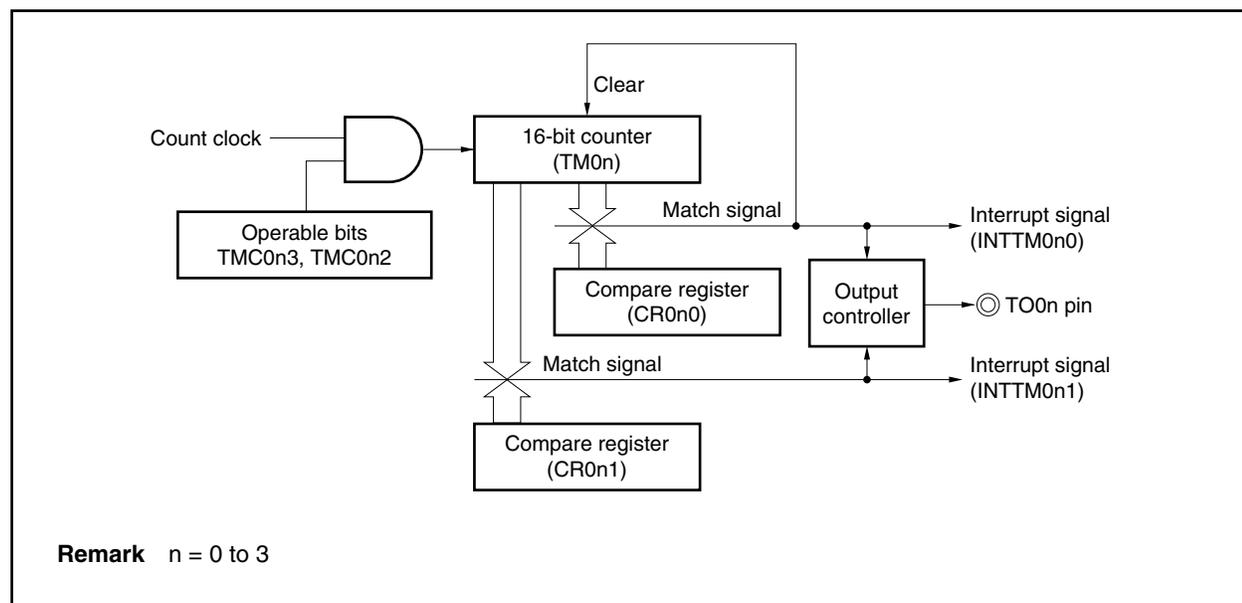
Figure 7-32. Example of Register Settings for PPG Output Operation
