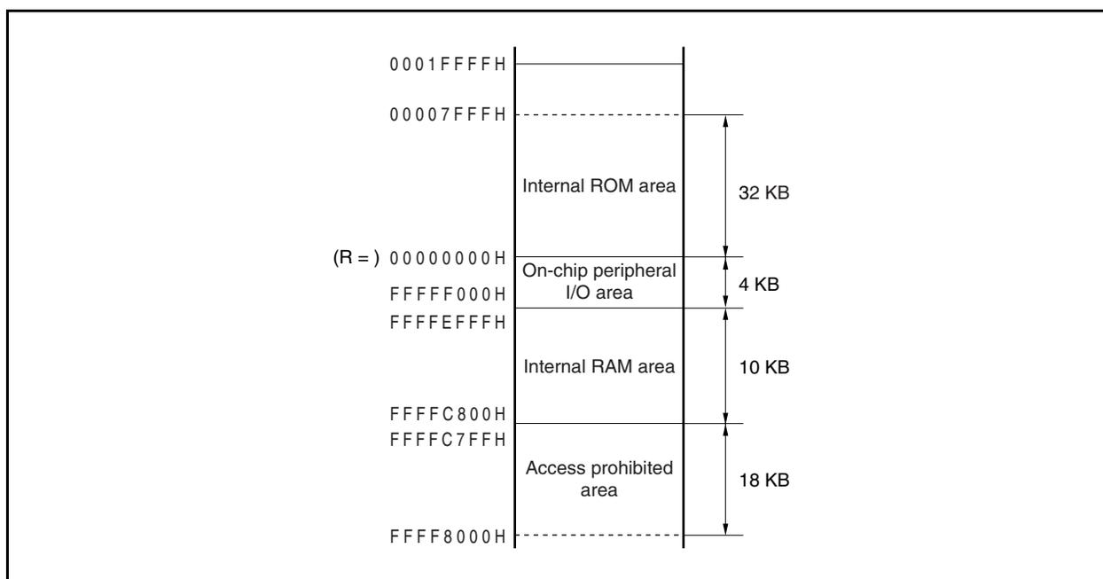
If R = r0 (zero register) is specified for the LD/ST disp16 [R] instruction, a range of addresses 00000000H  $\pm 32$  KB can be addressed by sign-extended disp16. All the resources of the internal hardware can be addressed by one pointer.
