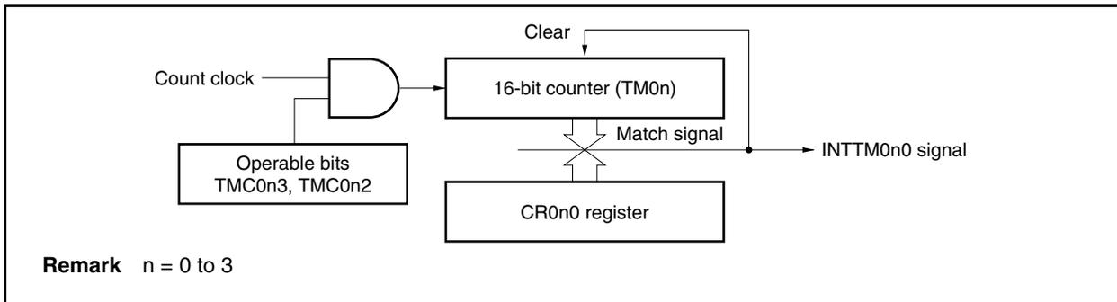
**Figure 7-3. Basic Timing Example of Interval Timer Operation**
