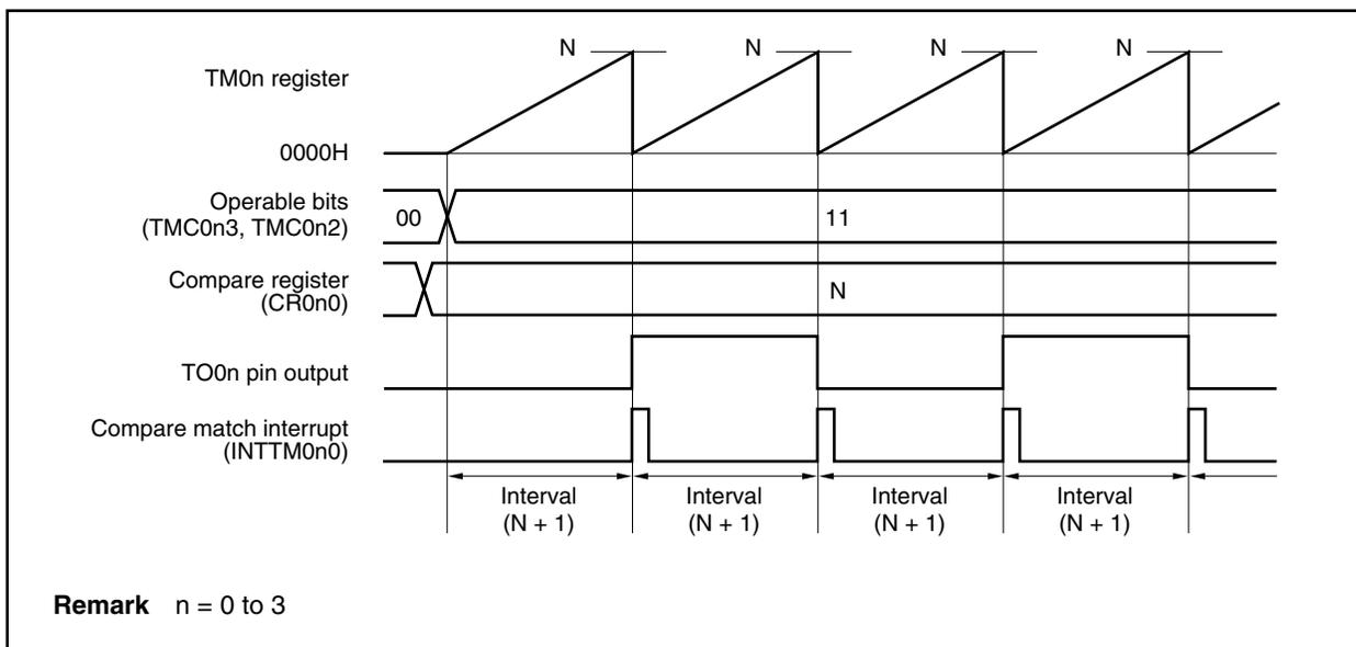
Figure 7-8. Example of Register Settings for Square Wave Output Operation
