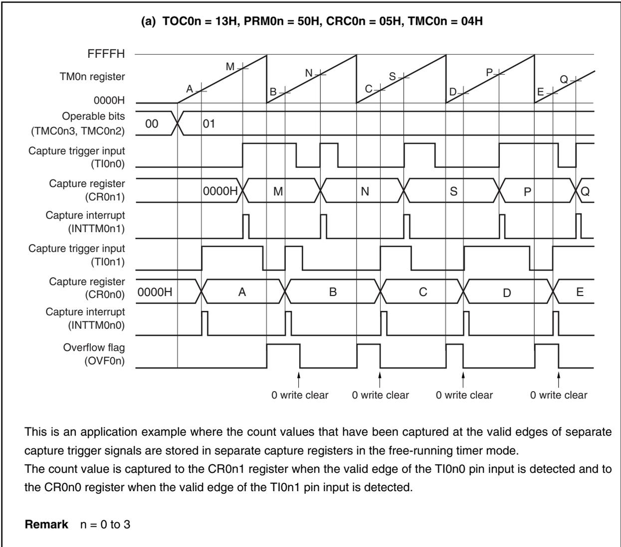
**Figure 7-28. Timing Example of Free-Running Timer Mode
