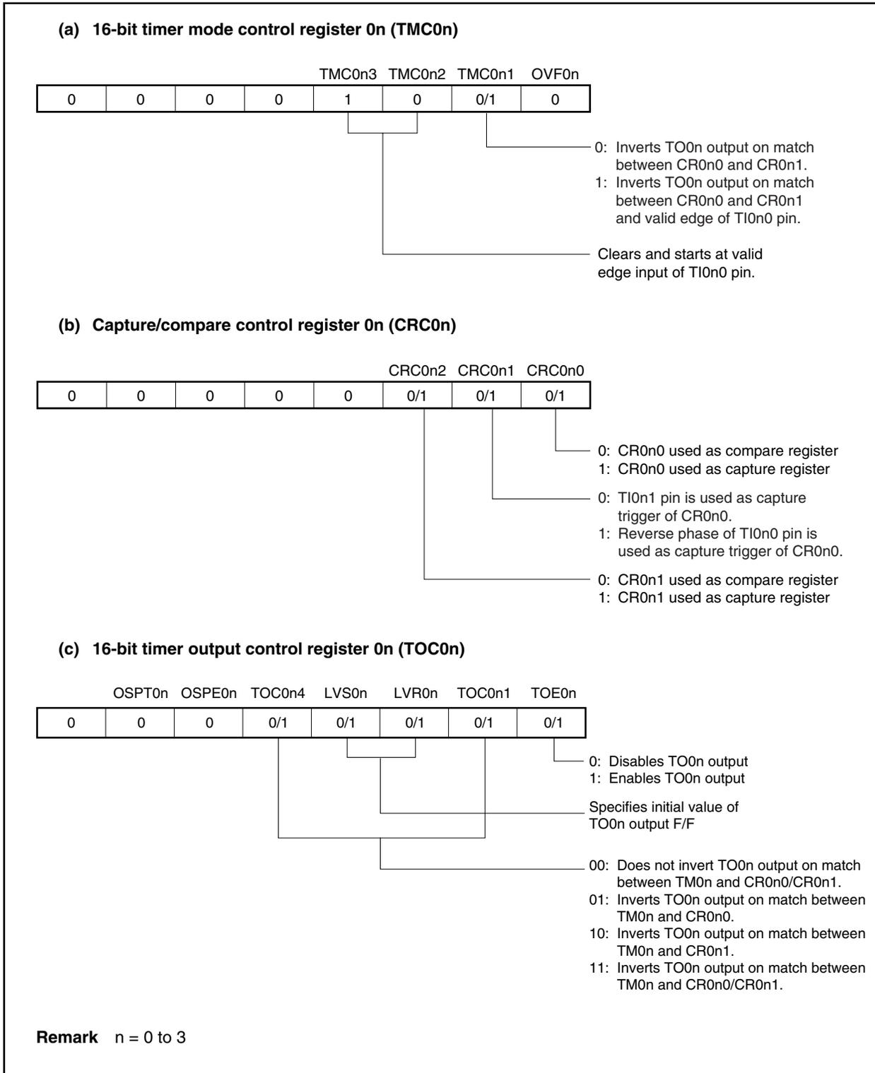
Figure 7-21. Example of Register Settings in Clear &amp; Start Mode Entered by TI0n0 Pin Valid Edge Input (2/2)
