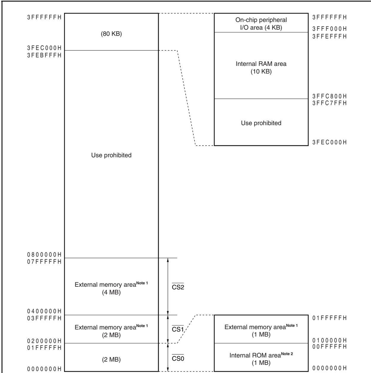
**Notes 1.** Each of these areas is a 512 KB space of 0100000H to 017FFFFH, 0200000H to 027FFFFH, or 0400000H to 047FFFFH (0180000H to 01FFFFFFH, 0280000H to 03FFFFFFH, and 0480000H to 07FFFFFFH are an image).
