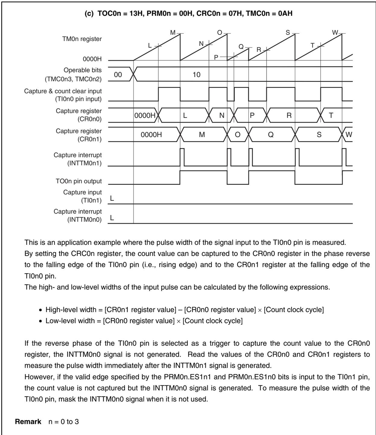
Figure 7-21. Example of Register Settings in Clear & Start Mode Entered by TI0n0 Pin Valid Edge Input (1/2)
