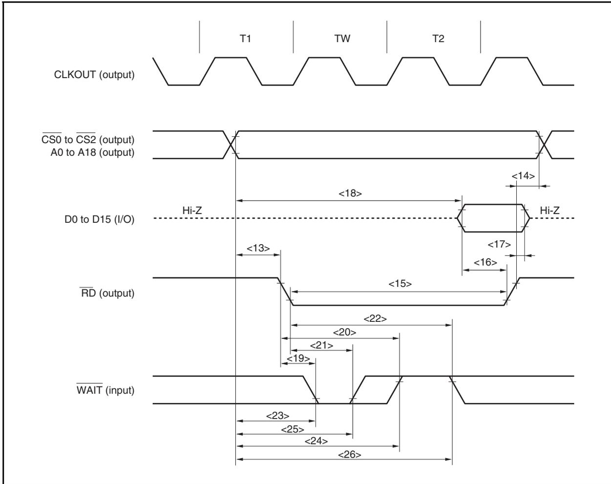
Write cycle (CLKOUT asynchronous, 1 wait)
