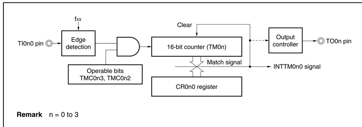
Figure 7-11. Example of Register Settings in External Event Counter Mode
