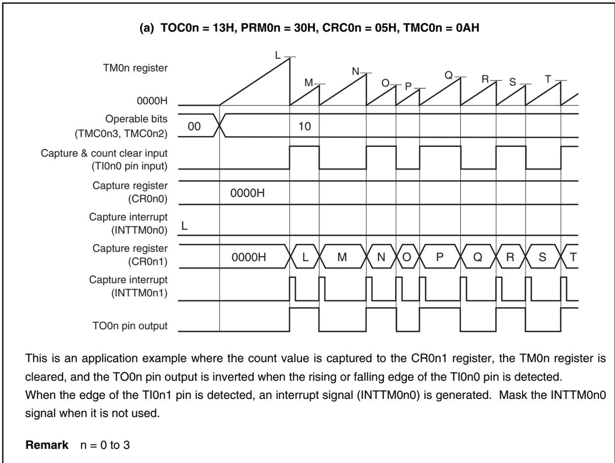
**Figure 7-20. Timing Example of Clear & Start Mode Entered by TIO<sub>n</sub>0 Pin Valid Edge Input (CR0<sub>n</sub>0 Register: Capture Register, CR0<sub>n</sub>1 Register: Capture Register) (2/3)**
