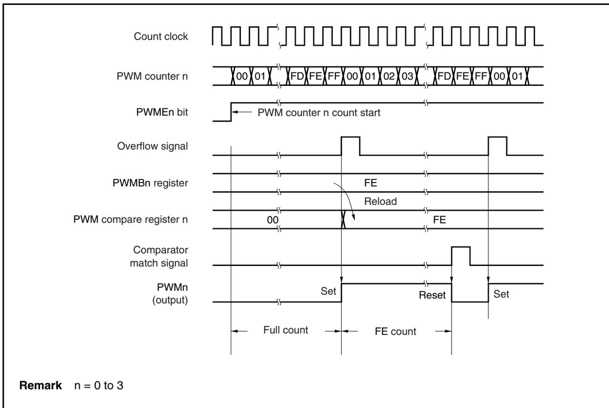
Figure 13-3. Operation Timing When PWMBn Register Is Set to 00H/FFH
