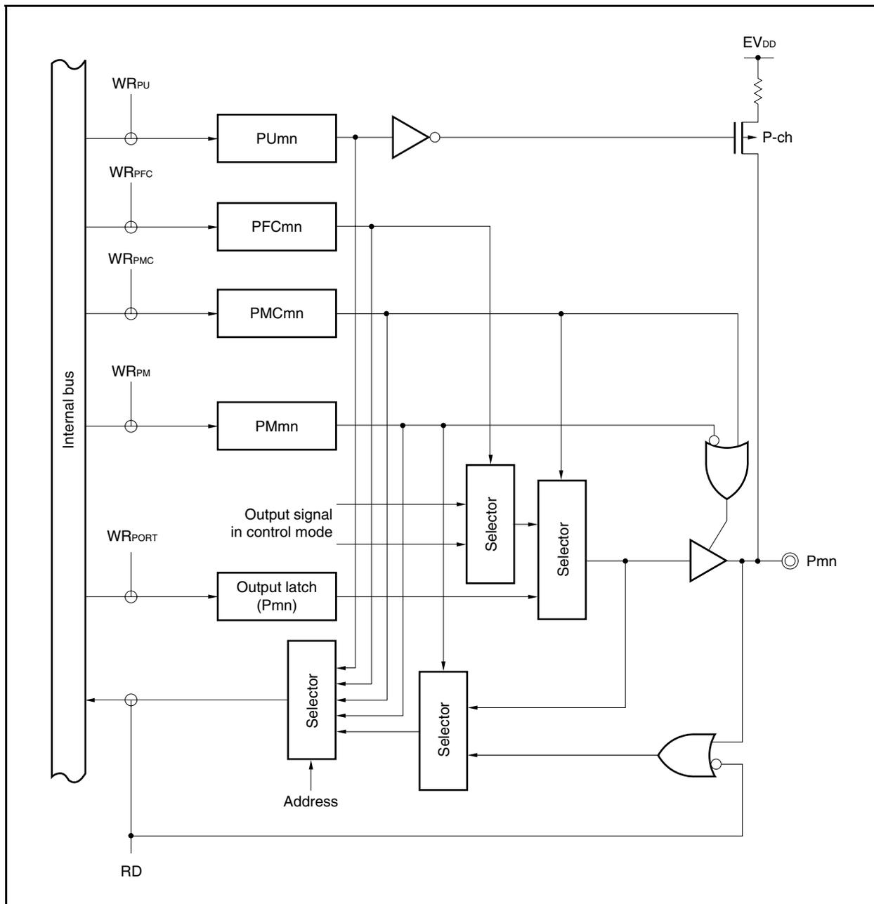
Figure 4-12. Block Diagram of Type C-1
