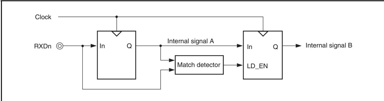
**Figure 14-11. Timing of RXDn Signal Judged as Noise**
