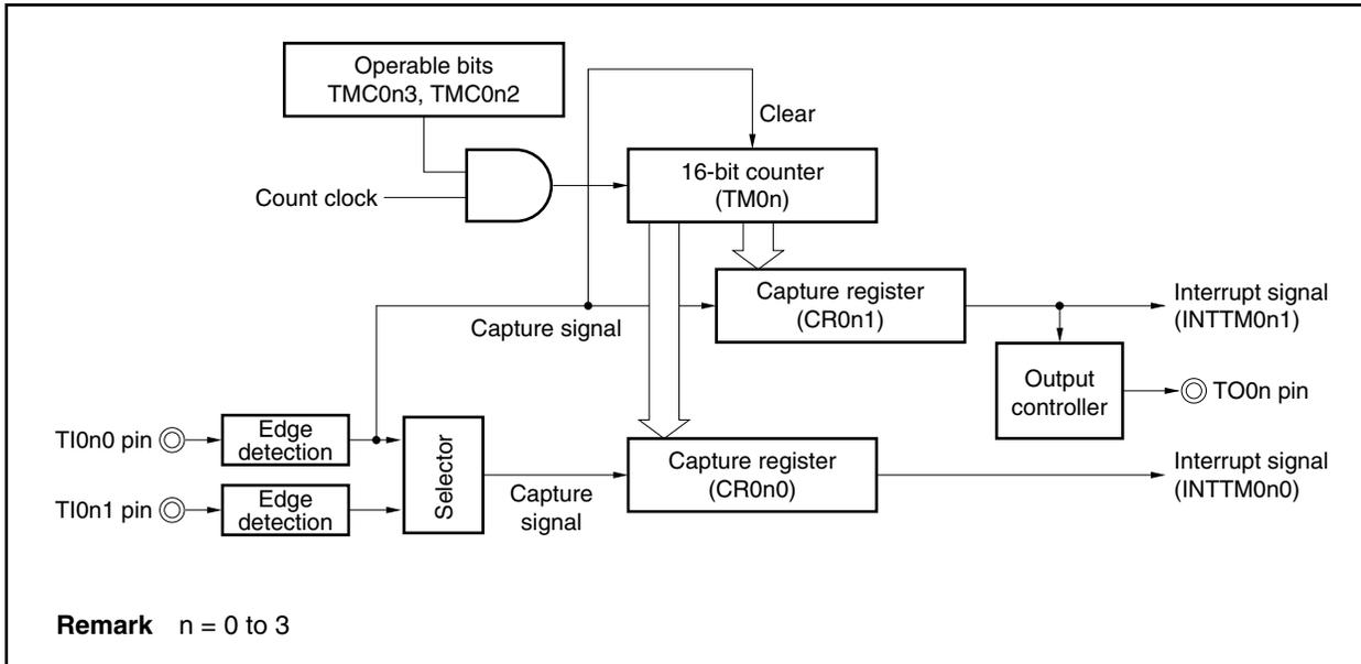
**Figure 7-20. Timing Example of Clear & Start Mode Entered by TI0n0 Pin Valid Edge Input (CR0n0 Register: Capture Register, CR0n1 Register: Capture Register) (1/3)**
