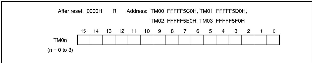
The count value of the TM0n register can be read by reading the TM0n register when the values of the TMC0n.TMC0n3 and TMC0n.TMC0n2 bits are other than 00. The value of the TM0n register is 0000H if it is read when the TMC0n3 and TMC0n2 bits are 00.
