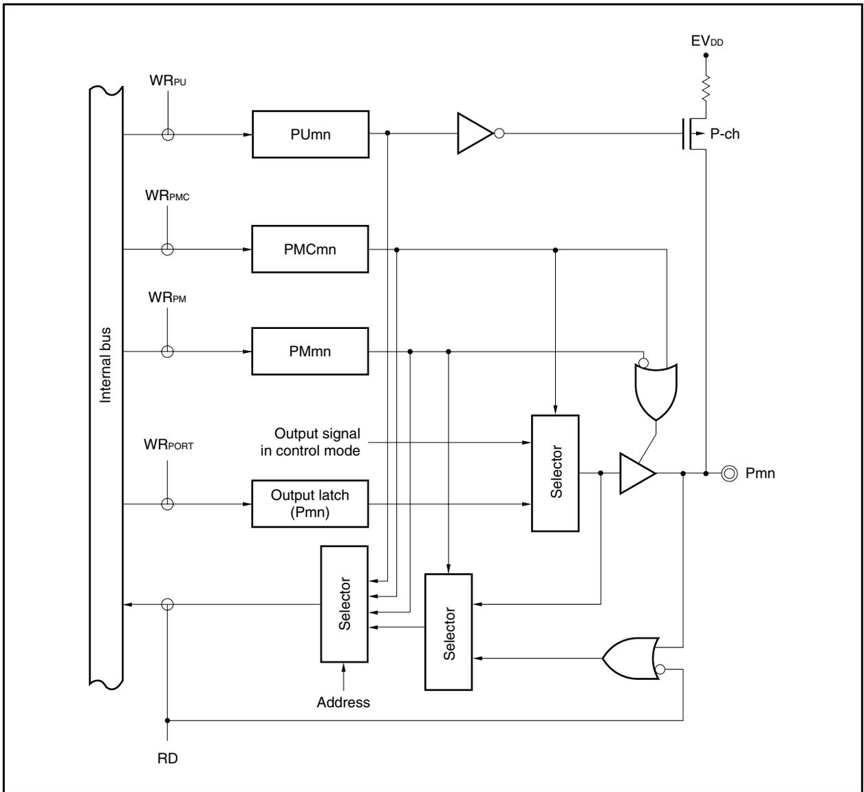
Figure 4-11. Block Diagram of Type B-4
