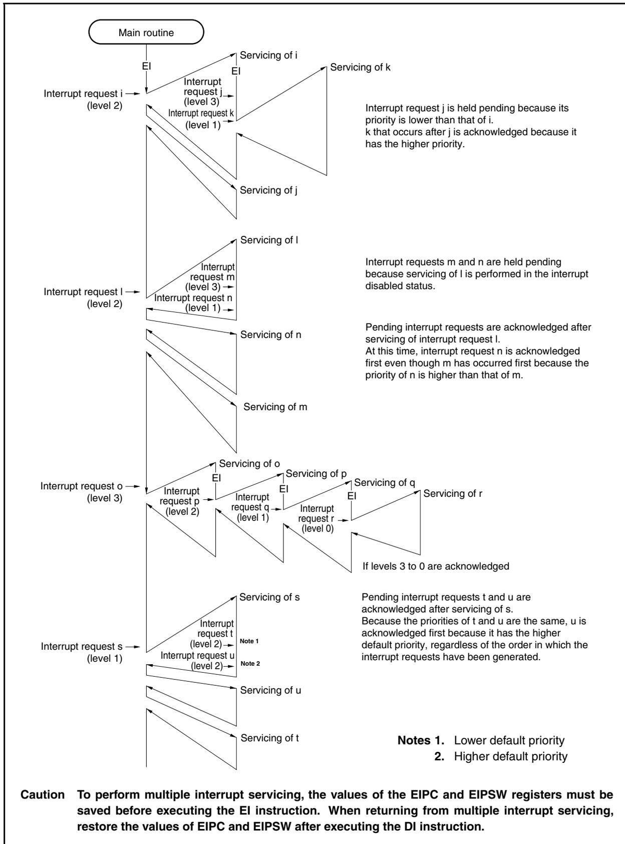
Figure 16-7. Example of Servicing Interrupt Requests Simultaneously Generated
