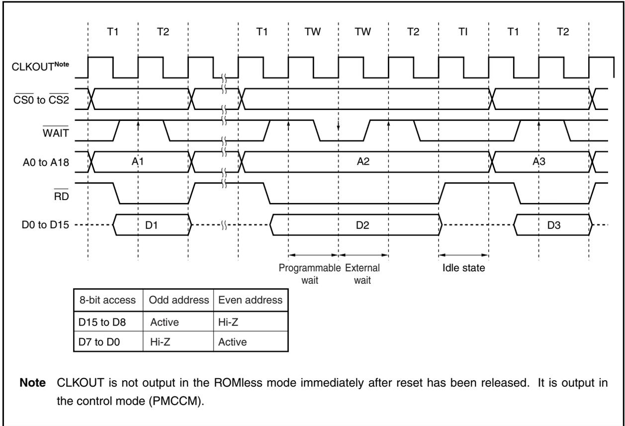
Figure 5-5. Bus Read Timing (Bus Size: 8 Bits)
