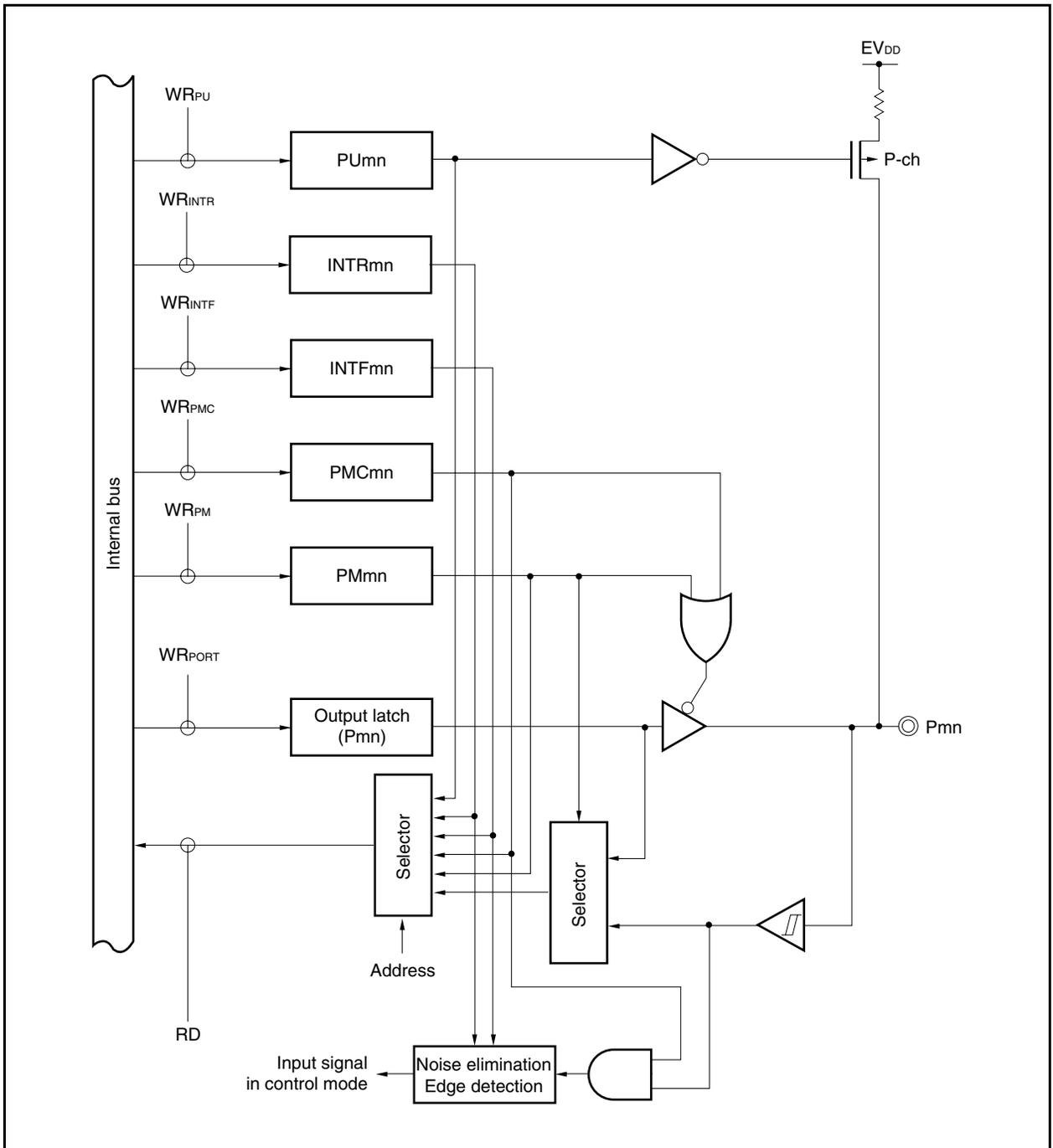
Figure 4-5. Block Diagram of Type A-4
