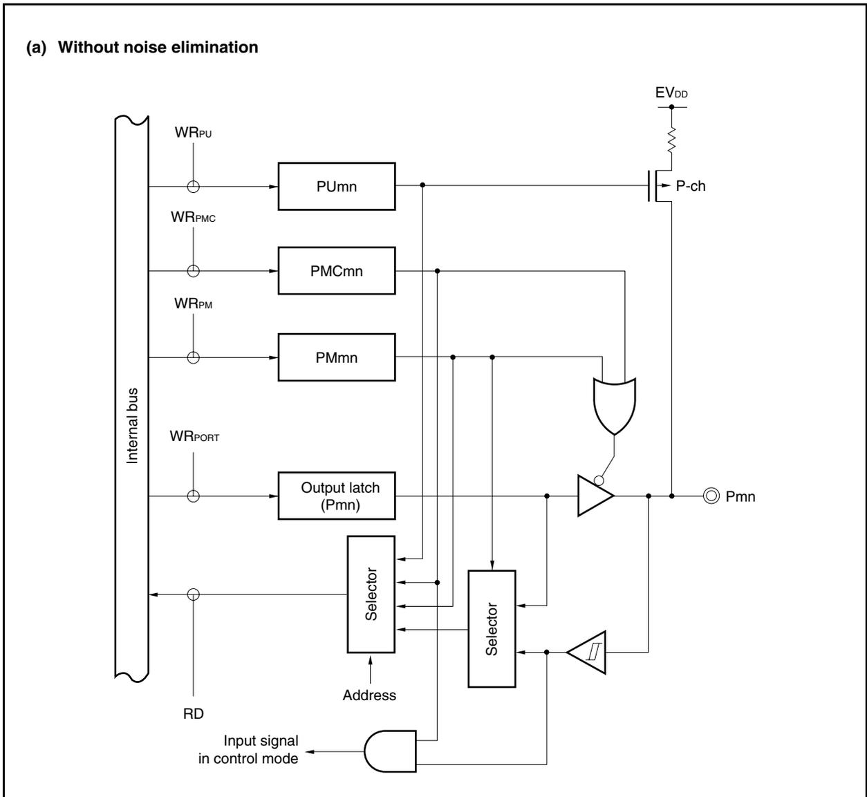
Figure 4-3. Block Diagram of Type A-2 (2/2)
