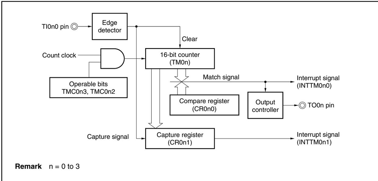
**Figure 7-16. Timing Example of Clear & Start Mode Entered by TIO<sub>n</sub>0 Pin Valid Edge Input (CR0<sub>n</sub> Register: Compare Register, CR0<sub>n</sub>1 Register: Capture Register) (1/2)**
