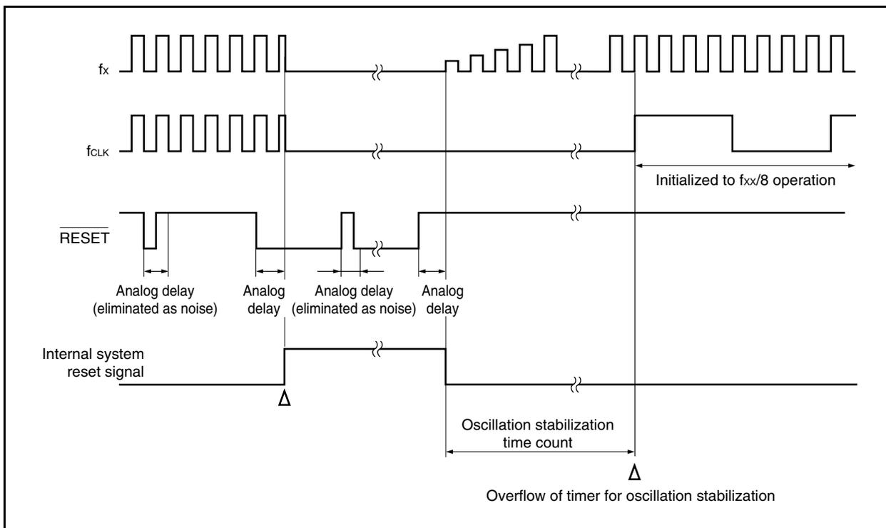
Figure 18-3. Operation on Power Application
