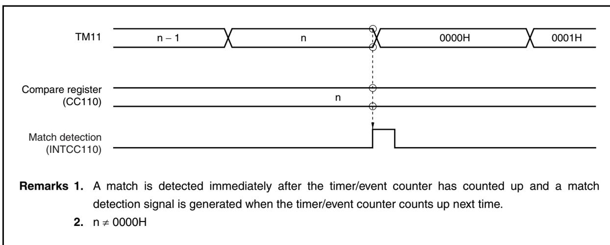
Figure 8-7. Compare Operation Example (When CCLR11 = 1 and CC110 Is 0000H)
