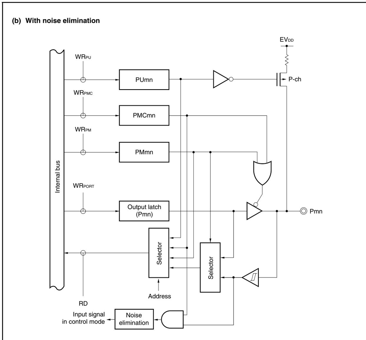
Figure 4-4. Block Diagram of Type A-3
