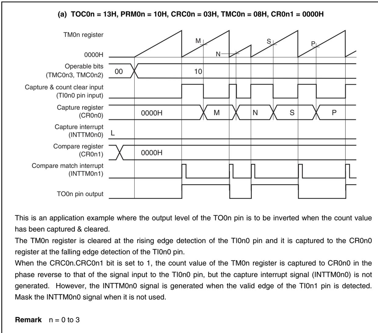
**Figure 7-18. Timing Example of Clear & Start Mode Entered by TIO<sub>n</sub> Pin Valid Edge Input (CR0<sub>n</sub> Register: Capture Register, CR0<sub>n</sub> Register: Compare Register) (2/2)**
