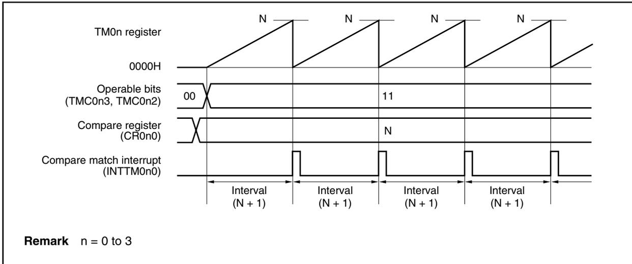
Figure 7-4. Example of Register Settings for Interval Timer Operation
