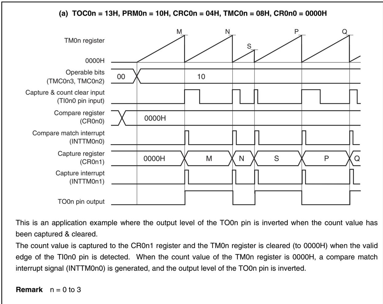
**Figure 7-16. Timing Example of Clear & Start Mode Entered by TIO<sub>n</sub> Pin Valid Edge Input
