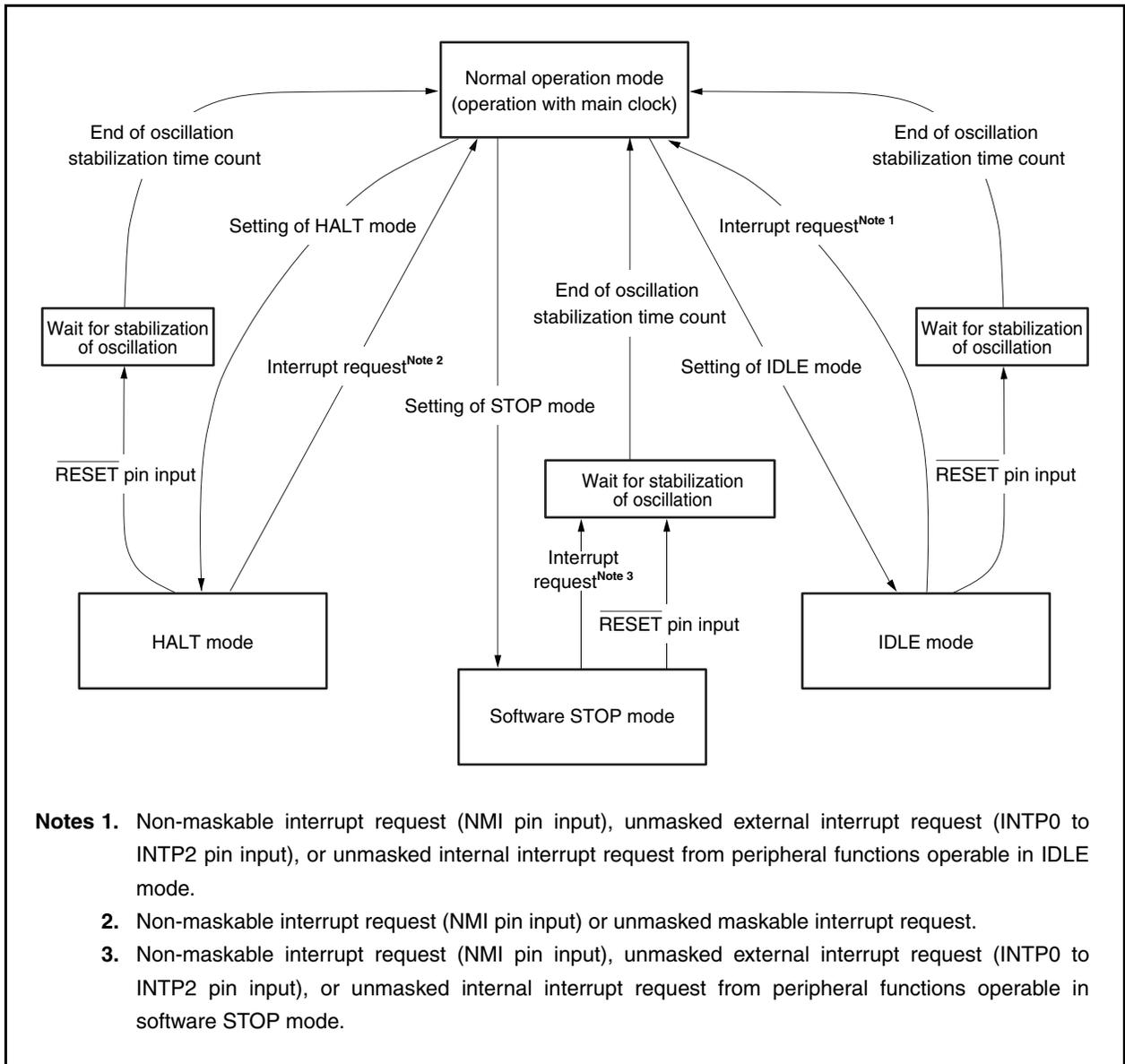
Figure 17-2. Status Transition (During Subclock Operation)
