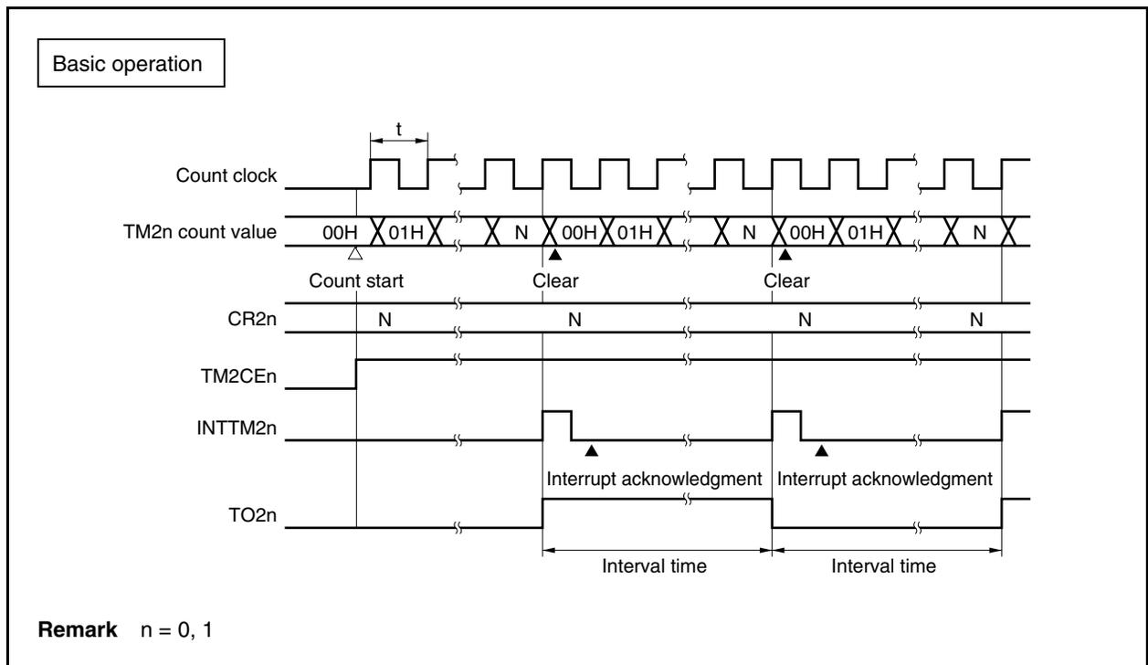
Figure 9-2. Timing of Interval Timer Operation (2/2)
