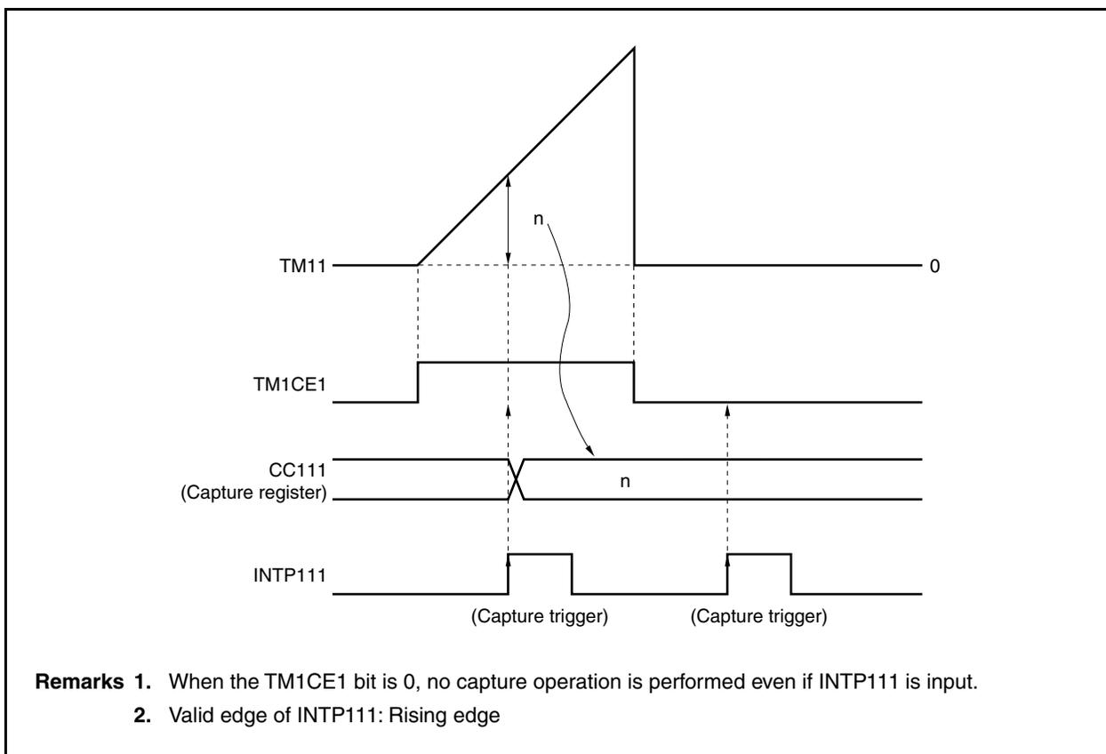
Figure 8-5. TM11 Capture Operation Example (When Both Edges Are Specified)
