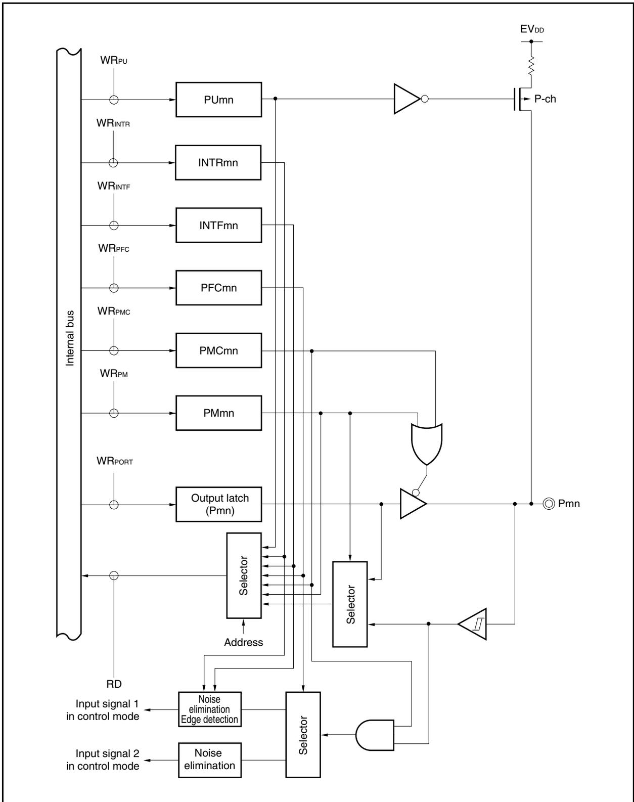
Figure 4-7. Block Diagram of Type A-6
