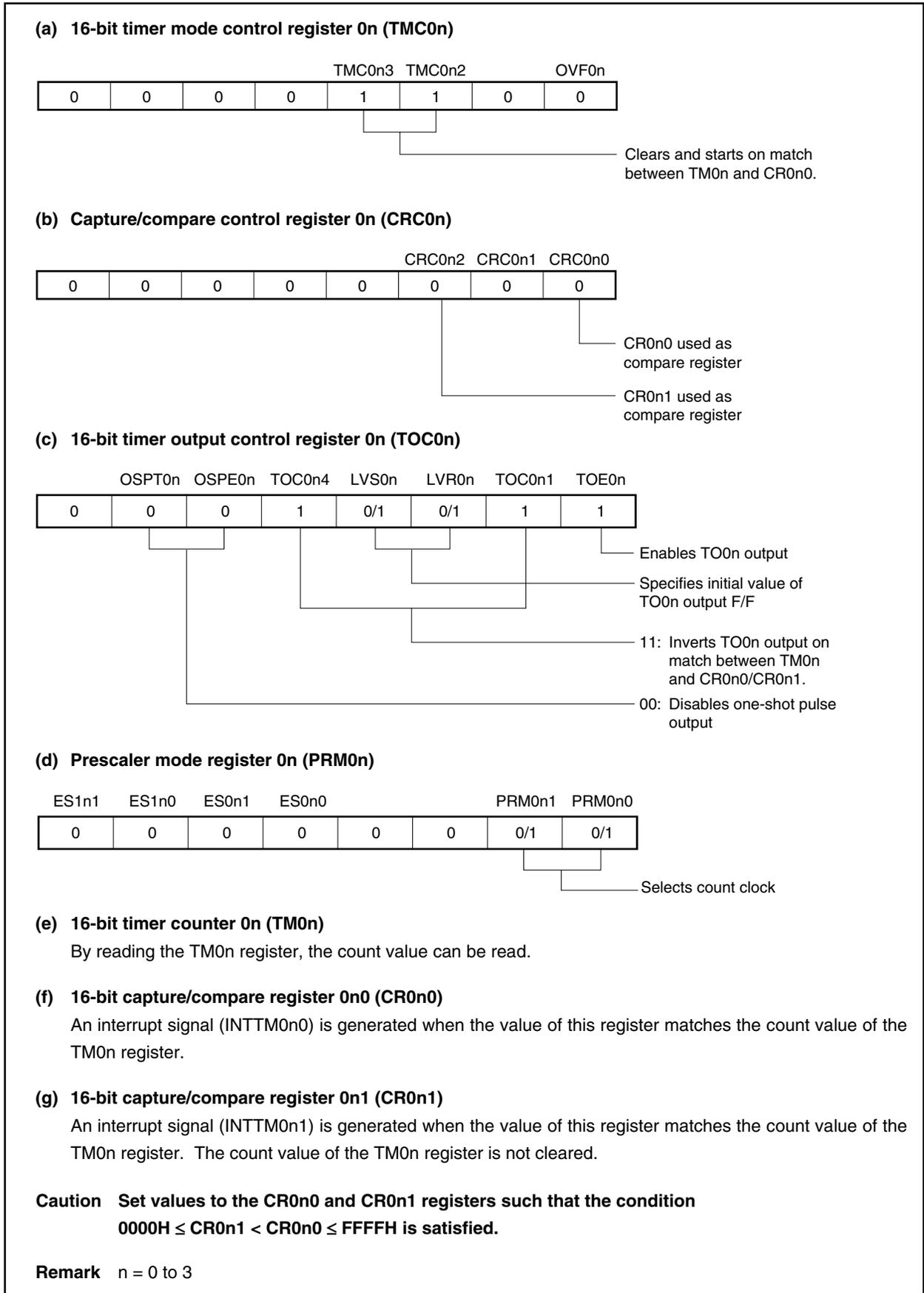
Figure 7-33. Example of Software Processing for PPG Output Operation
