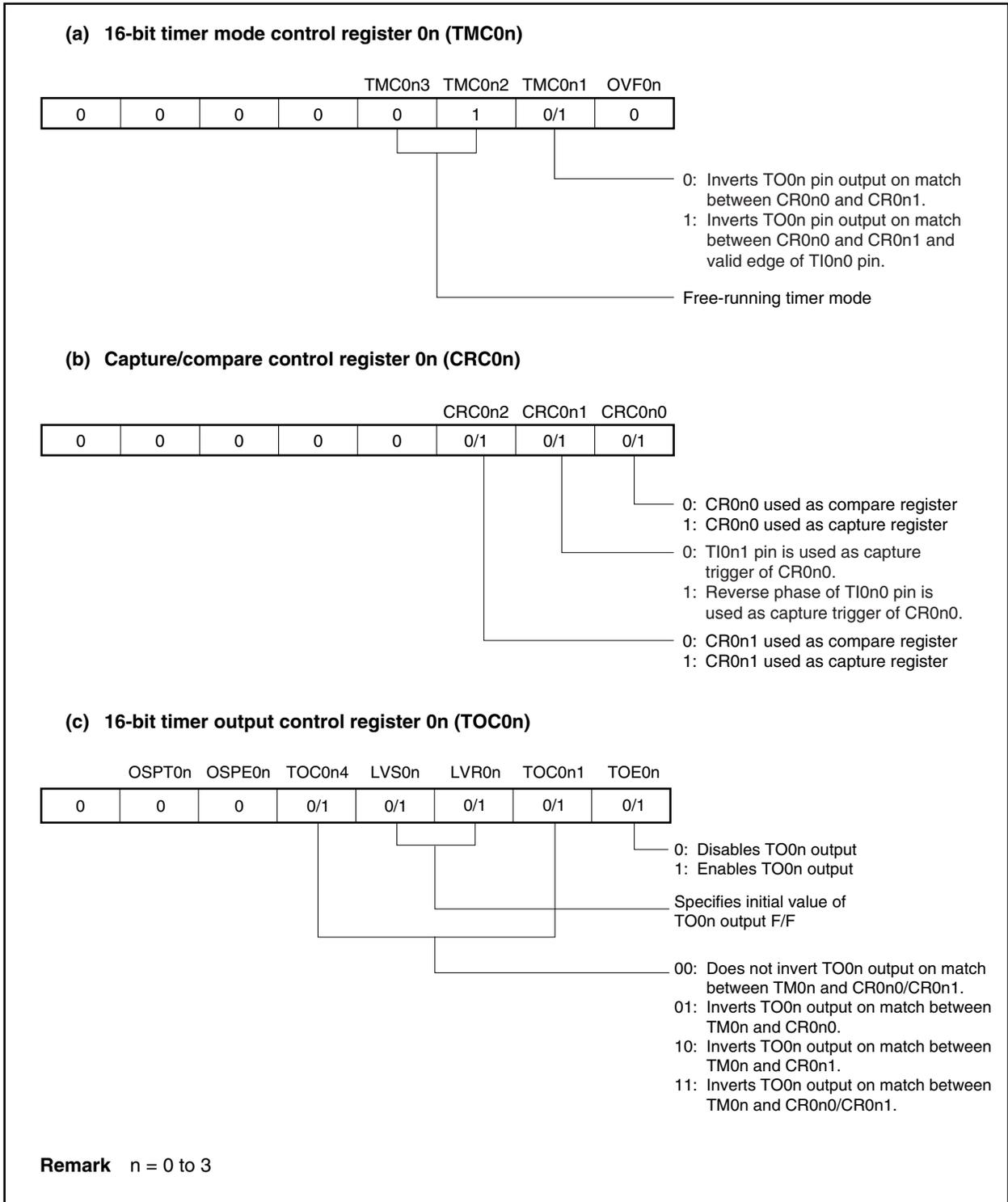
Figure 7-29. Example of Register Settings in Free-Running Timer Mode (2/2)
