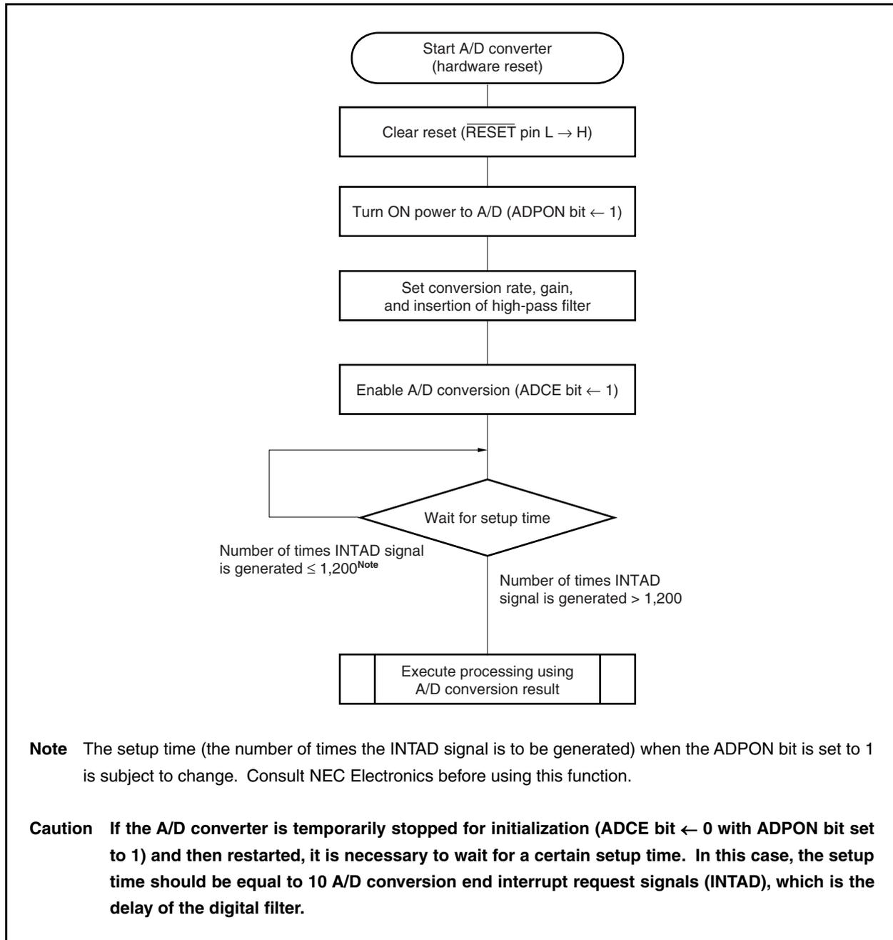
When A/D conversion is enabled, conversion of the signals on the six channels of analog input pins (ANIn0 and ANIn1 pins) is started. Two sets of 3-multiplex  $\Delta\Sigma$  circuits are provided, each of which executes conversion of three channels by time division. Each time conversion of all the six channels is completed, the INTAD signal is generated to inform the CPU that the conversion result can be read.
