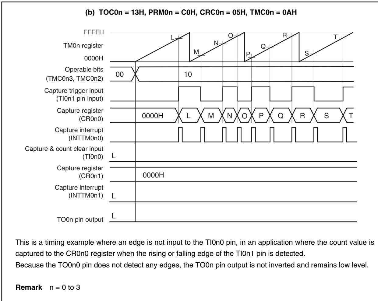
**Figure 7-20. Timing Example of Clear & Start Mode Entered by TI0n0 Pin Valid Edge Input (CR0n0 Register: Capture Register, CR0n1 Register: Capture Register) (3/3)**
