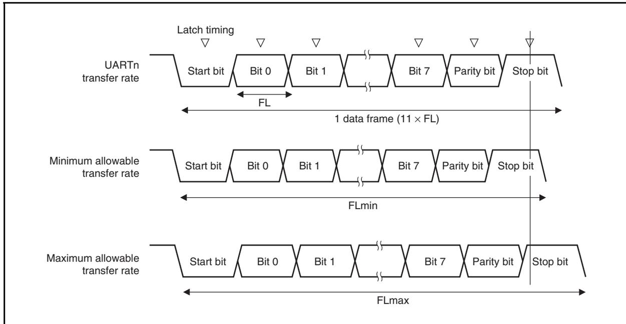
As shown in Figure 14-13, after the start bit is detected, the receive data latch timing is determined according to the counter that was set by the BRGCn register. If all data up to the final data (stop bit) is in time for this latch timing, the data can be received normally.
