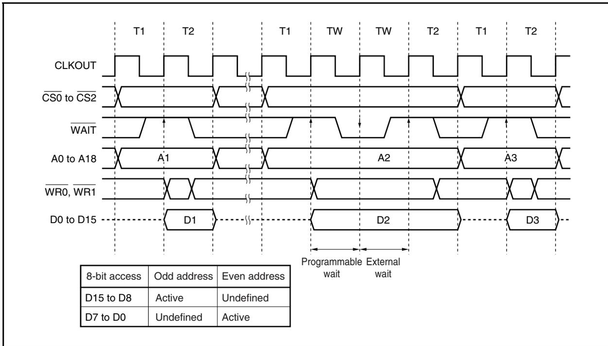
Figure 5-7. Bus Write Timing (Bus Size: 8 Bits)
