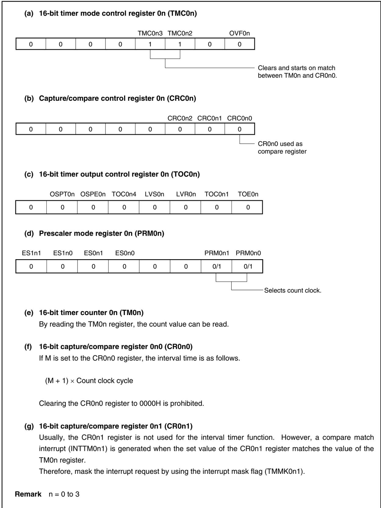
Figure 7-5. Example of Software Processing for Interval Timer Function
