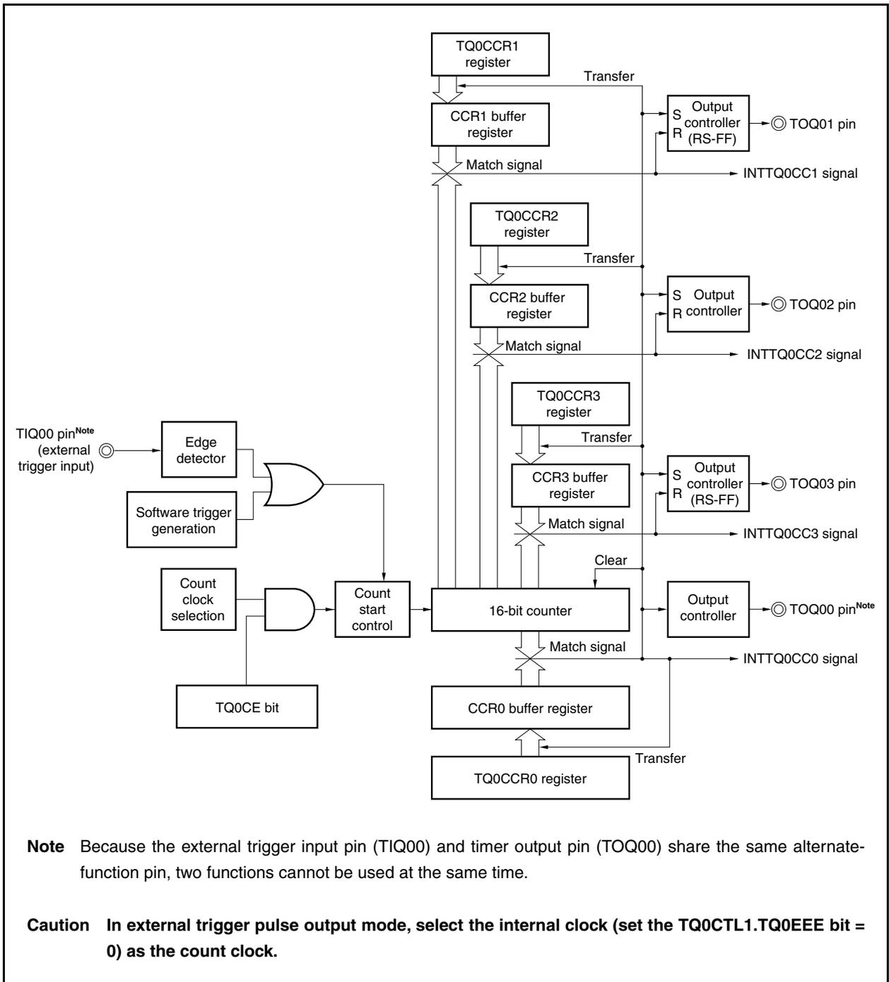
Figure 8-21. Basic Timing in External Trigger Pulse Output Mode
