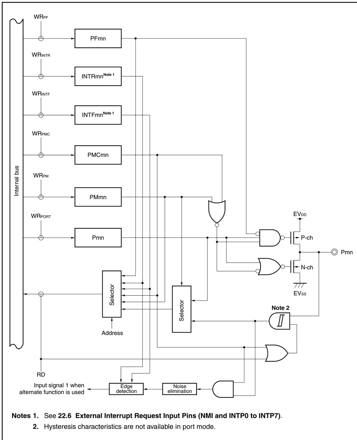
Figure 4-21. Block Diagram of Type L-2
