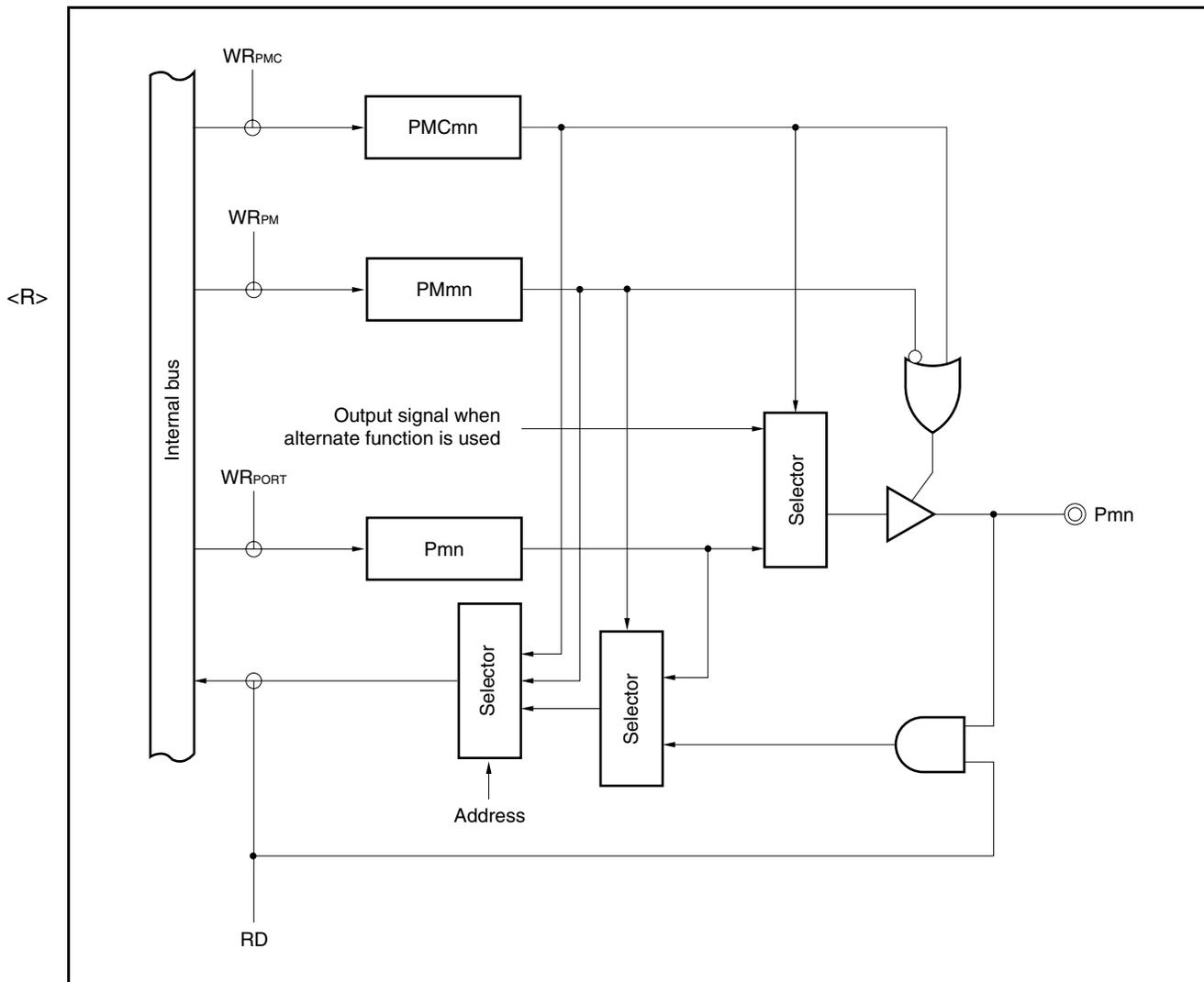
Figure 4-9. Block Diagram of Type D-3
