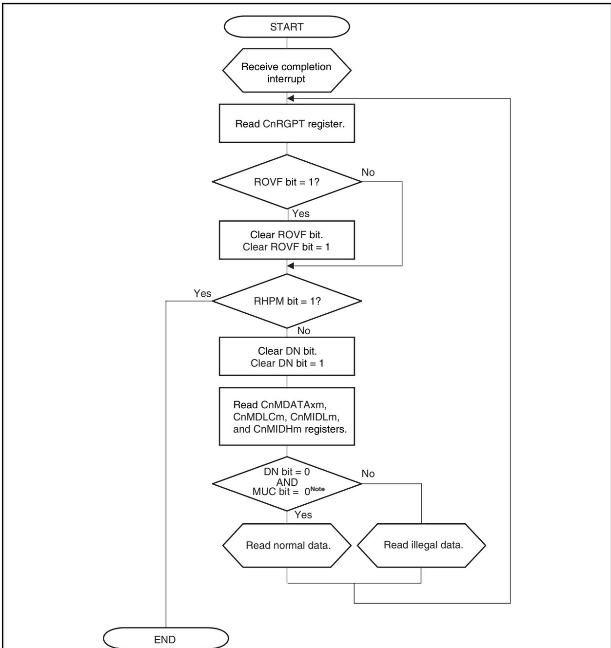
**Note** Check the MUC and DN bits using one read access.
