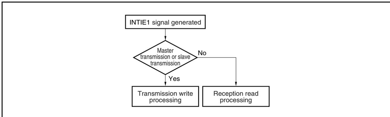
Figure 18-25. Example of Identifying INTIE2 Signal Interrupt (When INTIE1 and INTIE2 Signals Are Used)
