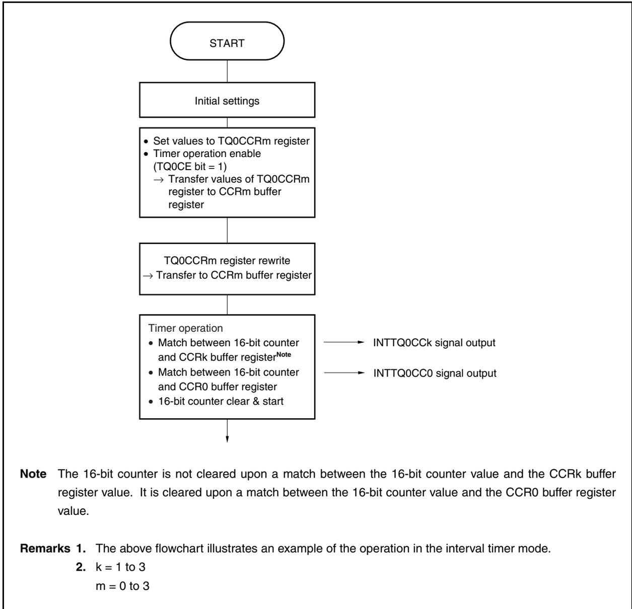
Figure 8-3. Timing of Anytime Write
