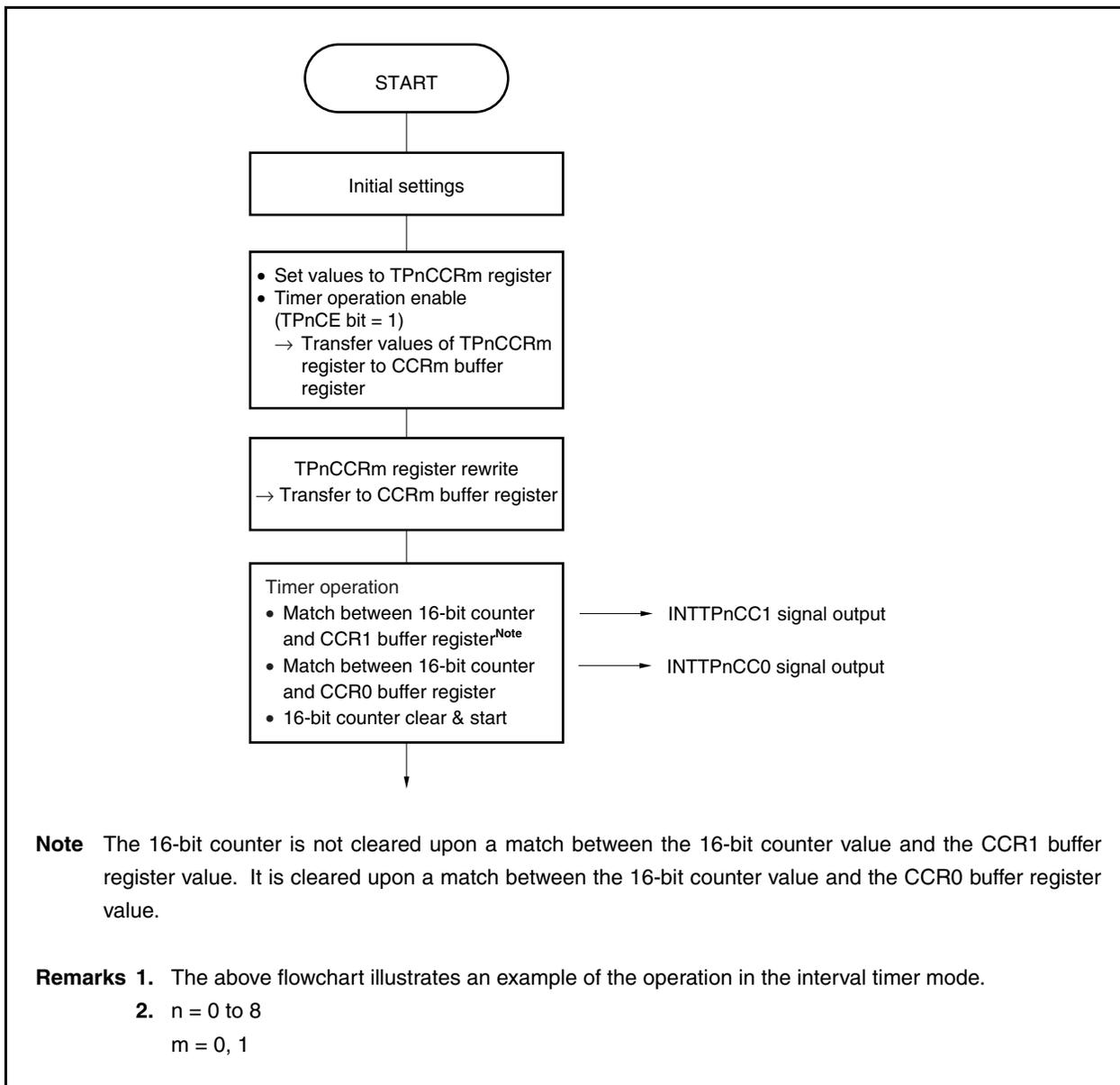
Figure 7-3. Timing of Anytime Write
