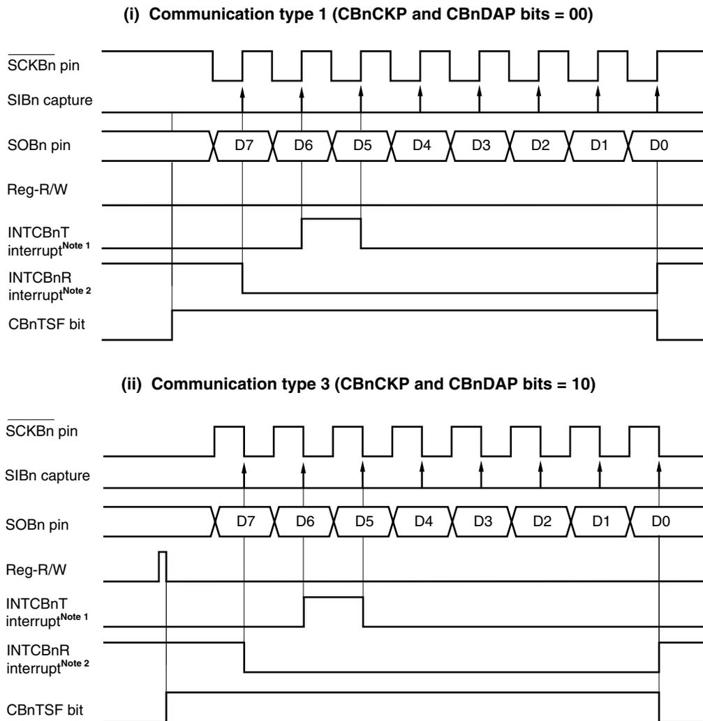
**Notes 1.** The INTCBnT interrupt is set when the data written to the CBnTX register is transferred to the data shift register in the continuous transmission or continuous transmission/reception mode. In the single transmission or single transmission/reception mode, the INTCBnT interrupt request signal is not generated, but the INTCBnR interrupt request signal is generated upon end of communication.
