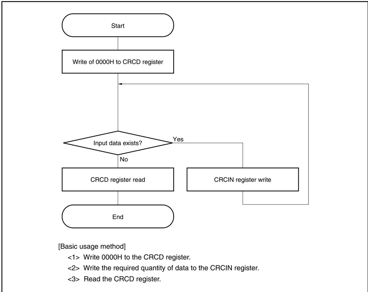
Communication errors can easily be detected if the CRC code is transmitted/received along with transmit/receive data when transmitting/receiving data consisting of several bytes.
