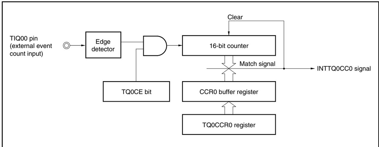
Figure 8-14. Basic Timing in External Event Count Mode
