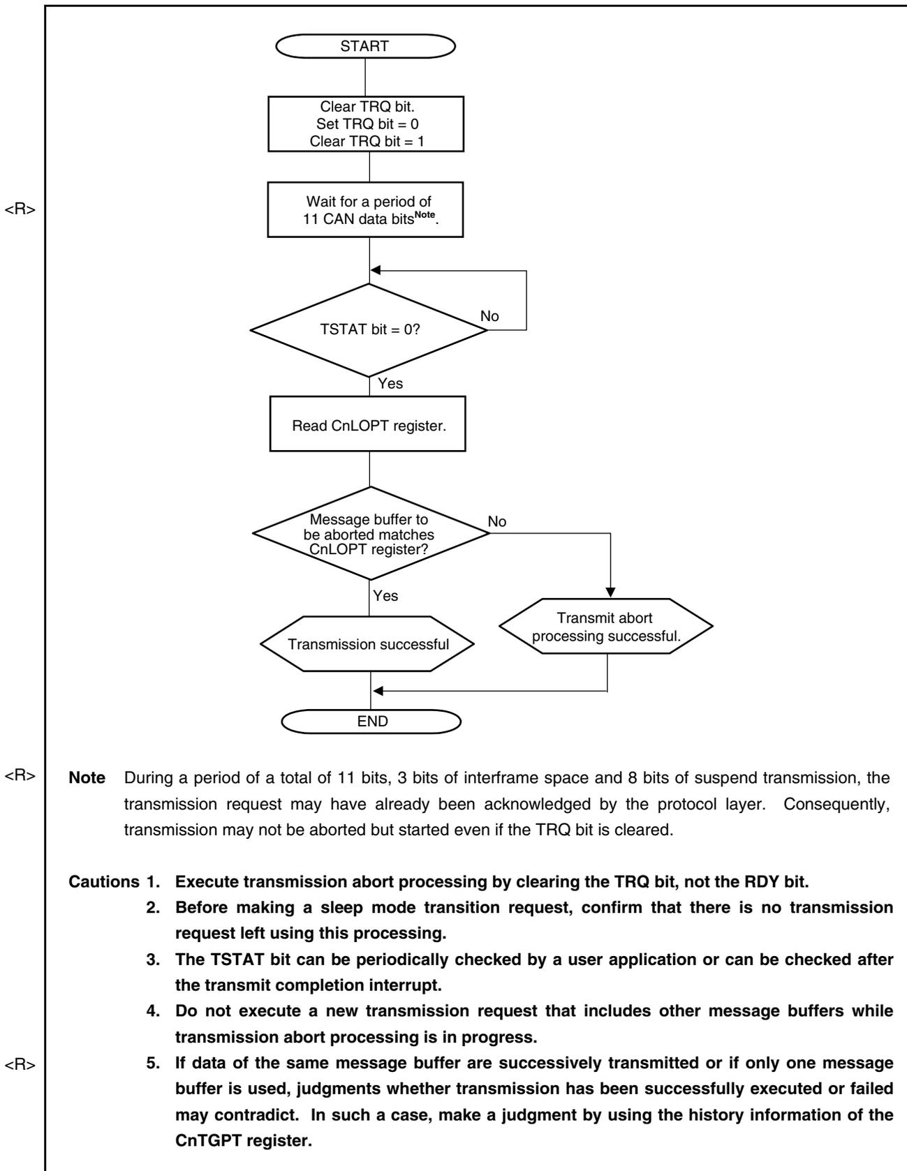
Figure 19-47. Transmission Abort Processing Except for ABT Transmission
