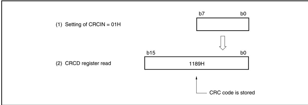
The code when 01H is sent LSB first is (1000 0000). Therefore, the CRC code from generation polynomial  $X^{16} + X^{12} + X^5 + 1$  becomes the remainder when  $(1000\ 0000) X^{16}$  is divided by  $(1\ 0001\ 0000\ 0010\ 0001)$  using the modulo-2 operation formula.
