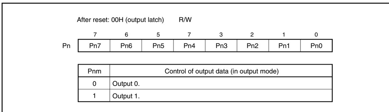
Data is written to or read from the Pn register as follows, regardless of the setting of the PMCn register.
