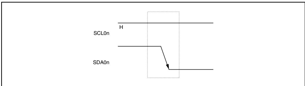
A start condition is generated when the IICn.STTn bit is set (1) after a stop condition has been detected (IICn.SPdn bit = 1). When a start condition is detected, the IICn.STDn bit is set (1) ( $n = 0$  to 2).
