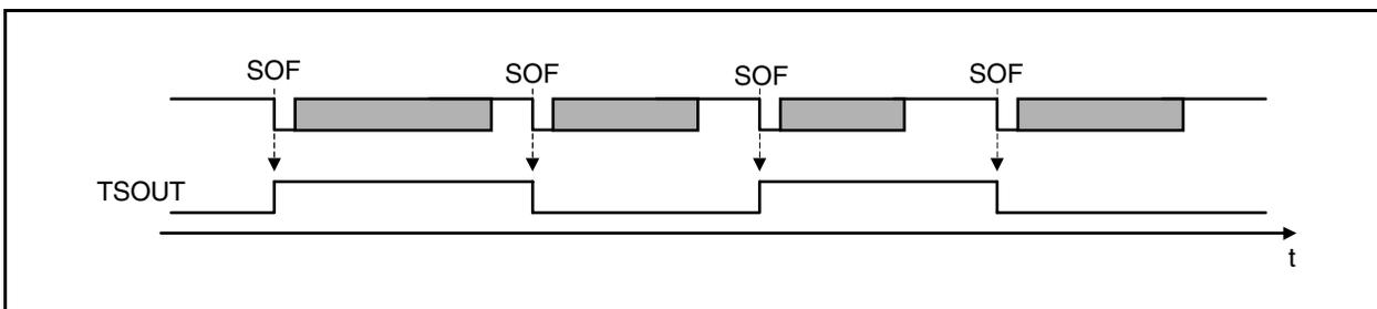
The TSOUT signal toggles its level upon occurrence of the selected event during data frame reception (in Figure 19-34, the SOF is used as the trigger event source). To capture a timer value by using the TSOUT signal, the capture timer unit must detect the capture signal at both the rising edge and falling edge.
