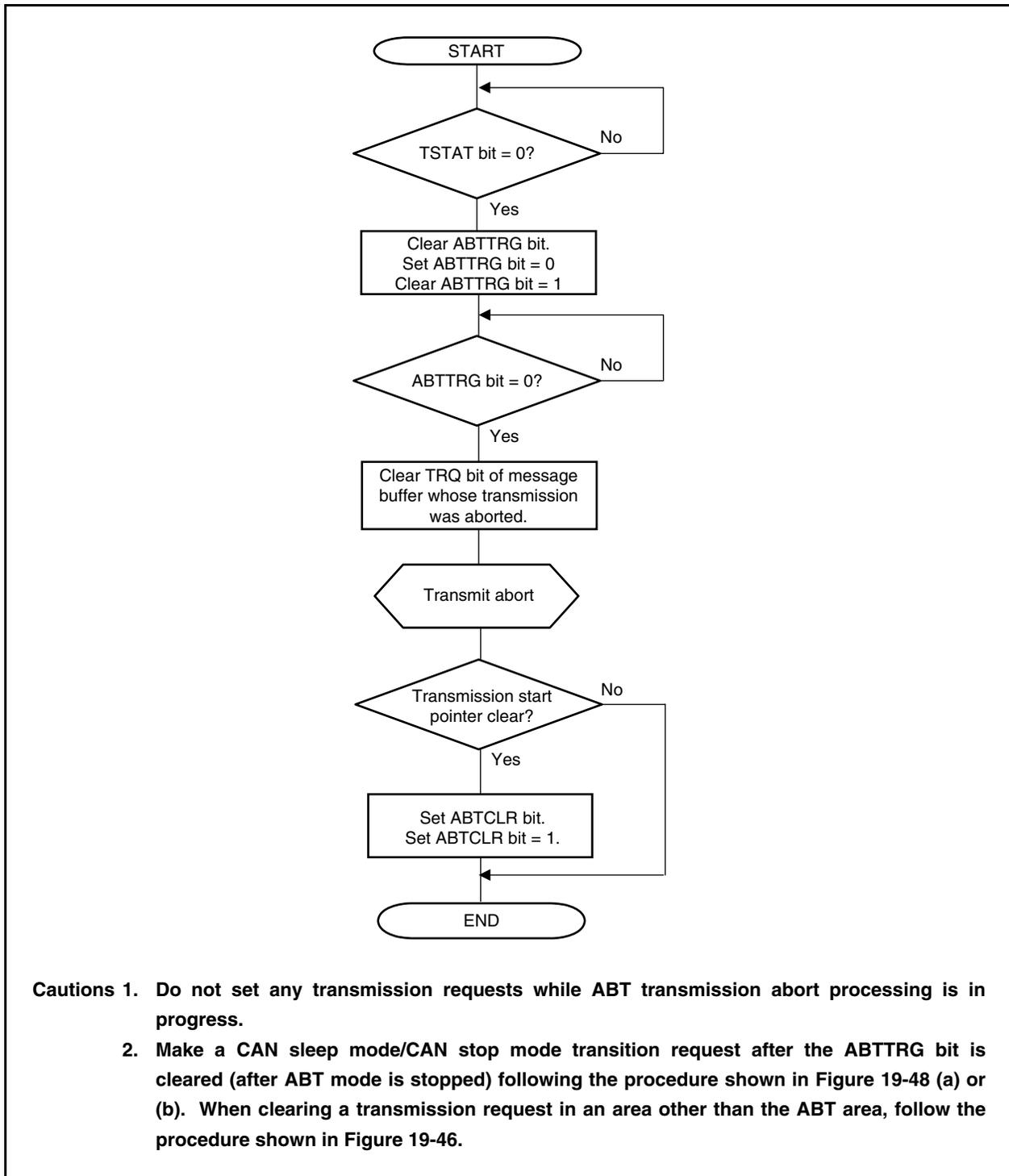
Figure 19-48 (b) shows the processing that does not skip resuming the transmission of a message that was interrupted when the transmission of an ABT message buffer was aborted.
