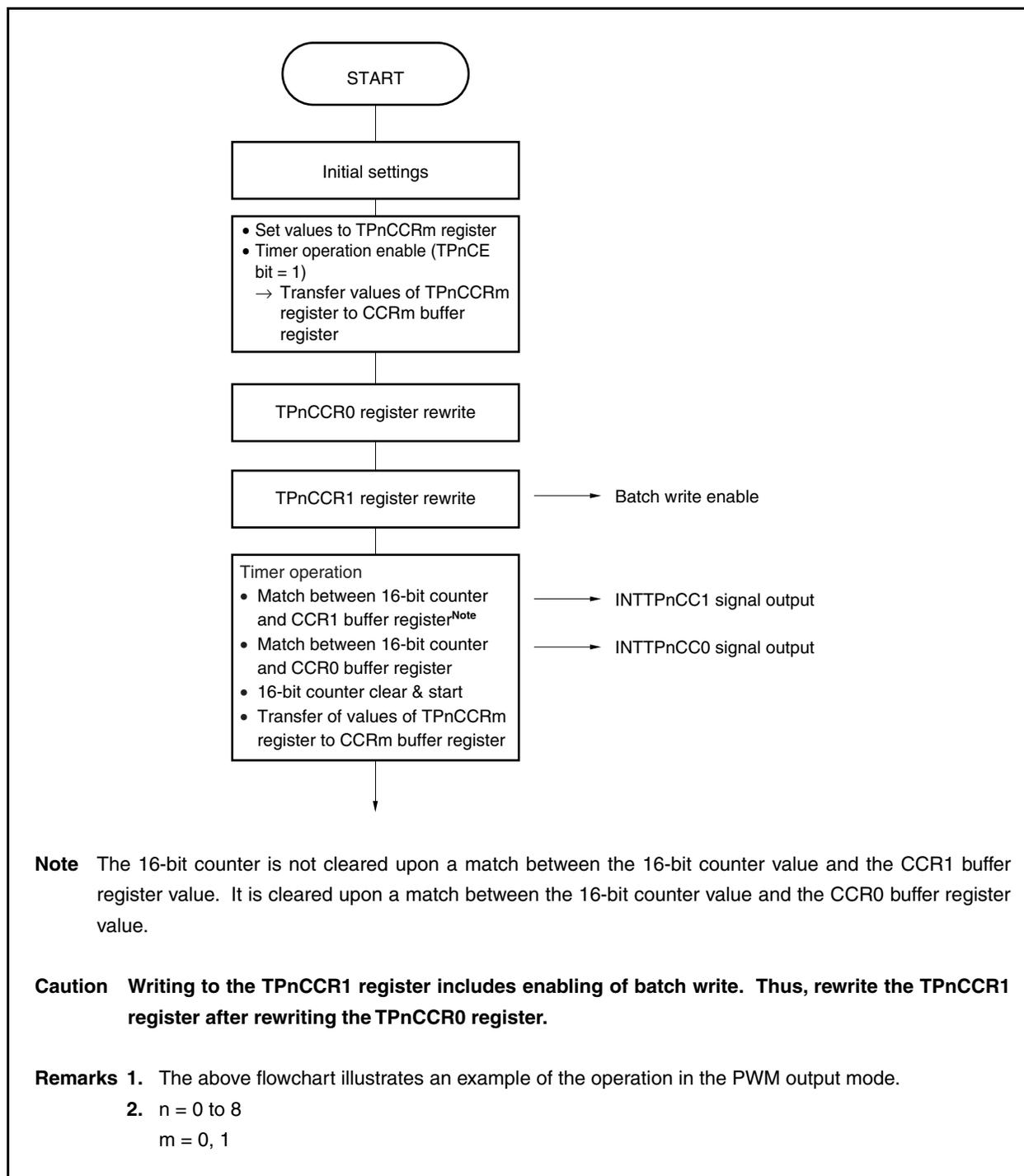
Figure 7-5. Timing of Batch Write
