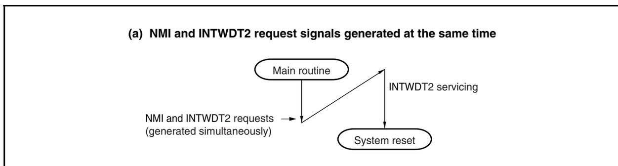
Figure 22-1. Non-Maskable Interrupt Request Signal Acknowledgment Operation (2/2)
