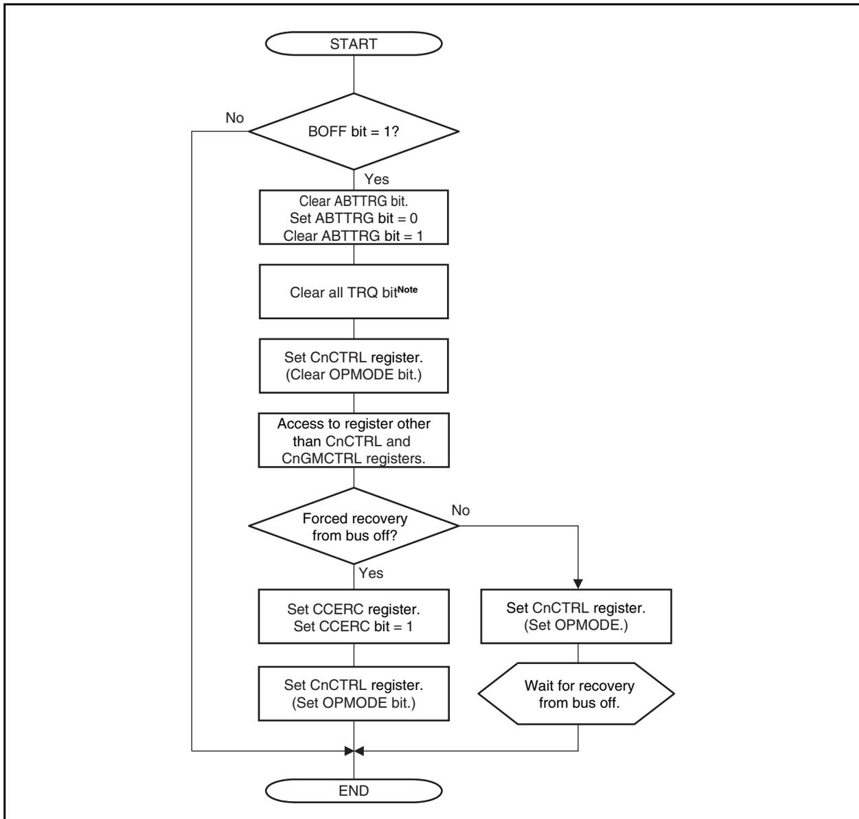
**Note** To initialize the message buffer by clearing the RDY bit before starting the bus-off recovery sequence, clear all the TRQ bits.
