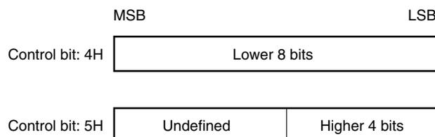
If the control bit received from the master unit is not as shown in Table 18-3, the unit locked by the master unit rejects acknowledging the control bit, and outputs the NACK signal.
