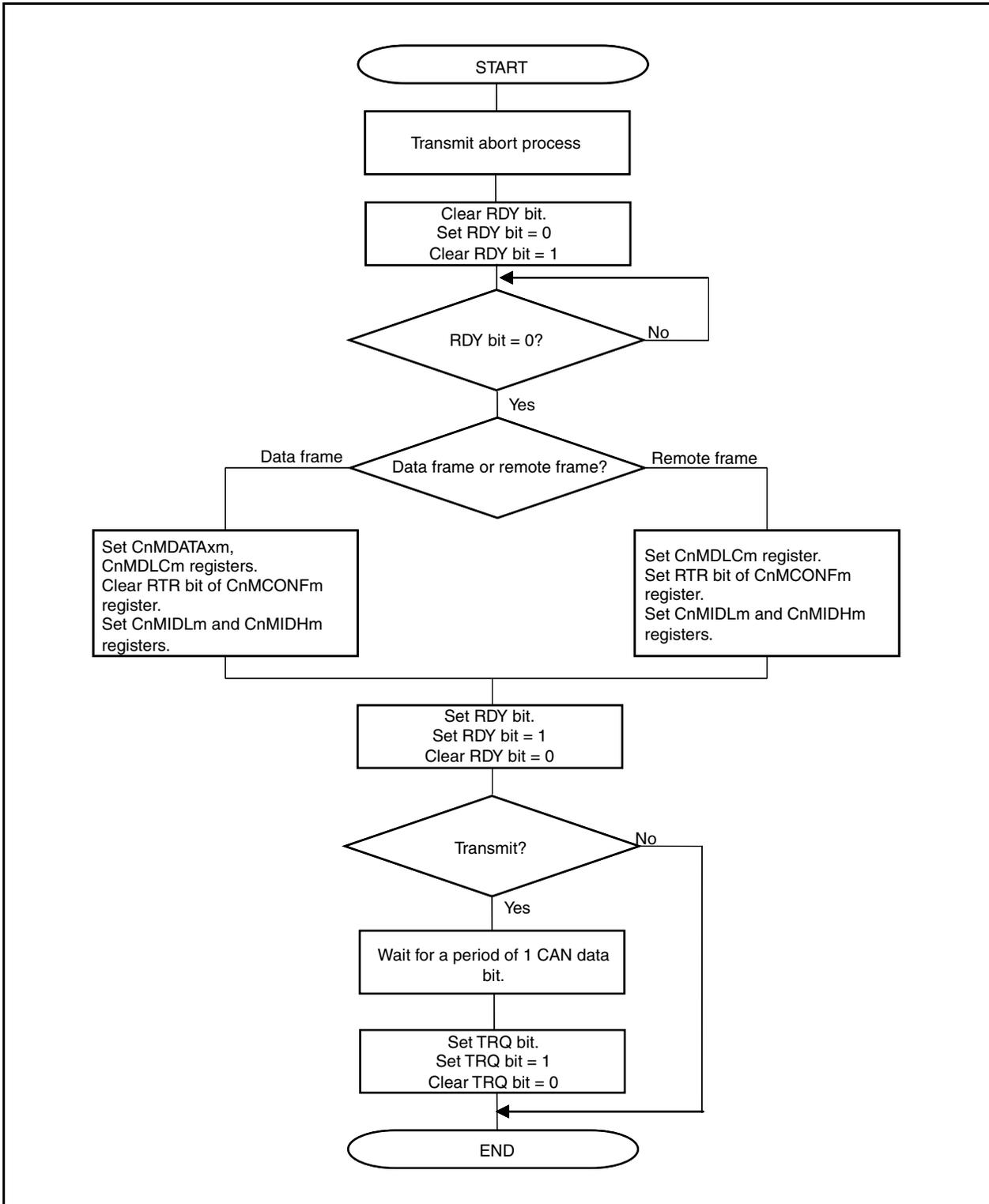
Figure 19-41 shows the processing for a transmit message buffer (CnMCONFm.MT2 to CnMCONFm.MT0 bits = 000B).
