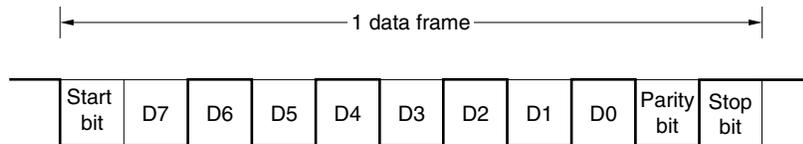
(c) 8-bit data length, MSB first, even parity, 1 stop bit, transfer data: 55H, TXDAn inversion
