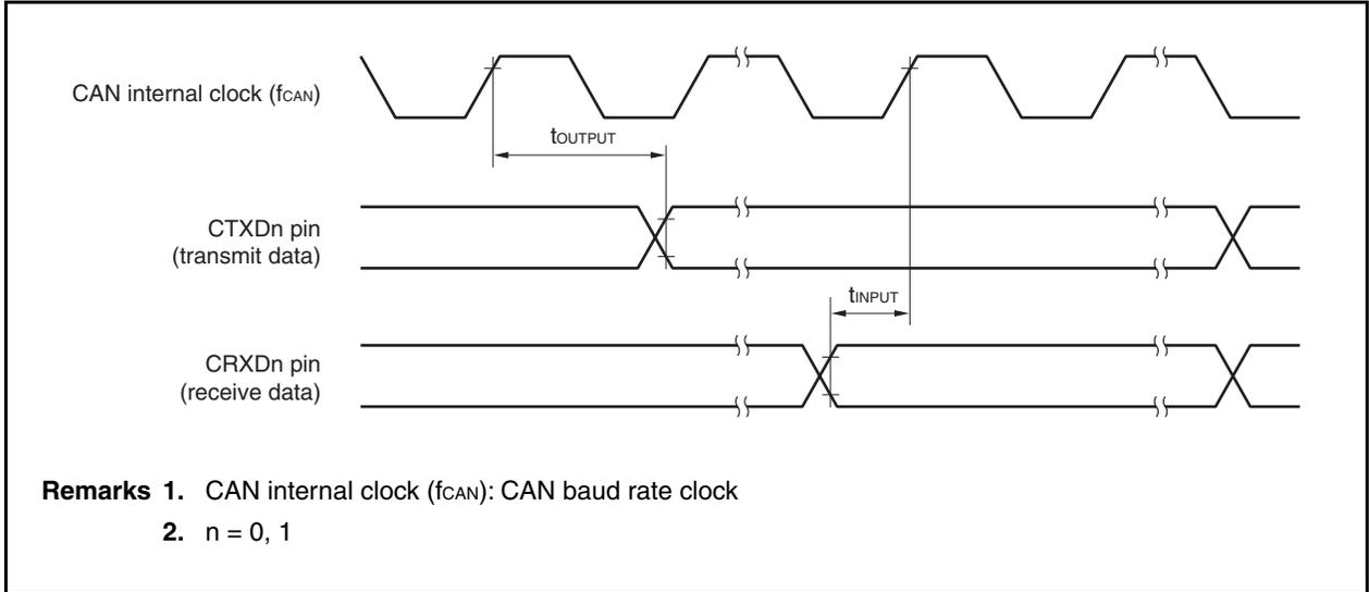
Internal delay time ( $t_{NODE}$ ) = Internal transmission delay time ( $t_{OUTPUT}$ ) + Internal reception delay time ( $t_{INPUT}$ )
