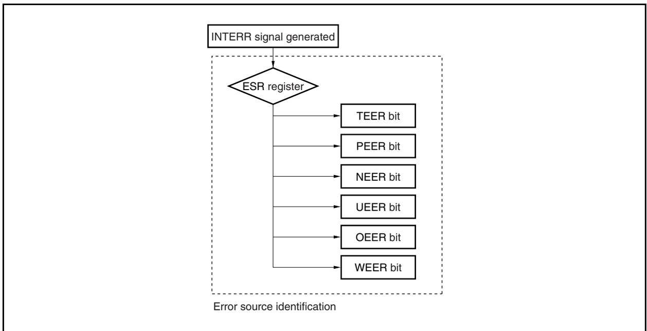
**Figure 18-23. Example of Identifying INTSTA Signal Interrupt (When INTIE1, INTERR, and INTSTA Signals Are Used)**
