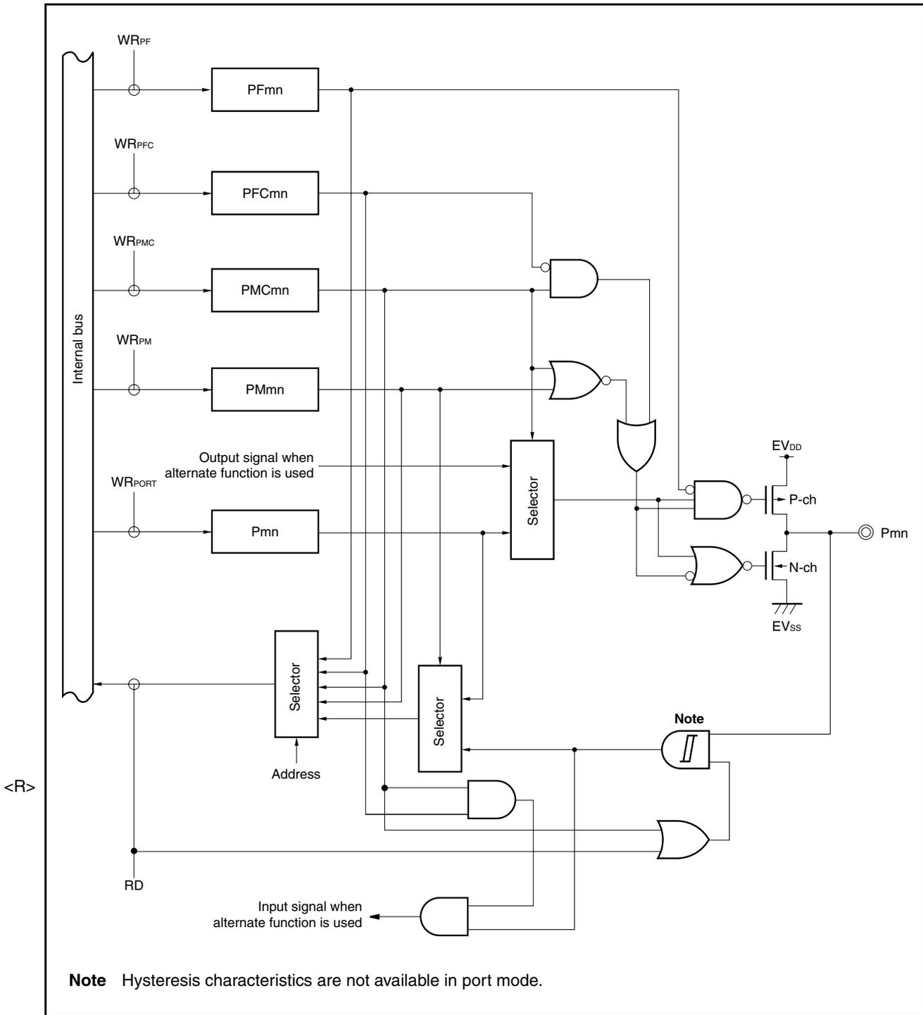
Figure 4-15. Block Diagram of Type G-3
