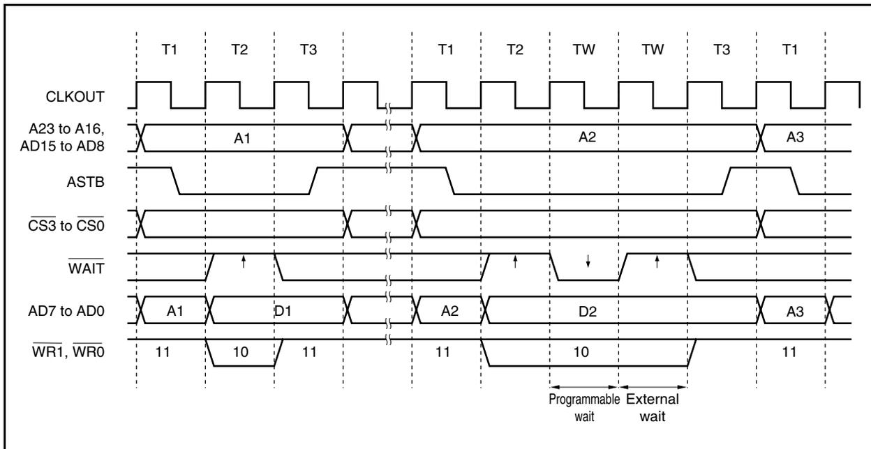
Figure 5-8. Multiplexed Bus Hold Timing (Bus Size: 16 Bits, 16-Bit Access)
