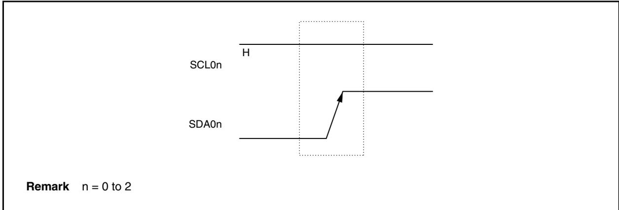
A stop condition is generated when the IICCn.SPTn bit is set to 1. When the stop condition is detected, the IICSn.SPDn bit is set to 1 and the interrupt request signal (INTIICn) is generated when the IICCn.SPIEn bit is set to 1 (n = 0 to 2).
