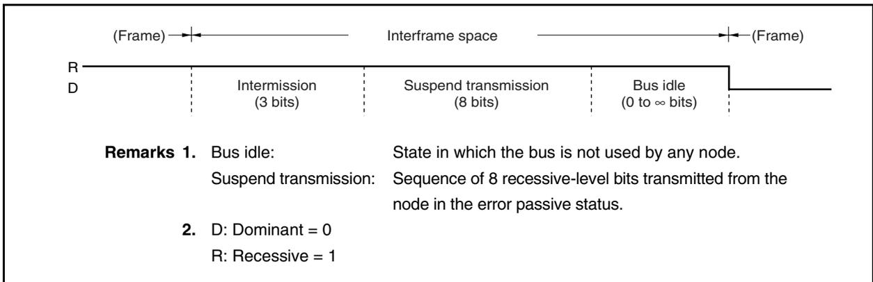
Usually, the intermission field is 3 bits. If the transmitting node detects a dominant level at the third bit of the intermission field, however, it executes transmission.
