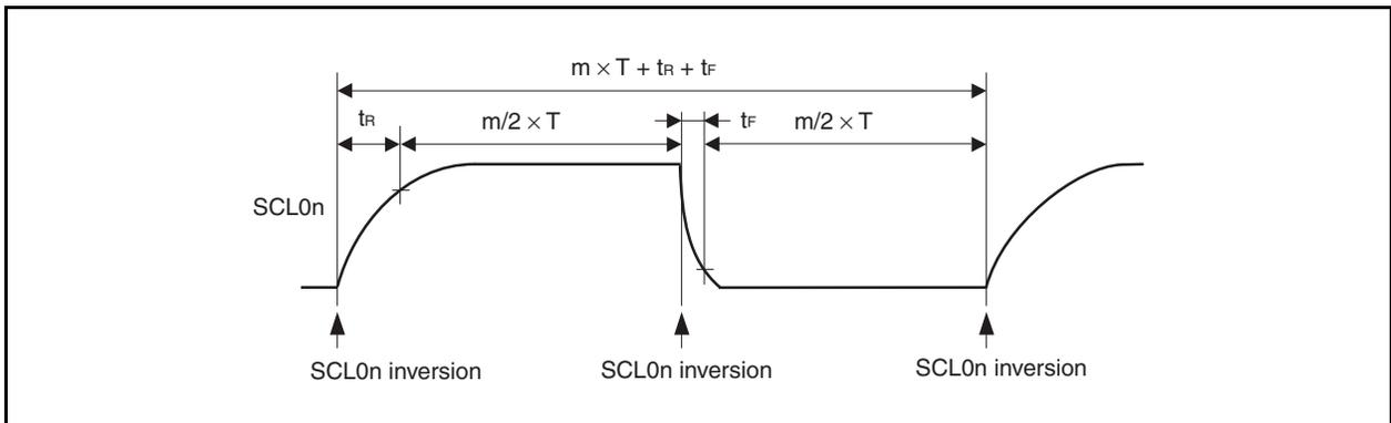
The clock to be selected can be set by the combination of the IICCLn.SMCn, IICCLn.CLn1, and IICCLn.CLn0 bits, the IICXn.CLXn bit, and the OCKSm.OCKSTHm, OCKSm.OCKSm1, and OCKSm.OCKSm0 bits (n = 0 to 2, m = 0, 1).
