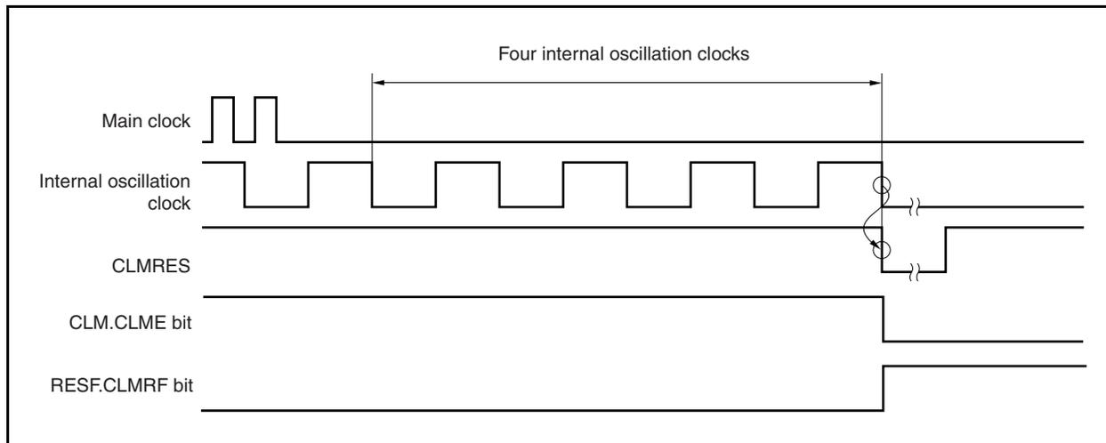
**(2) Clock monitor status after  $\overline{\text{RESET}}$  input**
