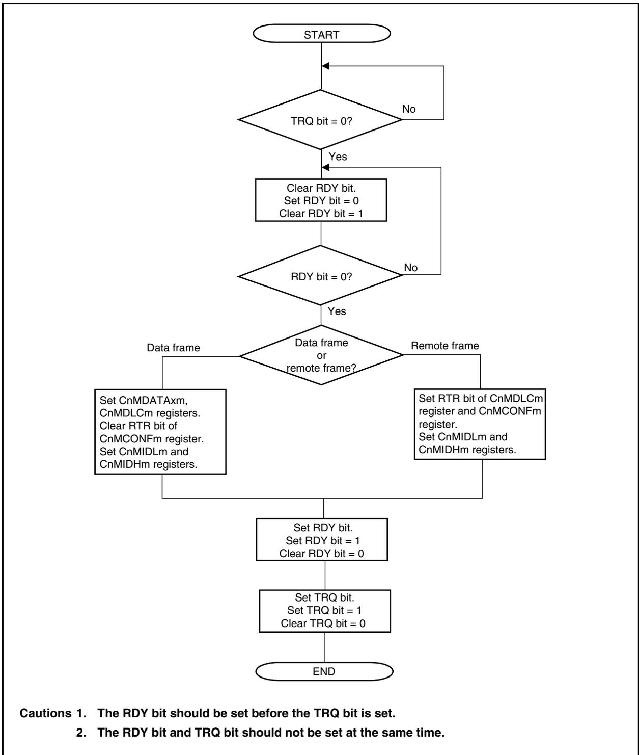
Figure 19-42 shows the processing for a transmit message buffer (CnMCONFm.MT2 to CnMCONFm.MT0 bits = 000B).
