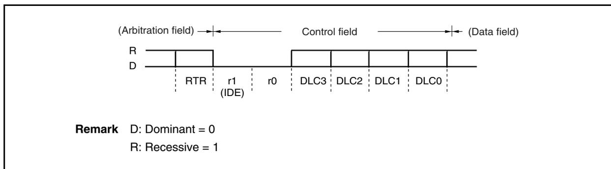
In a standard format frame, the control field’s IDE bit is the same as the r1 bit.
