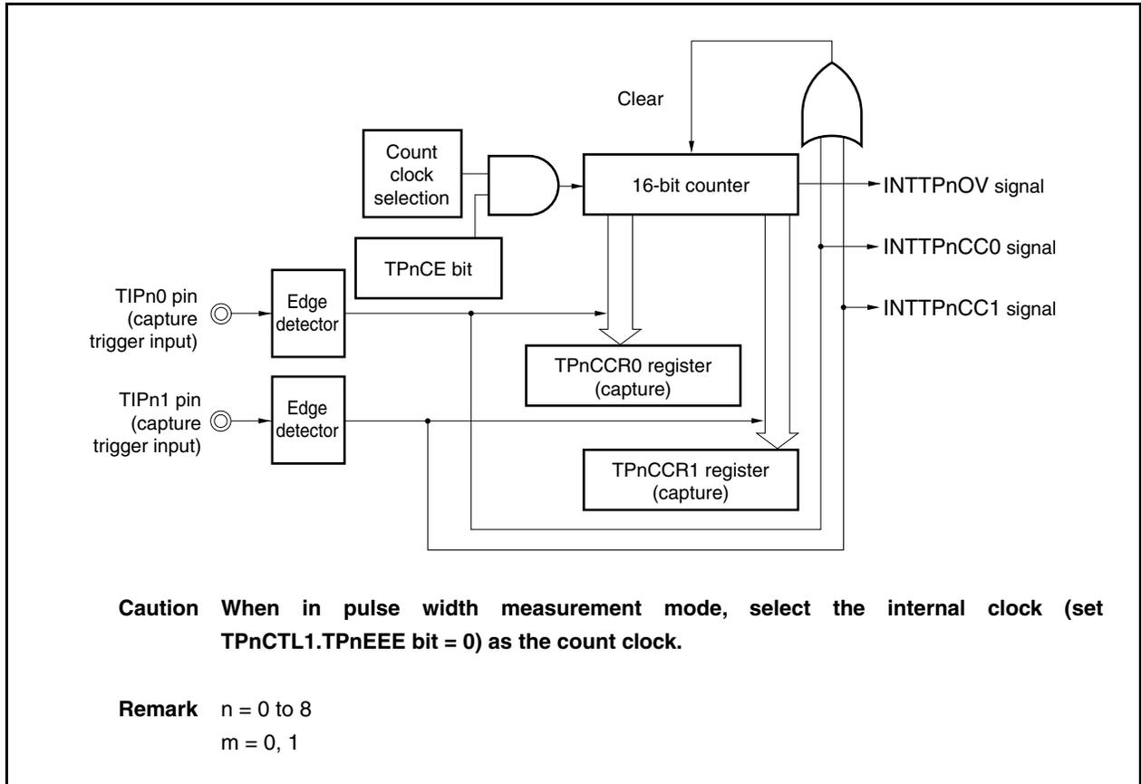
Figure 7-39. Basic Timing in Pulse Width Measurement Mode
