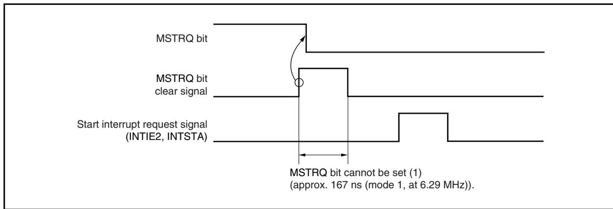
2. When a master request has been sent and bus mastership acquired, do not set the MSTRQ, ENSLVTX, or ENSLVRX bit until the end of communication (i.e. the communication end flag (ISR.ENDTRNS bit) or frame end flag (ISR.ENDFRAM bit) is set (1)) as setting these flags disables interrupt request signal generation. However, these flags can be set if communication has been aborted.
