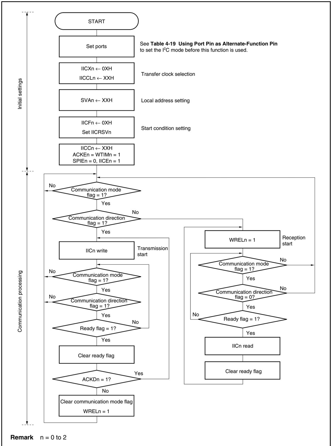
The following shows an example of the processing of the slave device by an INTIICn interrupt (it is assumed that no extension codes are used here). During an INTIICn interrupt, the status is confirmed and the following steps are executed.
