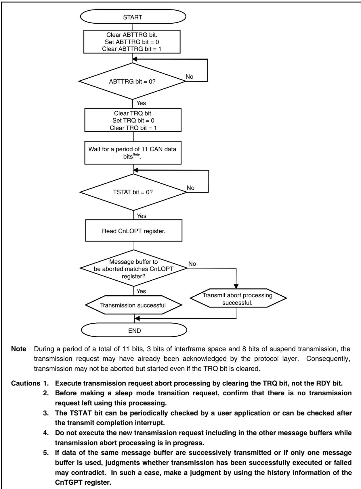
Figure 19-48 (a) shows processing that does not skip resuming the transmission of a message that was interrupted when the transmission of an ABT message buffer was aborted.
