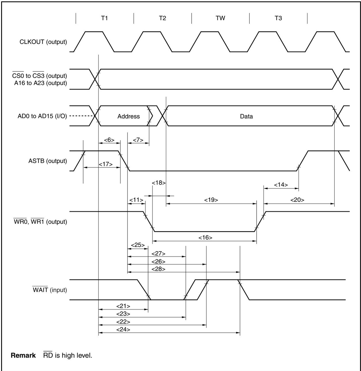
**(b) Read/write cycle (CLKOUT synchronous): In multiplexed bus mode**
