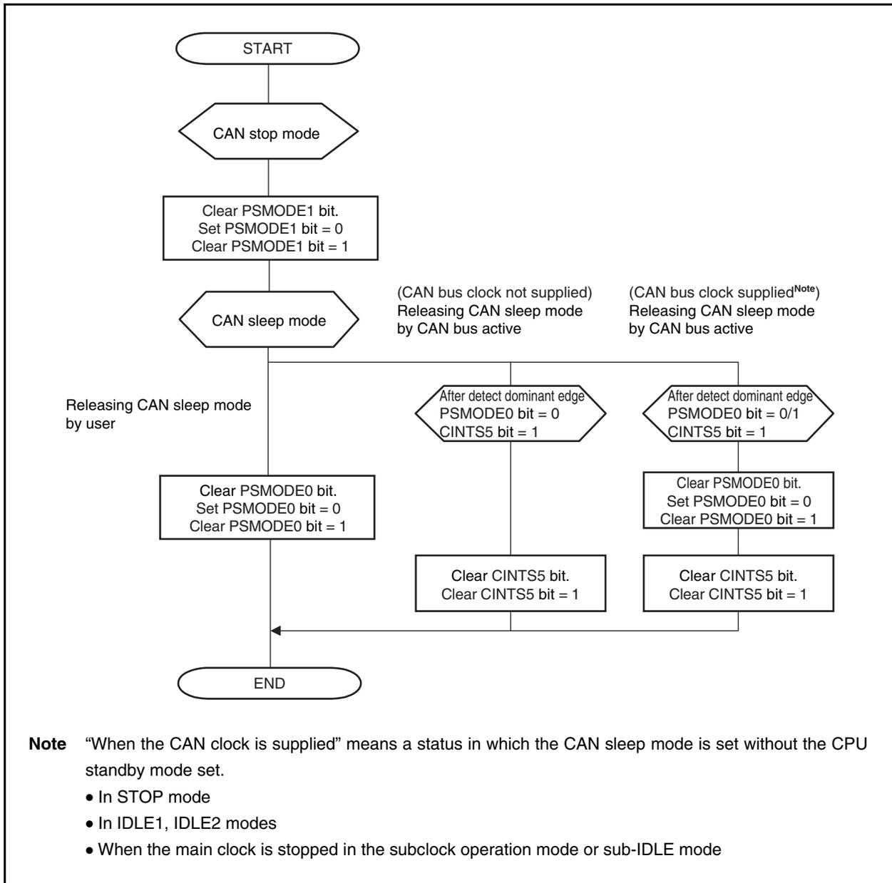
Figure 19-54. Bus-off Recovery (Other Than in Normal Operation Mode with ABT)
