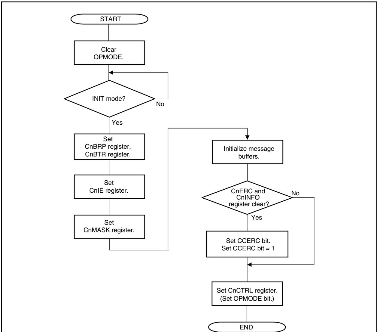
**Caution** After setting the CAN module to the initialization mode, avoid setting the module to another operation mode immediately after. If it is necessary to immediately set the module to another operation mode, be sure to access registers other than the CnCTRL and CnGMCTRL registers (e.g., set a message buffer).
