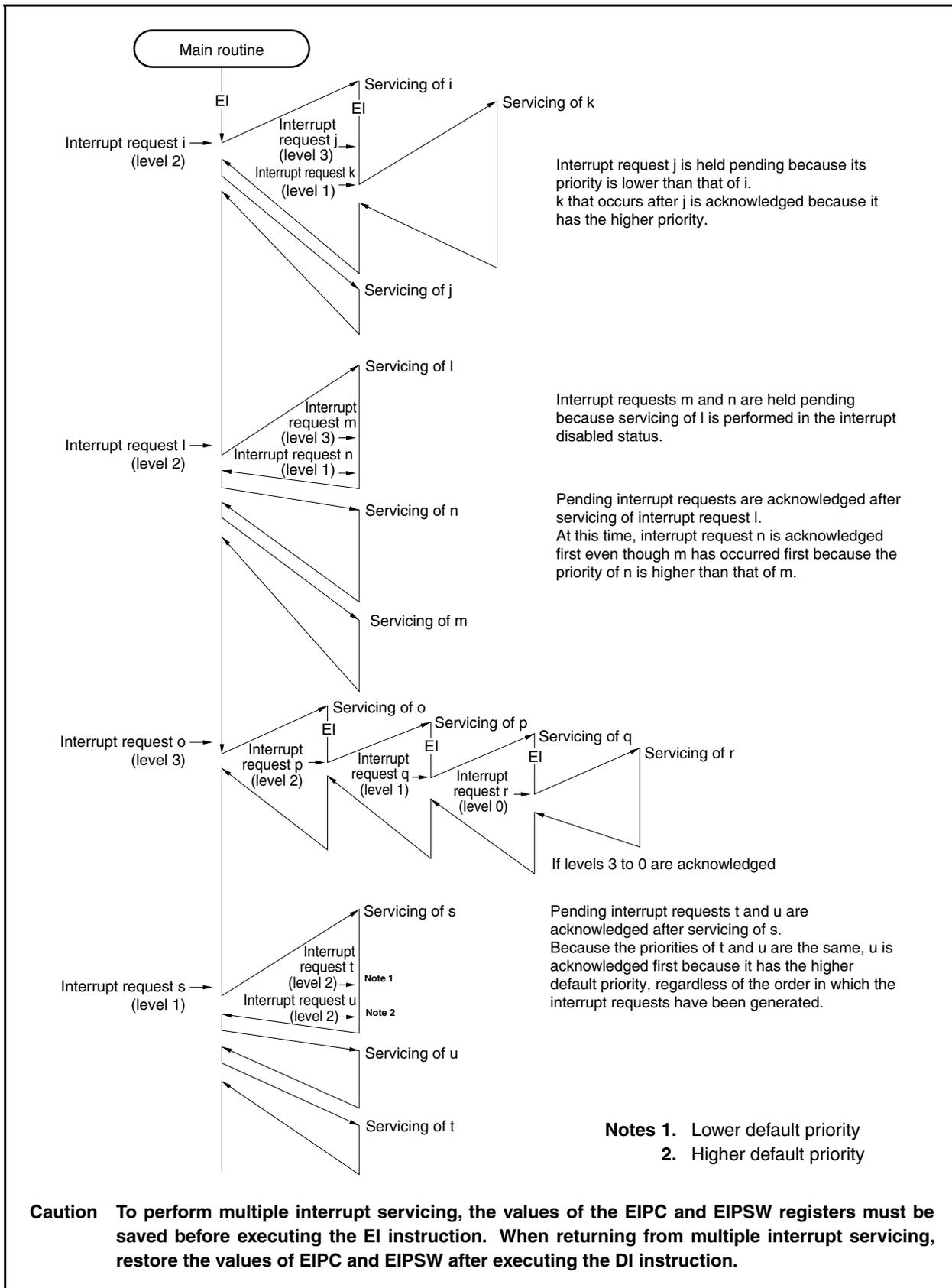
Figure 22-8. Example of Servicing Interrupt Request Signals Simultaneously Generated
