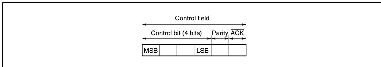
Table 18-5. Acknowledge Signal Output Condition of Control Field
