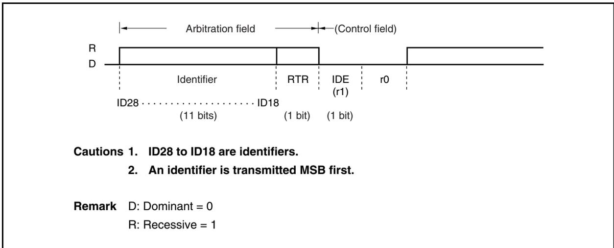
Figure 19-7. Arbitration Field (in Extended Format Mode)
