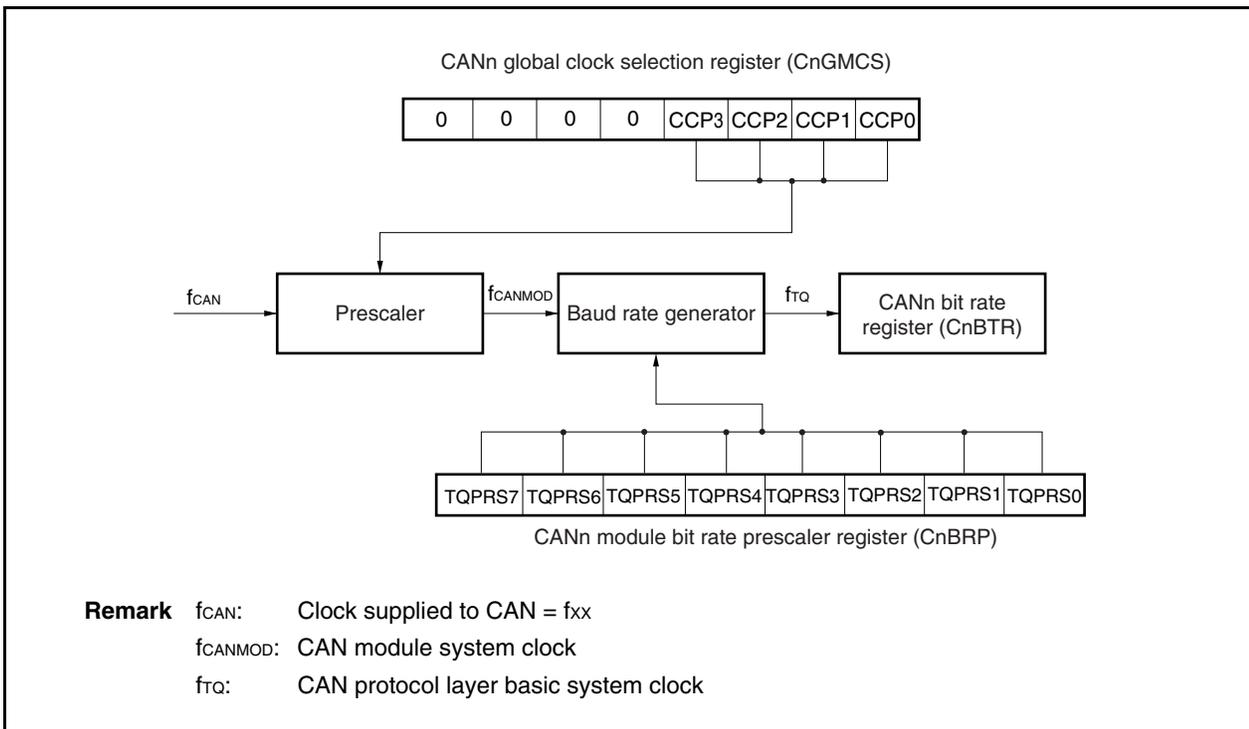
**(13) CANn module bit rate register (CnBTR)**
