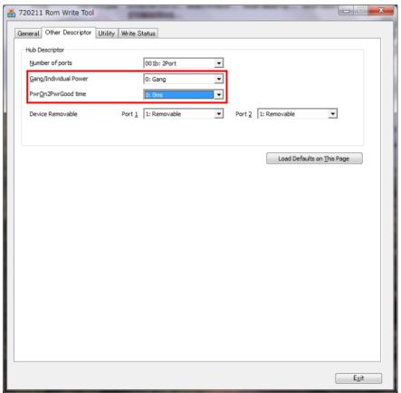
2. Or, use a power switch in gang mode. In this case, PwrOn2Pwrgood time should be "1: 100ms" in the uPD720211 ROM Writing Tool and using this workaround has no effect on power consumption.
