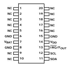
FIGURE 1. ISL12022M PINOUT
