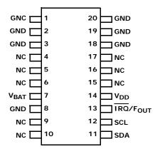
FIGURE 2. ISL12022MA PINOUT
