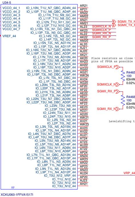
Place resistors as close to pins of FPGA as possible
