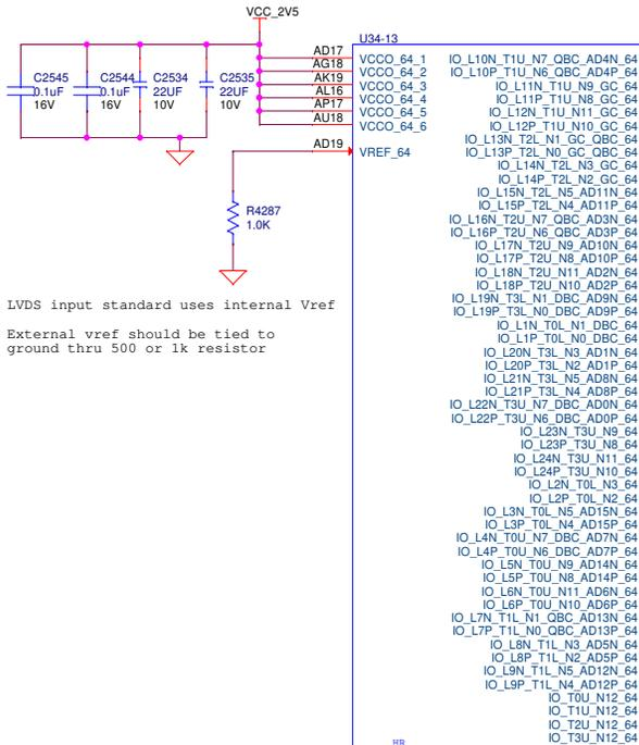
LVDS input standard uses internal Vref
