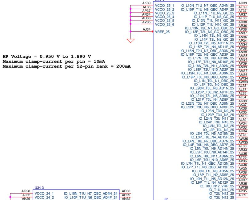
AR# 72582 Space-Grade XQR0060 will prohibit you from placing memory (D08) interfaces in bank 25 and/or bank 46 due to corner pads not being bonded out to package
