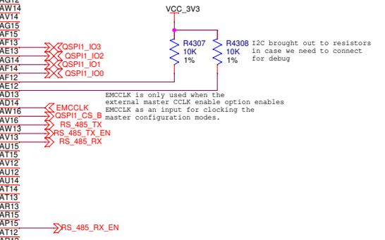
EMCCLK is only used when the external master CLK enable option enables EMCCLK as an input for clocking the master configuration modes.
