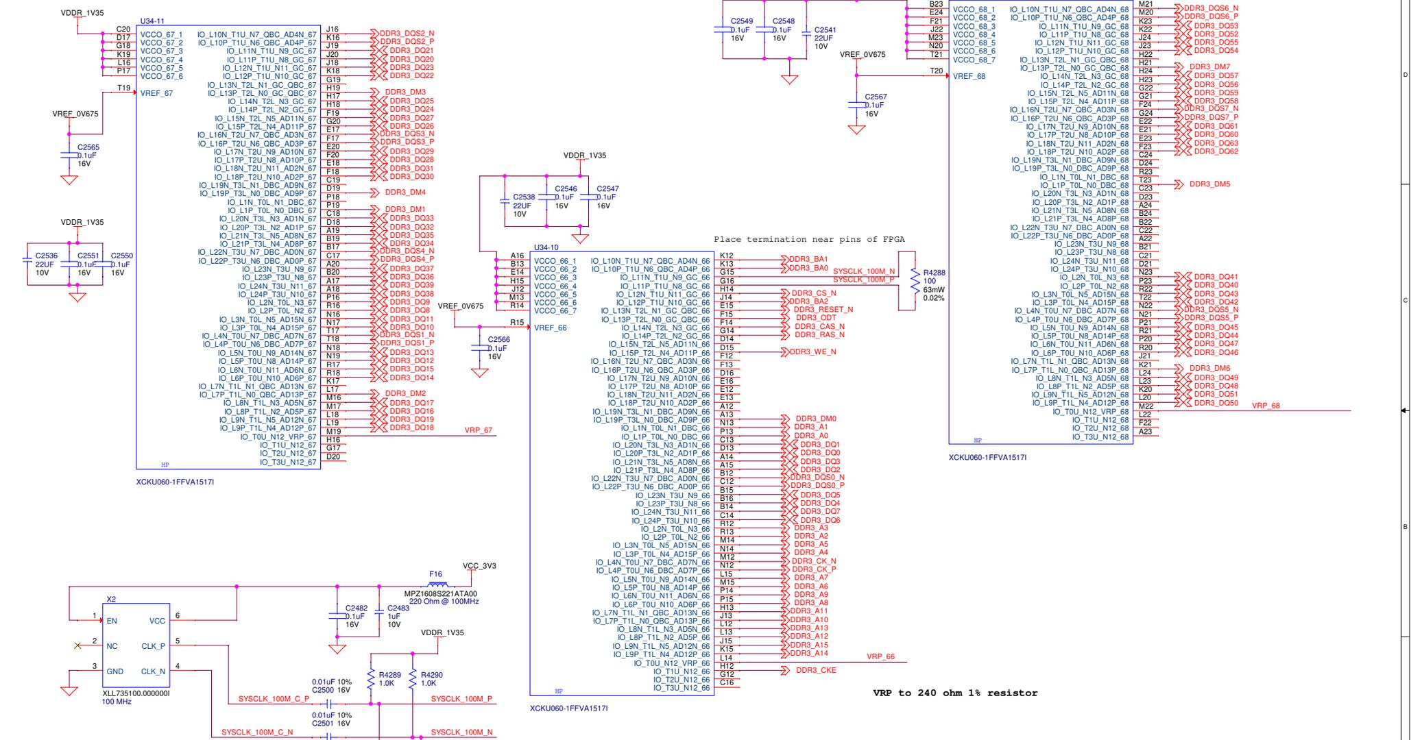
Place termination near pins of FPGA
