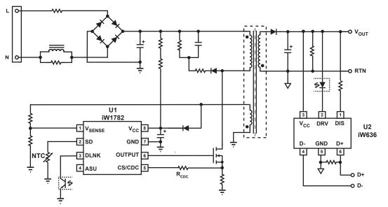
Figure 3.3 : iW1782 Typical Low Cost Application Circuit for Multi-Level Output Voltage and Current (Using iW636 as Secondary-Side Controller for QC3.0. Achieving < 50mW No-Load Power Consumption Without Using Active Start-up Device)
