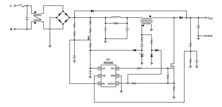
Figure 3.1 : iW2206 PFC Boost Application Circuit
