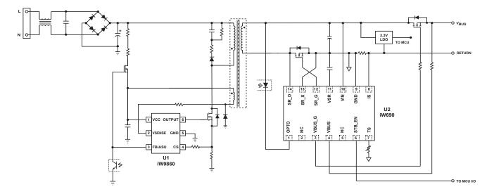
Figure 3. iW9860 Typical Application Circuit for Fixed Output Voltage, Zero Standby Power (Using iW690 as Secondary-Side Controller, Achieving < 5mW No-Load Power Consumption).
