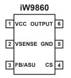
Figure 4. SOT23-6 Package (Top View)
