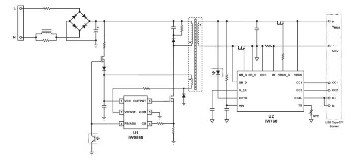
Figure 1. iW9860 Typical Application Circuit with Active Start-up Circuit (Using iW760 as Secondary-Side Controller. Achieving < 5mW Standby Power Consumption at 230V<sub>AC</sub>)
