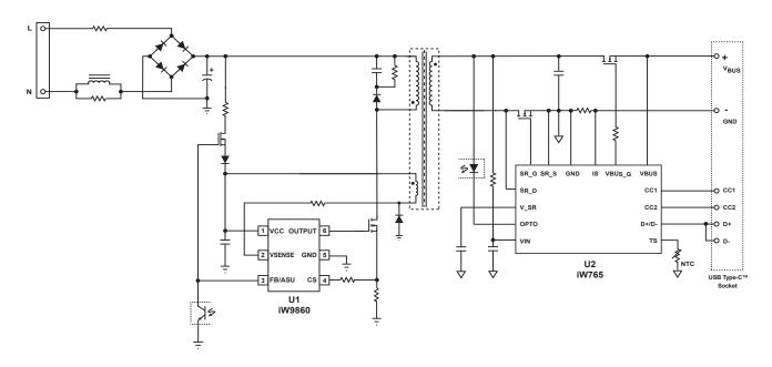
Figure 2. iW9860 Typical Application Circuit with Active Start-up Circuit (Using iW765 as Secondary-Side Controller. Achieving < 5mW Standby Power Consumption at 230V<sub>AC</sub>)
