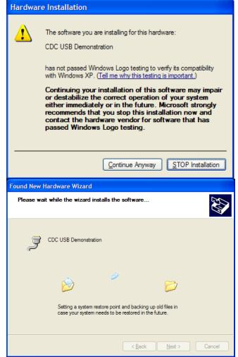
An additional COM port will become available to Window Applications. To be able to see the port that has been allocated you can open the Windows Device Manager window. To do this, go to the start menu and select run. In the dialog displayed type "devmgmt.msc". This will open the device manager. Expand the group of serial ports and the installed ports will be listed. When the Serial Terminal program connects to this COM port<sup>\*</sup>, it will receive a repeating message from the RSK saying:
