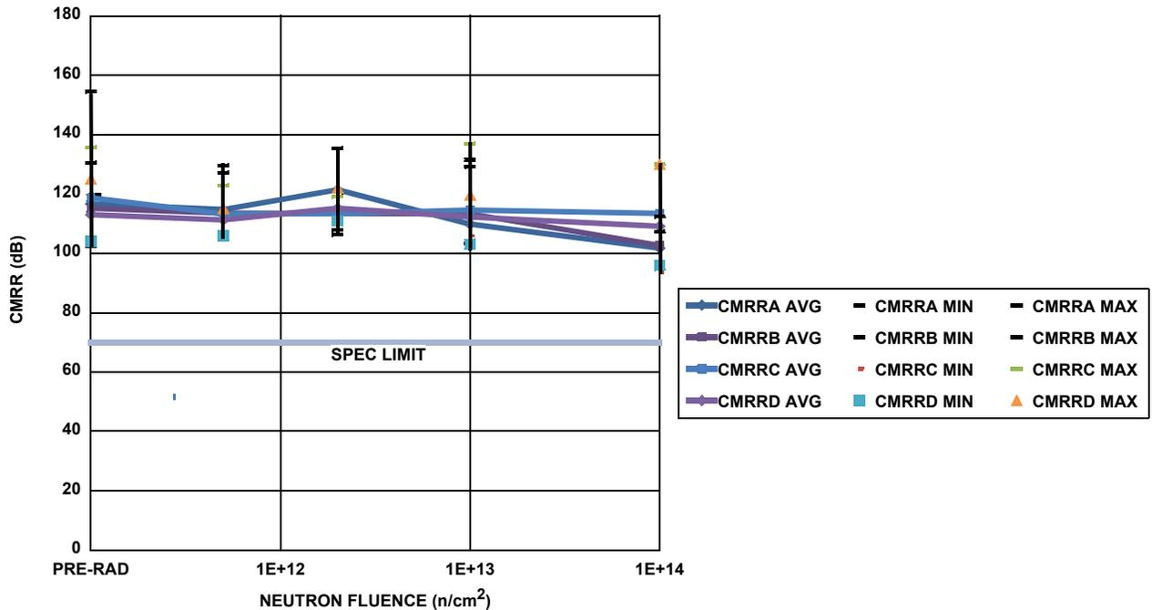
FIGURE 12. ISL70444SEH common mode rejection ratio as a function of neutron irradiation, showing the mean, minimum and maximum of the populations at each level. Sample size was 5 for each cell ( $5 \times 10^{11} \text{ n/cm}^2$ ,  $2 \times 10^{12} \text{ n/cm}^2$ ,  $1 \times 10^{13} \text{ n/cm}^2$  and  $1 \times 10^{14} \text{ n/cm}^2$ ), with two control units. The post-total dose irradiation SMD limit is 70dB minimum.
