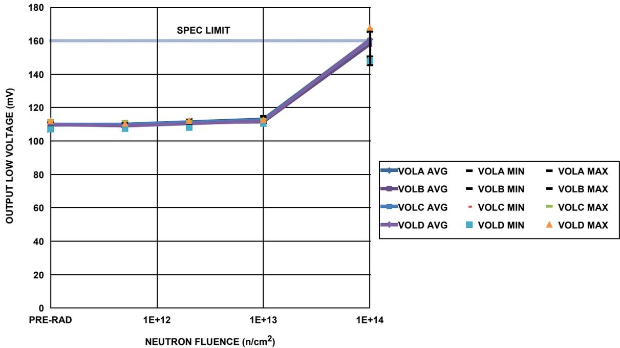
FIGURE 7. ISL70444SEH output LOW voltage as a function of neutron irradiation, no load, showing the mean, minimum and maximum of the populations at each level. Sample size was 5 for each cell ( $5 \times 10^{11} \text{ n/cm}^2$ ,  $2 \times 10^{12} \text{ n/cm}^2$ ,  $1 \times 10^{13} \text{ n/cm}^2$  and  $1 \times 10^{14} \text{ n/cm}^2$ ), with two control units. The post-total dose irradiation SMD limit is 160mV maximum.
