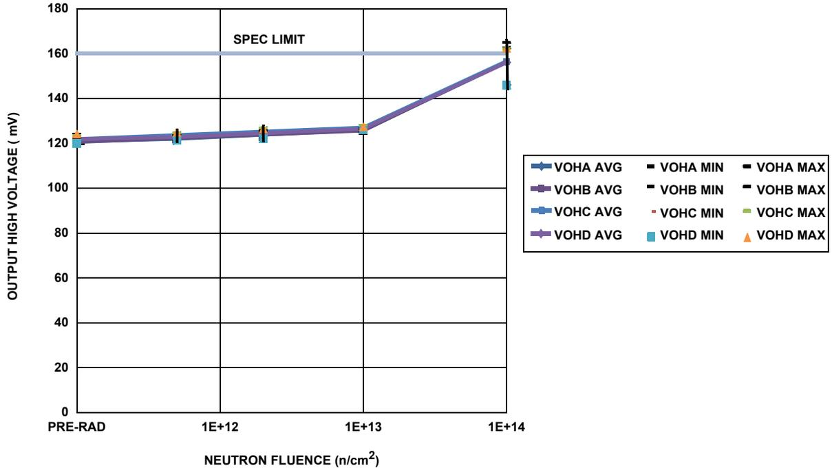
FIGURE 6. ISL70444SEH output HIGH voltage as a function of neutron irradiation, each channel, no load, showing the mean, minimum and maximum of the populations at each level. Sample size was 5 for each cell ( $5 \times 10^{11} \text{ n/cm}^2$ ,  $2 \times 10^{12} \text{ n/cm}^2$ ,  $1 \times 10^{13} \text{ n/cm}^2$  and  $1 \times 10^{14} \text{ n/cm}^2$ ), with two control units. The post-total dose irradiation SMD limit is 160mV maximum.
