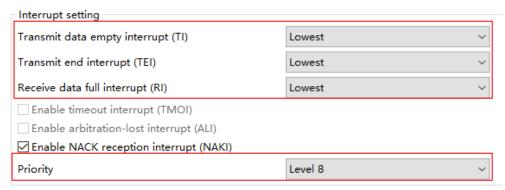
Figure 5-1. RIIC interrupt priority setting
