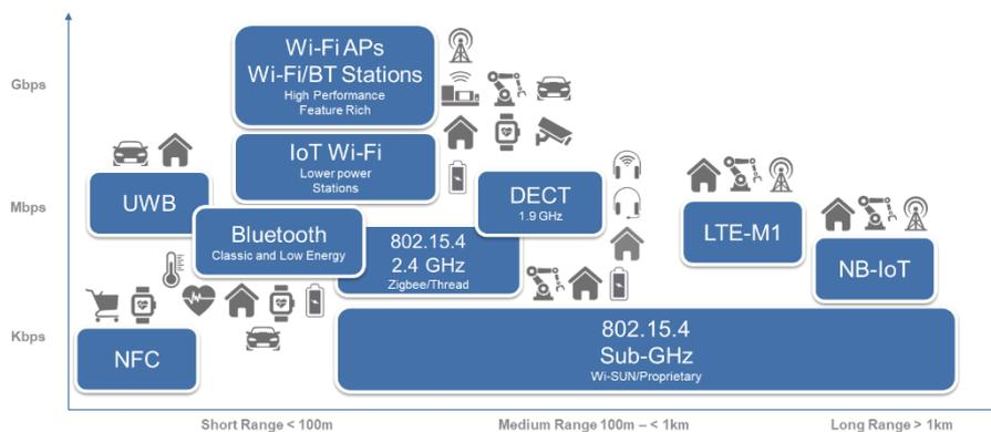
Figure 1: Wireless connectivity technologies and IoT applications
