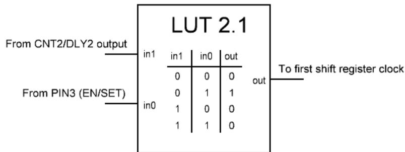
**Figure 7. 2-bit LUT1 truth table**
