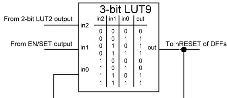
Figure 3. Active LOW latch truth table
