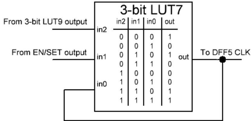
Figure 4. 3-bit LUT7 truth table
