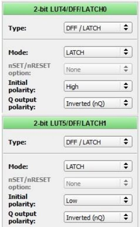
Figure 3. Latches configuration
