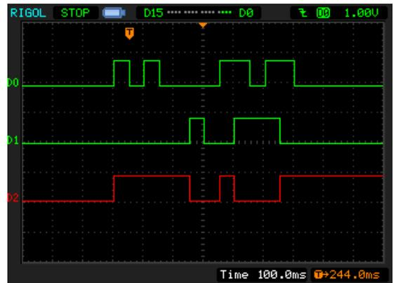
Figure 4. RS flip flop functional diagram
