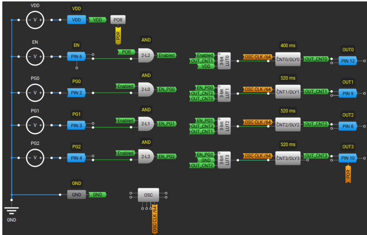
Figure 5. Power up and down sequencer with PG input block diagram
