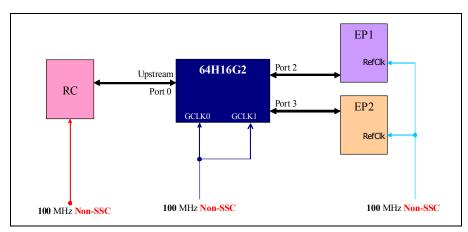
Figure 9 Example of Non-Common Clock Mode
