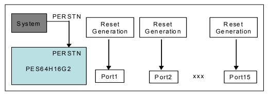
Figure 13 Reset Scheme for Hot Plug Support
