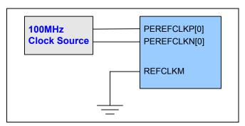
Figure 6 100 MHz Global Reference Clock Selection
