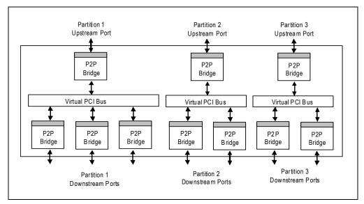
Figure 19 Example of Switch Partitioning
