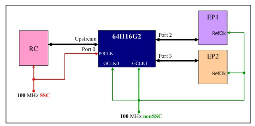
Figure 10 Example of Local Port Clock mode with SSC on Root Complex
