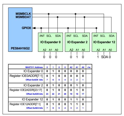
Figure 16 Example of I/O Expander Interface
