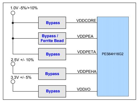
Figure 17 Board Power Supply Arrangement
