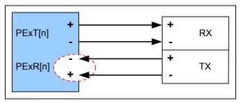
Figure 2 Polarity Inversion
