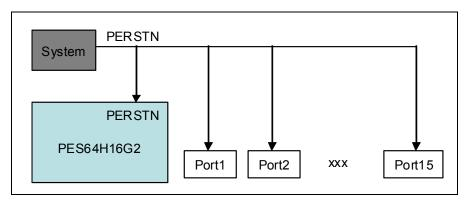
Figure 12 Simplified Reset Scheme
