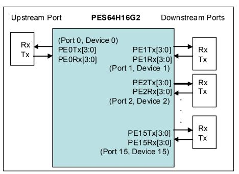
Figure 1 Port Numbering and Device Numbering
