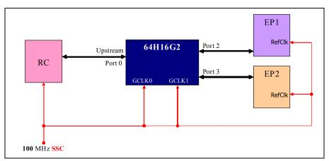
Figure 8 Example of Common Clock Mode with SSC
