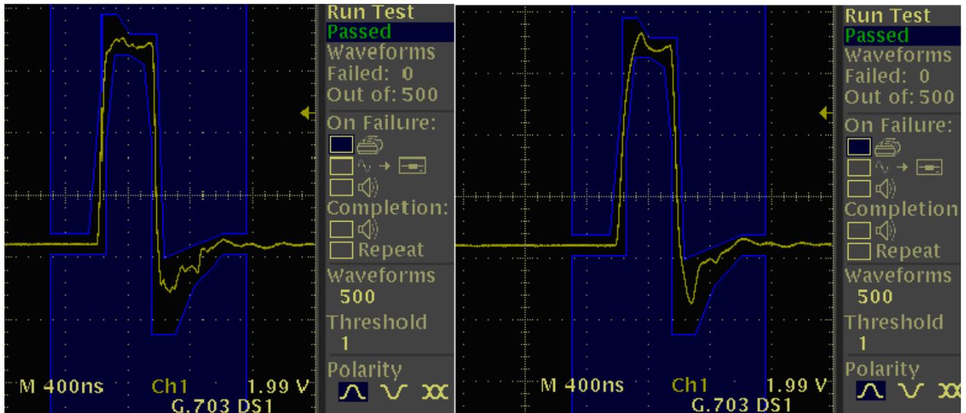
Note that transmit pulse shape is dependent on the line's overall impedance conditions. In actual applications, the specific values of these external components may need some adjustments to achieve optimal pulse shape.
