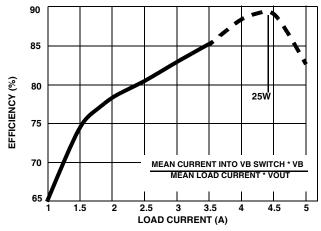
FIGURE 6. ISL6160EVAL2 EFFICIENCY vs LOAD CURRENT
