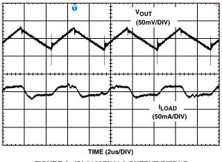
FIGURE 8. ISL6160EVAL2 OUTPUT RIPPLE
