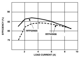
FIGURE 10. HIP6006EVAL1 EFFICIENCY WITH EITHER RFP25N05 OR RFP45N06 MOSFETs
