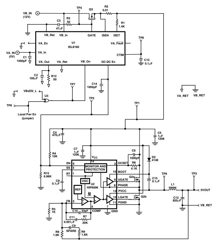
FIGURE 11. ISL6160EVAL2 SCHEMATIC
