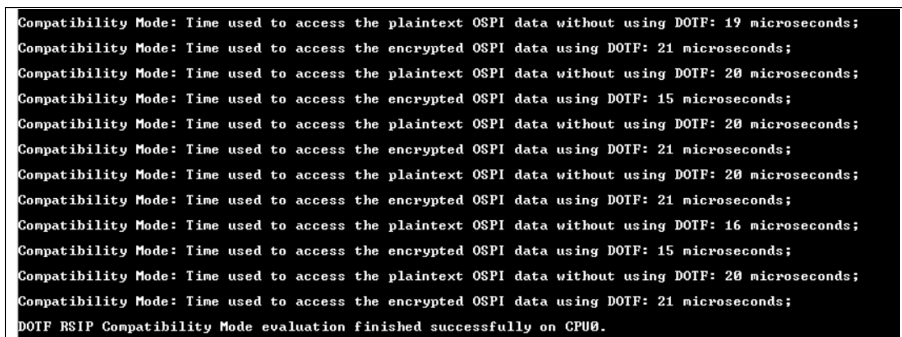
Figure 36. Access Plaintext and DOTF Decrypted Data in Compatibility Mode on RA8P1 (CPU0)
