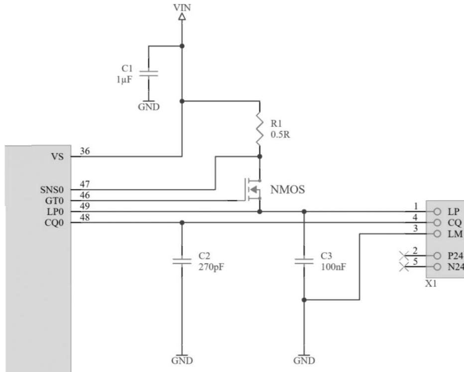
Figure 3. IO-Link Channel 0
