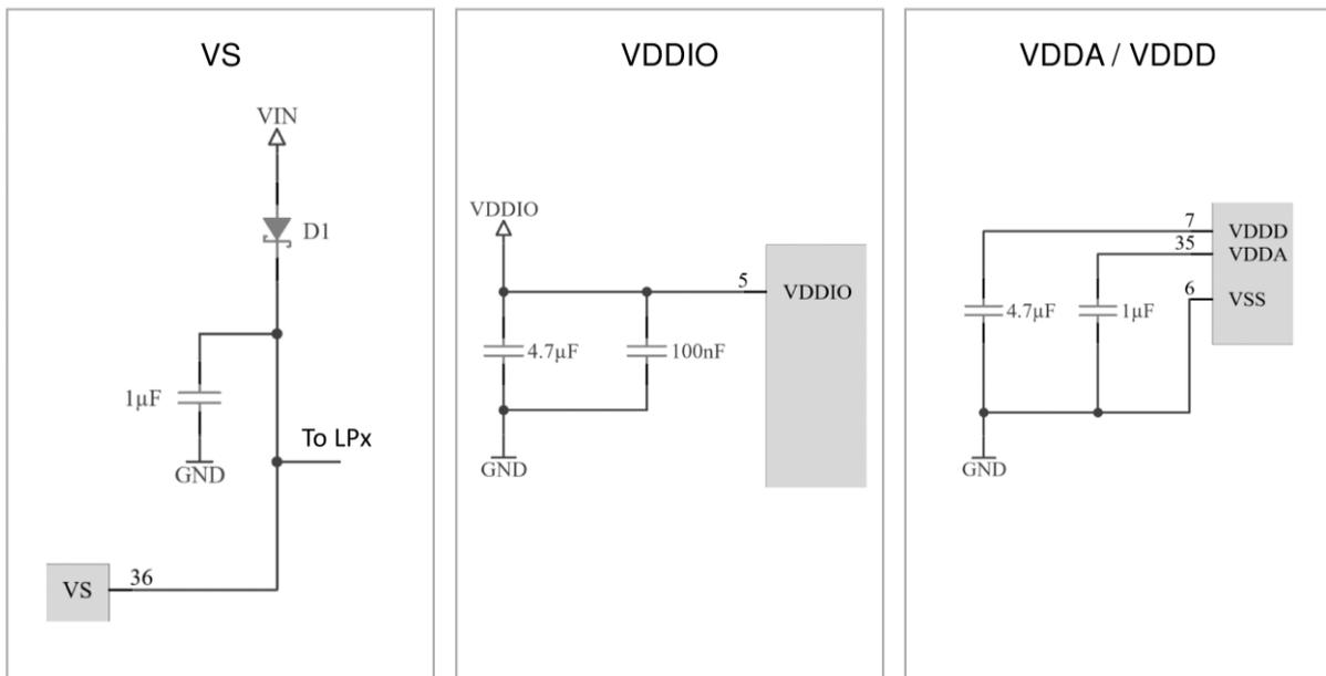
Figure 5. Power Supply Decoupling and Stabilization Network
