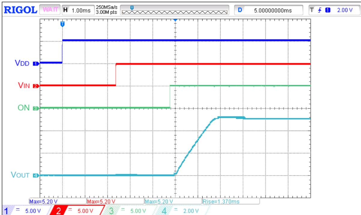
Figure 6. A Load Switch Powering Up a  $1\mu\text{F}$  Load Capacitor with Fast  $V_{DD}$  and  $V_{IN}$  rise Times.
