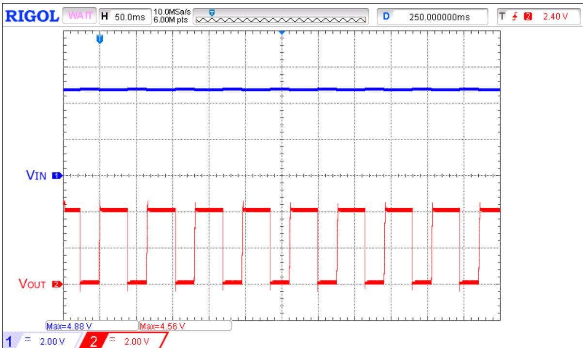
Figure 14. Adding 470  $\mu$ F Low ESR/ESL Aluminum Polymer Capacitor at  $V_{IN}$  Eliminates Voltage Spikes Caused by the Parasitic Inductance of the 1.2-m Length AWG13 Wires from Power Supply during Active Current Limit Operation.
