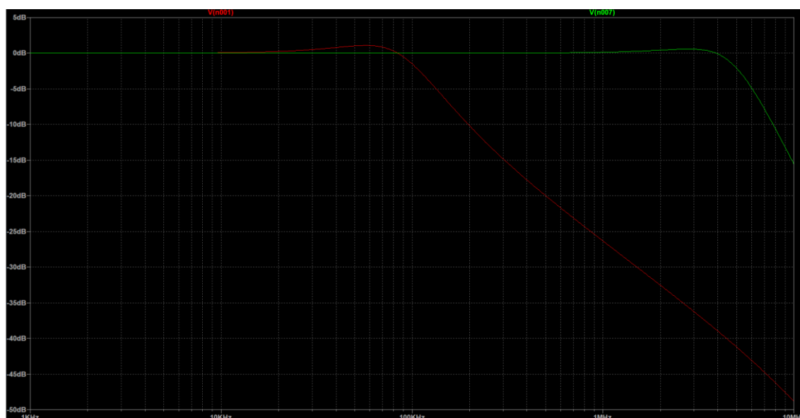
Figure 12. Simulated Frequency Response of a Filter Built on SLG47001/03 for Two Cutoff Frequencies
