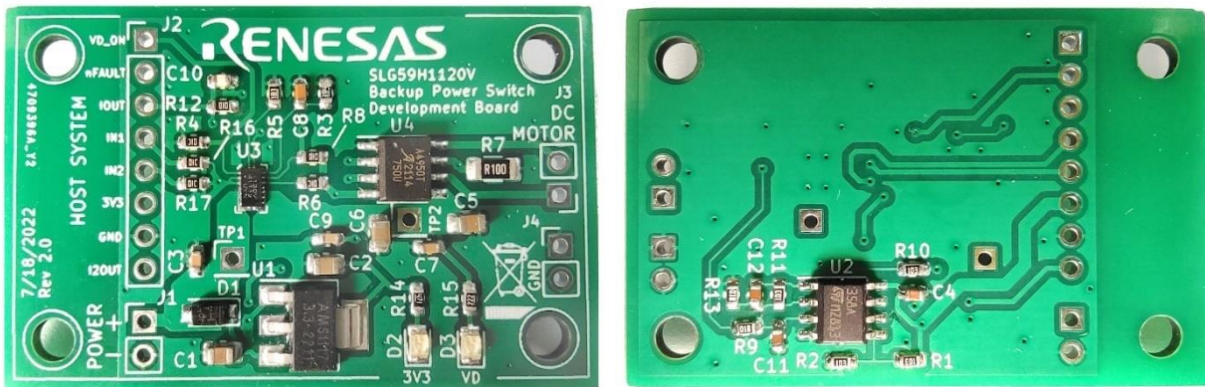
Figure 4. Experimental Module PCBA Front/Back View
