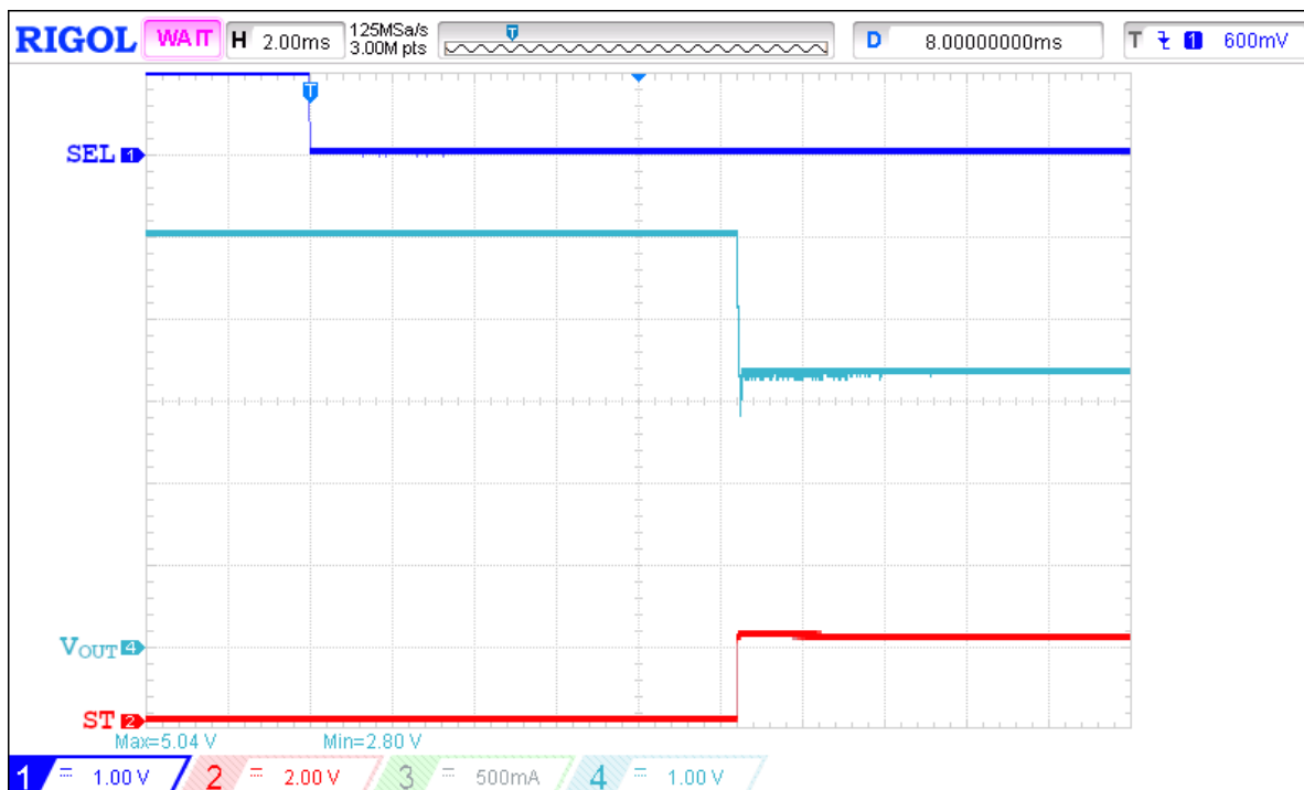
Figure 10: Switchover operation waveform for V_{IN1} = 3.3\text{ V} , V_{IN2} = 5\text{ V} , C_{SS} = 220\text{ nF} , PR = \text{High} , SEL = \text{High} \rightarrow \text{Low} , R_{LOAD} = 100\ \Omega , C_{LOAD} = 2\ \mu\text{F}
