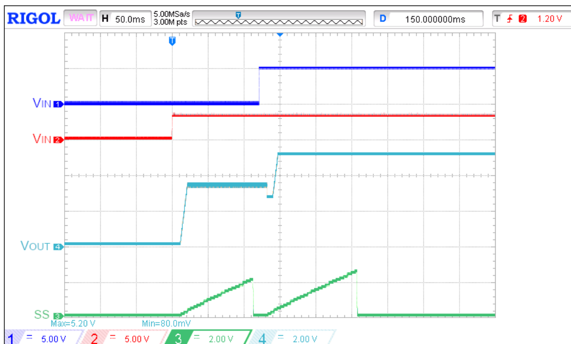
Figure 28: Higher voltage level priority operation waveform when V_{IN1} is applied after first SS rise is done for V_{IN1} = 5\text{ V} , V_{IN2} = 3.3\text{ V} , SEL = \text{Low} , PR = \text{Low} , C_{SS} = 220\text{ nF} , R_{LOAD} = 100\text{ }\Omega , C_{LOAD} = 2\text{ }\mu\text{F}
