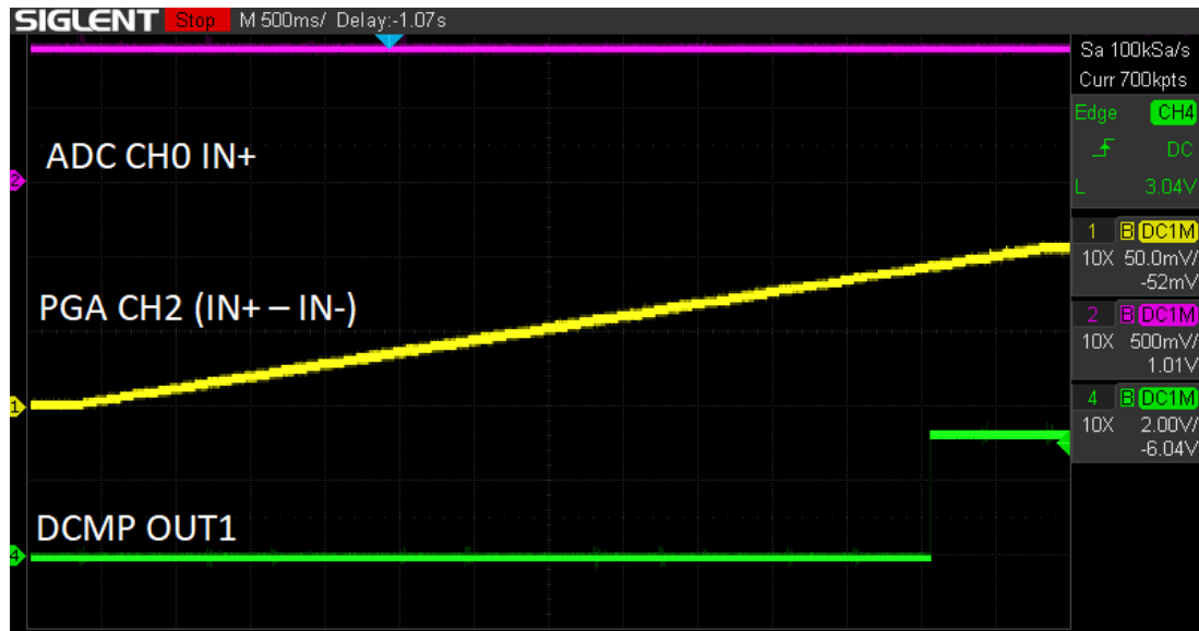
Figure 4. Waveform Illustrating Overpower Monitor
