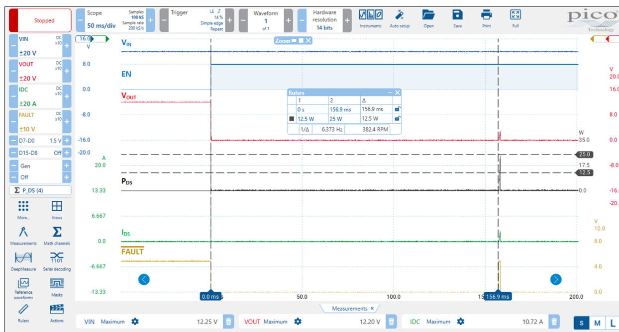
Figure 15: SLG59H1132V 25 W SOA operating waveform during Active Current Limit for V_{IN} = 12\text{ V} , C_{SLEW} = 10\text{ nF} , R_{SET} = 30.1\text{ k}\Omega , C_{LOAD} = 10\text{ }\mu\text{F} , R_{LOAD} = \text{switch in } 1\text{ }\Omega
