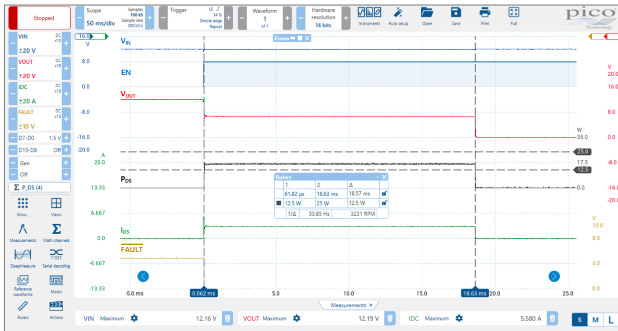
Figure 14: SLG59H1132V 12.5 W SOA operating waveform during Active Current Limit for V_{IN} = 12\text{ V} , C_{SLEW} = 10\text{ nF} , R_{SET} = 30.1\text{ k}\Omega , C_{LOAD} = 10\text{ }\mu\text{F} , R_{LOAD} = \text{switch in } 2\text{ }\Omega (Extended view)
