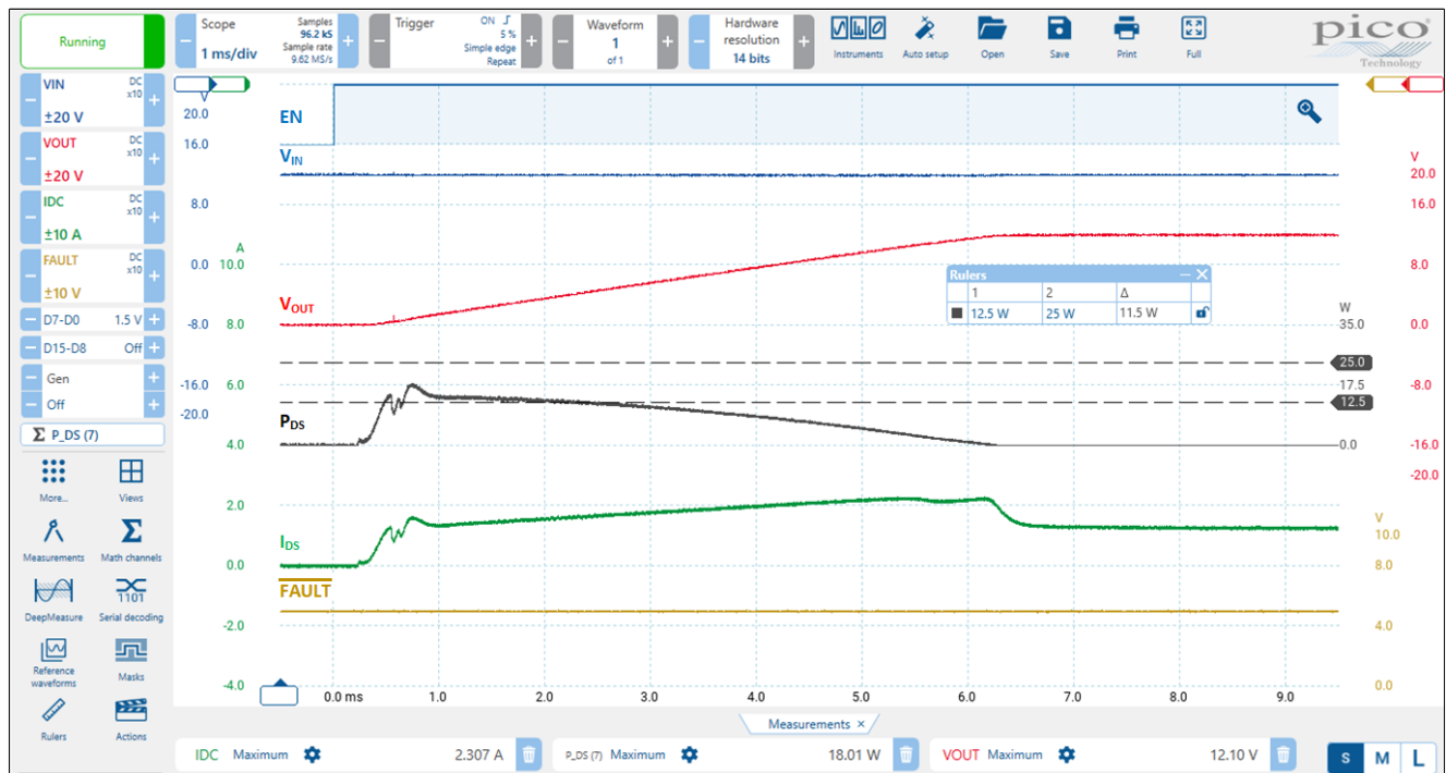
Figure 21. Turn-on operation waveform for V IN = 12 V, C SLEW = 16 nF, R SET = 14 kΩ, C LOAD = 600 μF, R LOAD = 10 Ω
