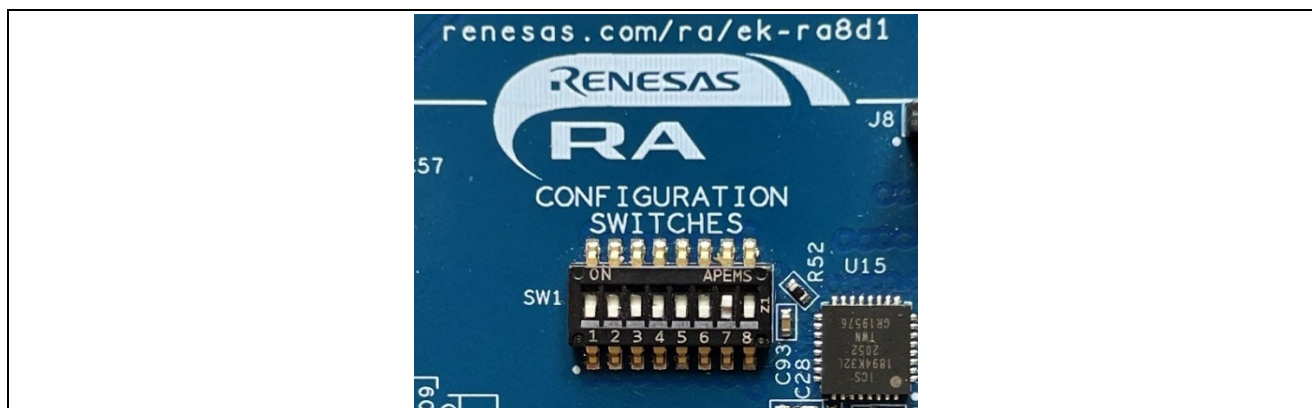
Figure 36. Enabling SW1-7 for SDRAM on the EK-RA8D1
