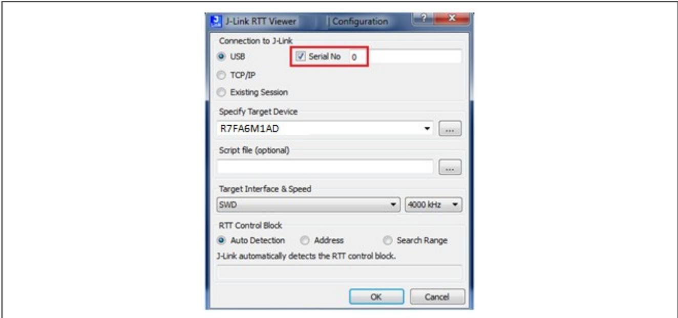
4. For parts other than Cortex-M33, click **OK**. For MCUs based on Cortex M33 Core, refer the Appendix.
