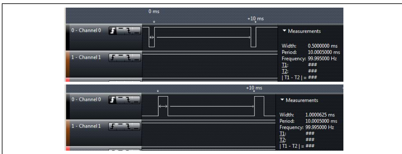
Figure 60. PWM Signals for Backlight Control
