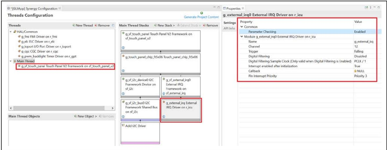
Figure 26. Configuring External IRQ Driver on r\_icu Properties
