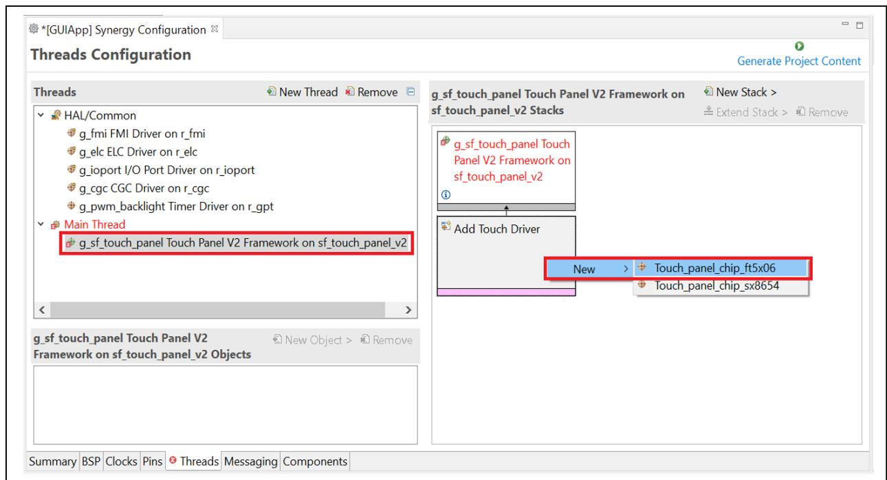
Figure 23. Add the Touch\_panel\_chip\_ft5x06 Touch driver
