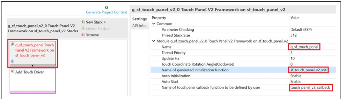
Figure 22. Configuring Touch Panel V2 Framework Properties
