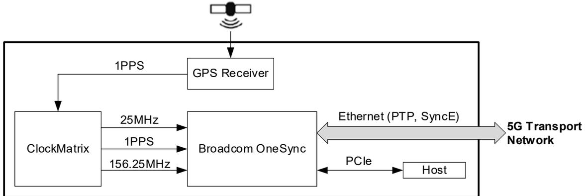
Figure 4. Clocking for Broadcom Ethernet Switch ASICs
