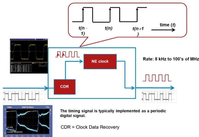
Figure 1. Example Clock Tree for Physical-Layer Synchronization (SyncE)
