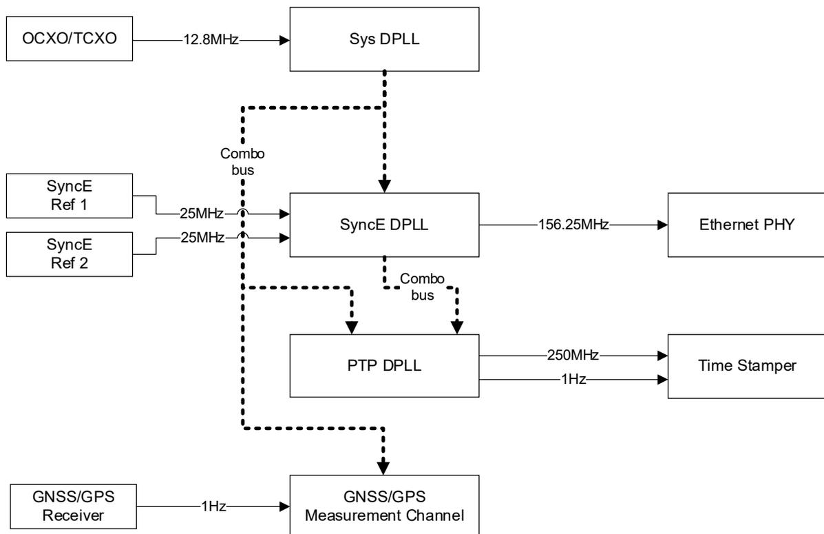
Figure 2. ClockMatrix Simplified Block Diagram
