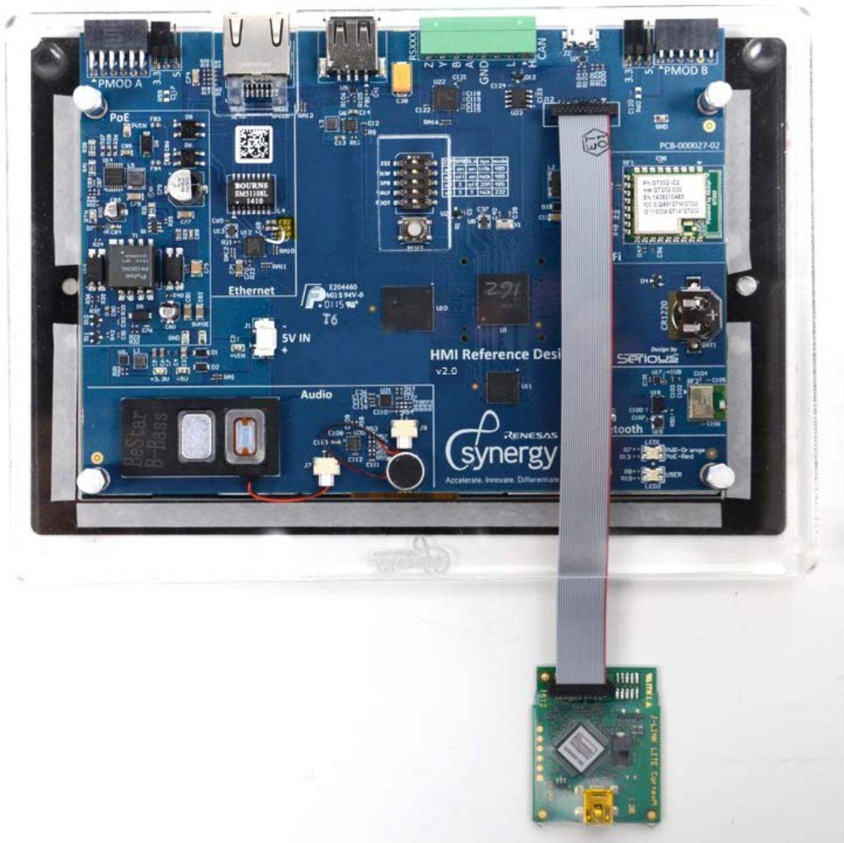
2. Connect the J-link Lite for Cortex M to the PC with the supplied USB cable. The LED on the J-link Lite for Cortex M illuminates solid green if communicating properly with the PC. If the LED is blinking, check the connection to the PC and make sure the drivers are loaded.
