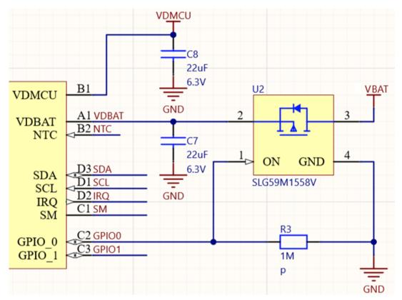
The circuit depicted above will keep the battery disconnected as long as there is no voltage on GPIO0. The GPIO0 is set high by the microcode running in the PTX30W. This guarantees that bootup and biasing of the charge pass transistor are completed before the battery gets connected.
