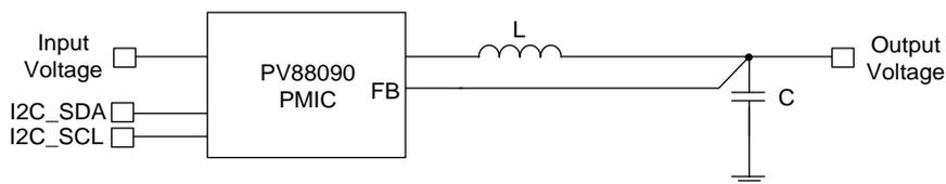
Figure 2: PV88090 Simplified Block Diagram for one Buck stage
