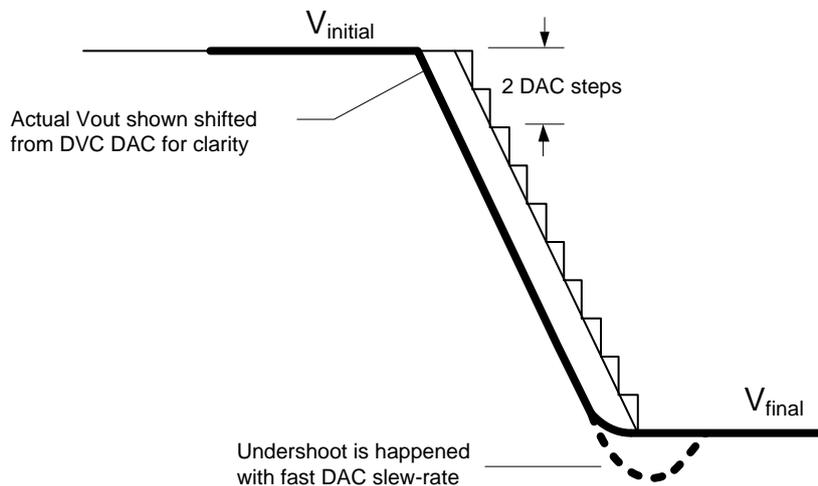
Figure 4: PV88090 DVC down transition measurement example
