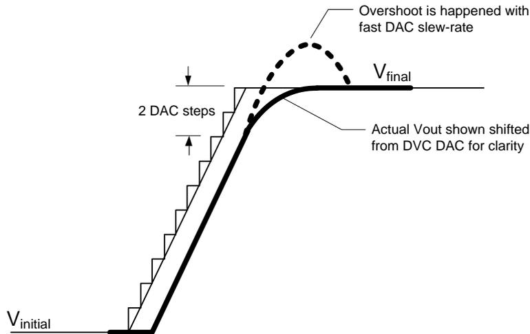
Figure 3: PV88090 DVC up transition measurement example
