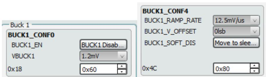
Figure 9: Setting in Dialog GUI\_Sending 0X60 to BUCK1\_CONF0
