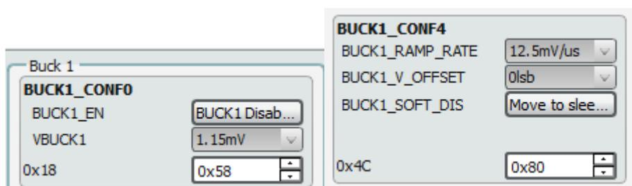
Figure 11: Setting in Dialog GUI\_Sending 0x58 to BUCK1\_CONF0
