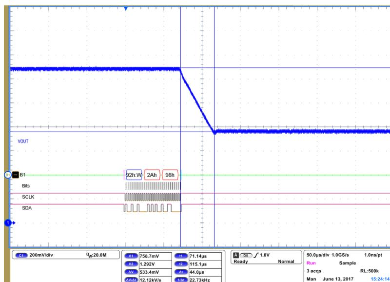
Figure 8: DVC step-down with 12.5mV/µs slew rate
