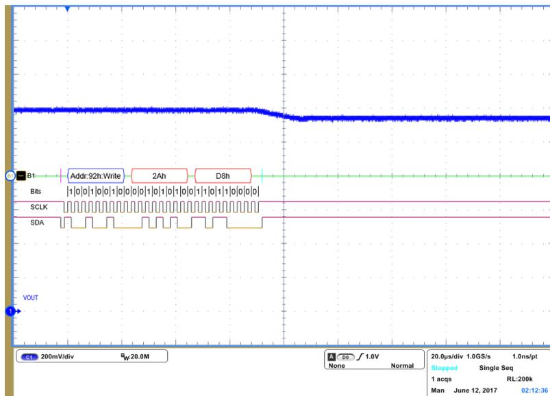
Figure 10: DVC step-down from 1.2V to 1.15V
