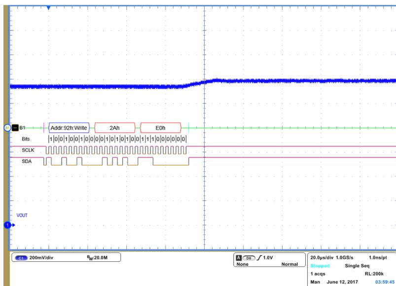
Figure 12: Dynamic Voltage Control step-up from 1.15V to 1.2V
