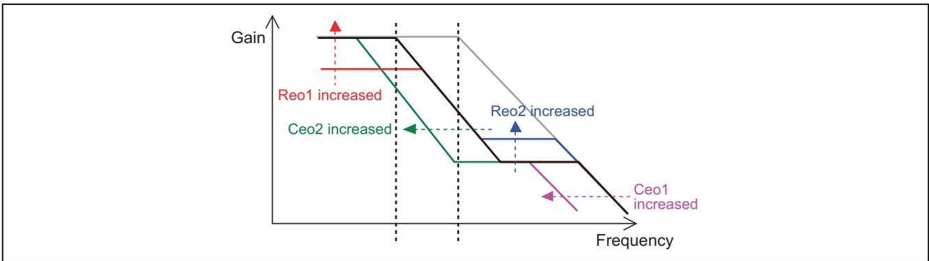
Figure 12 Overview of Gain-Frequency Characteristics
