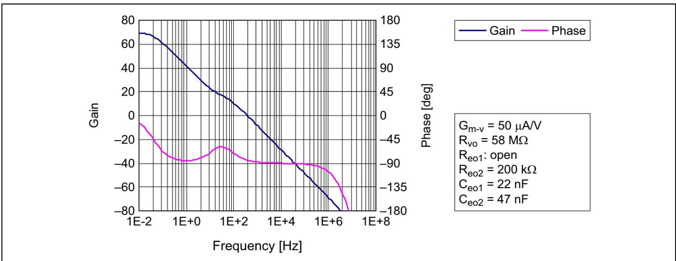
Figure 13 Frequency Characteristics of the Error Amplifier
