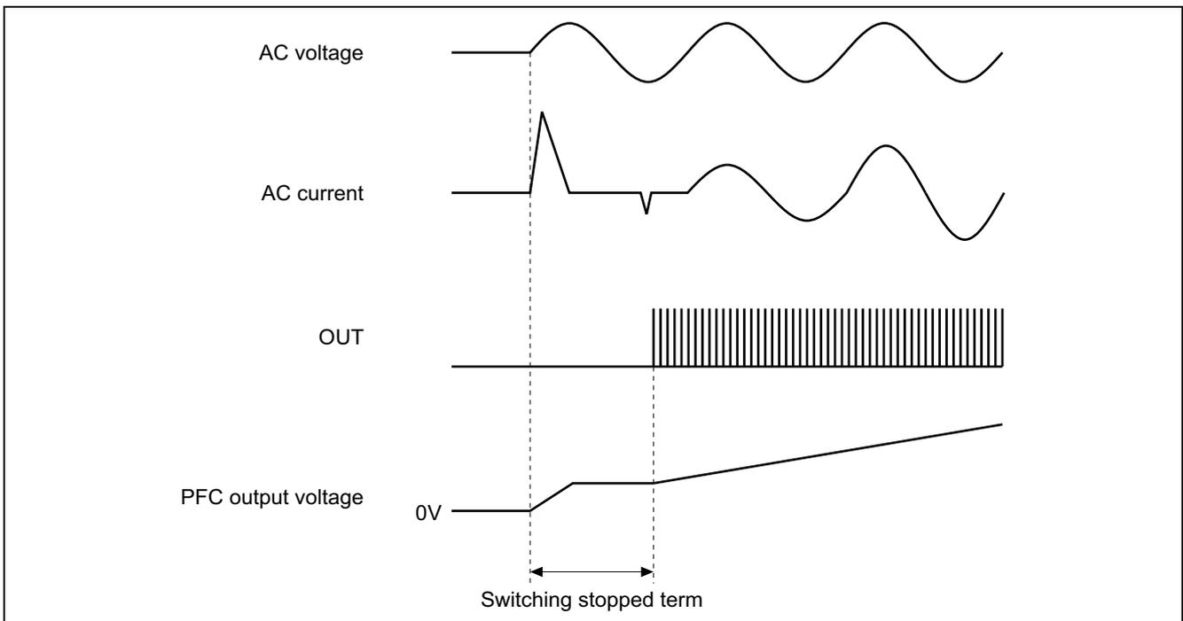
Figure 10 Example(1) Stop of the Switching Operation
