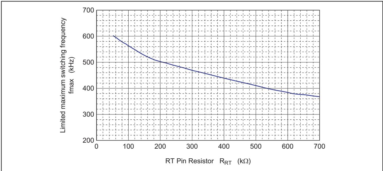
Figure 9 RT Pin Resistor vs. Limited Maximum Switching Frequency
