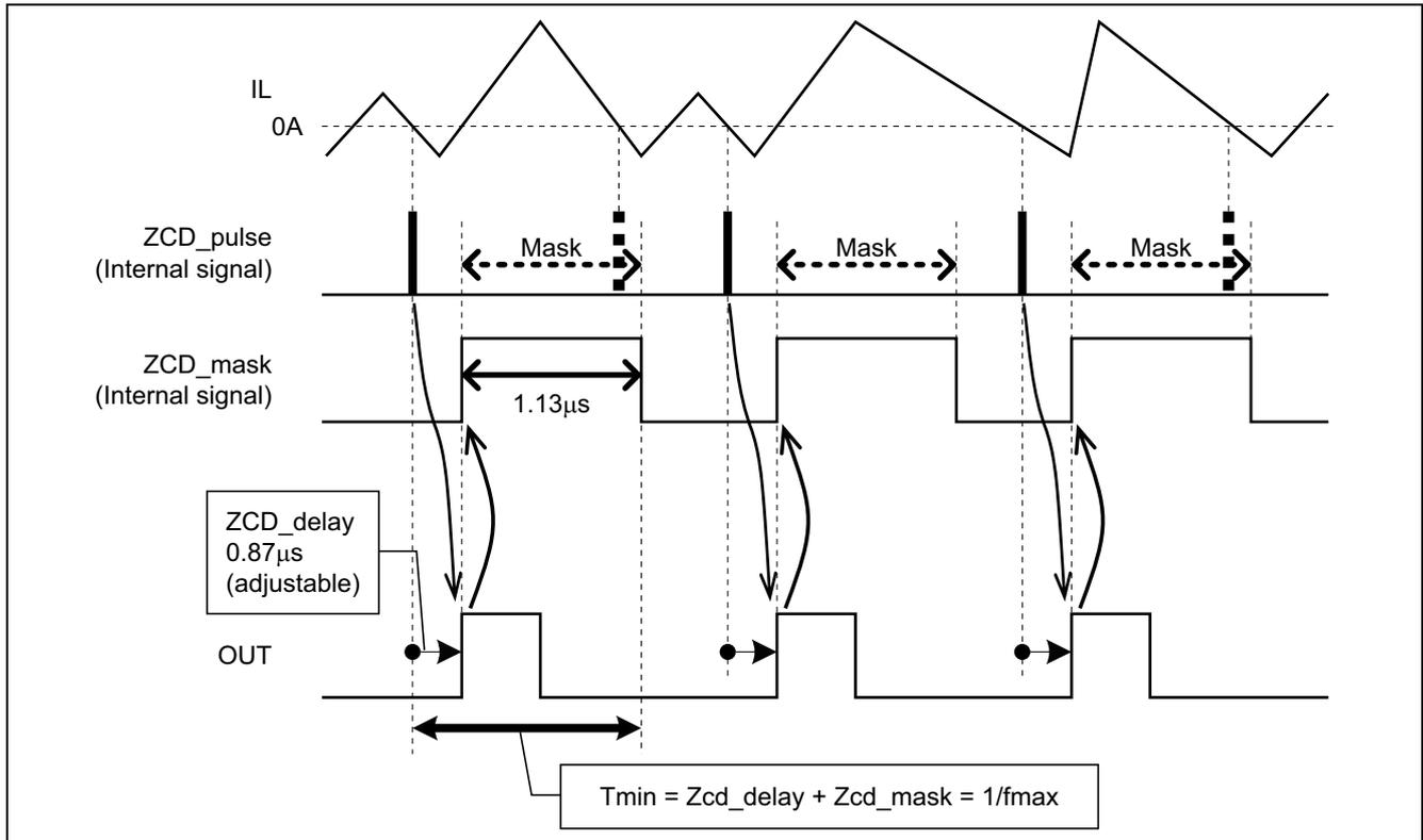
Figure 8 Waveform at Limited Maximum Switching Frequency Operation
