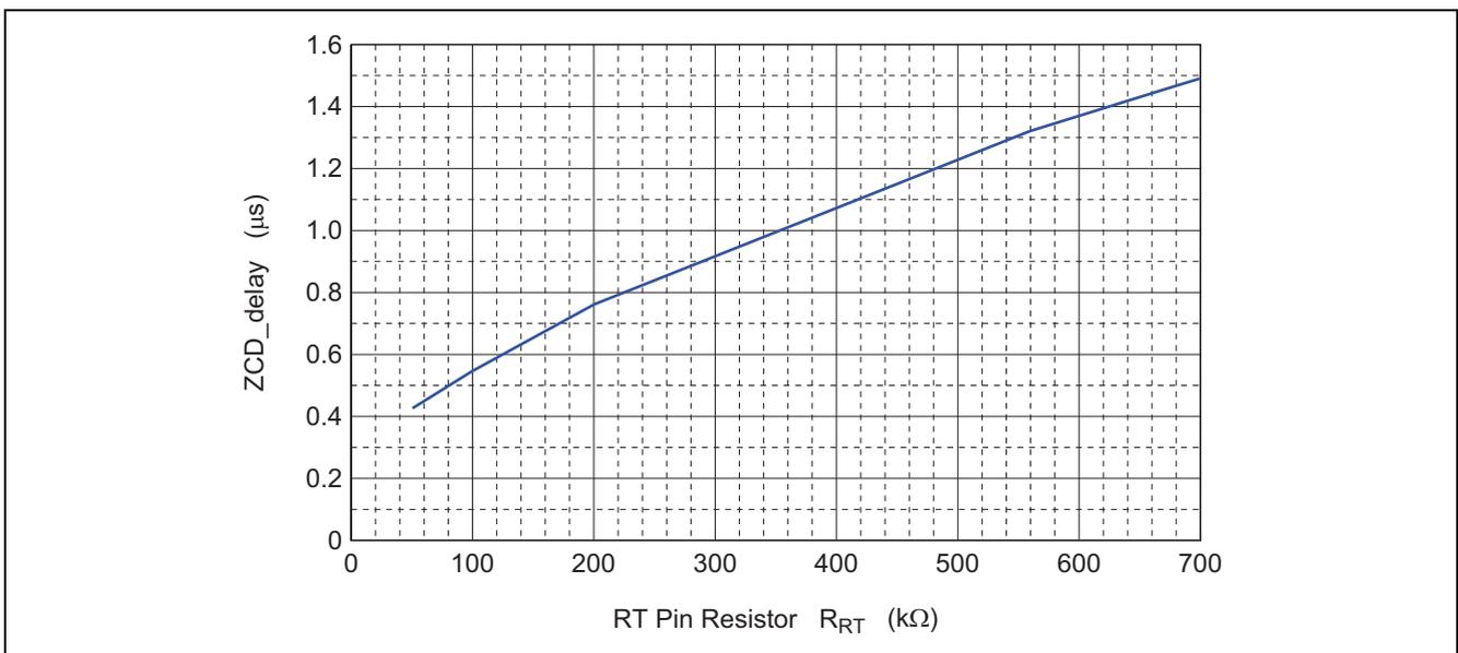
Figure 2 RT Pin Resistor vs. ZCD\_dealy Time
