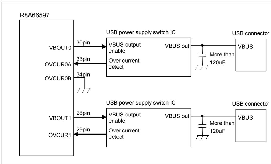
**Figure 6 Example of Host Controller VBUS Power Supply Circuit**
