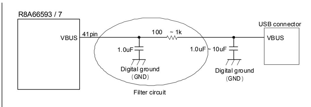
**Figure 7 Example of Peripheral Controller VBUS Power Supply Circuit**
