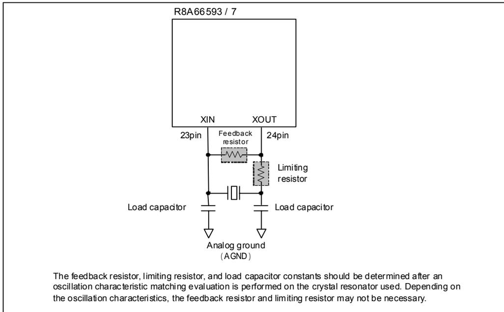
**Figure 4 Example of a Crystal Resonator Connection**
