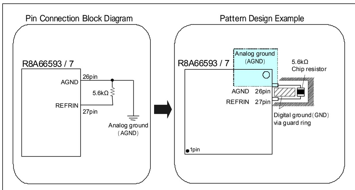
Figure 8 Pin Connection and Design Example of Pattern Around the REFRIN Pin
