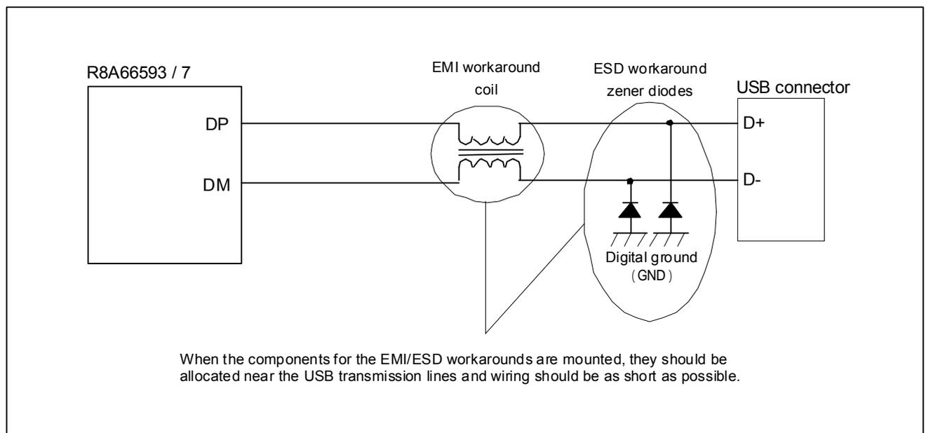
**Figure 9 Connection Example When Components for EMI/ESD Workarounds are Used**
