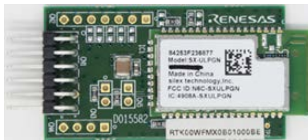
Figure 3. Sillex SX-ULPGN Wi-Fi PMOD Module
