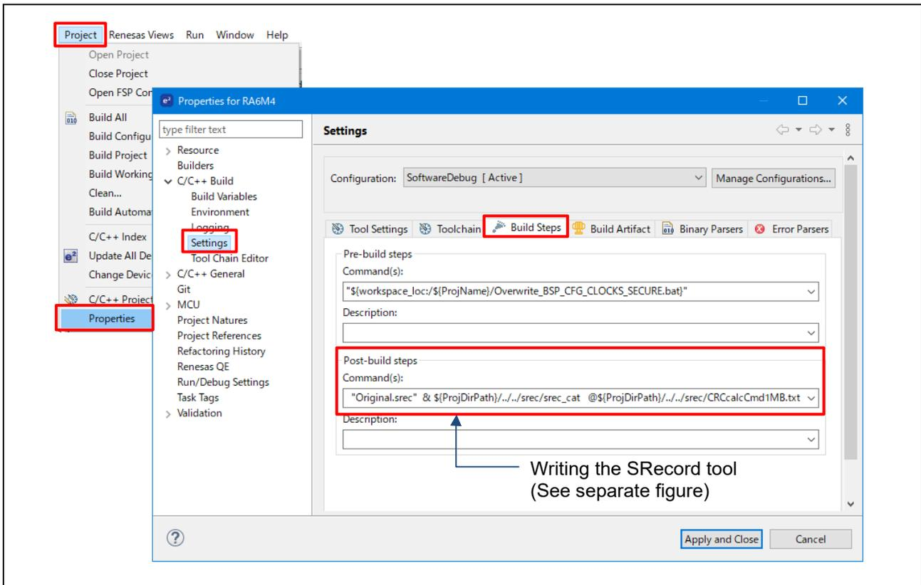
Figure 2.3 Output SRecord File and Start SRecord Tool
