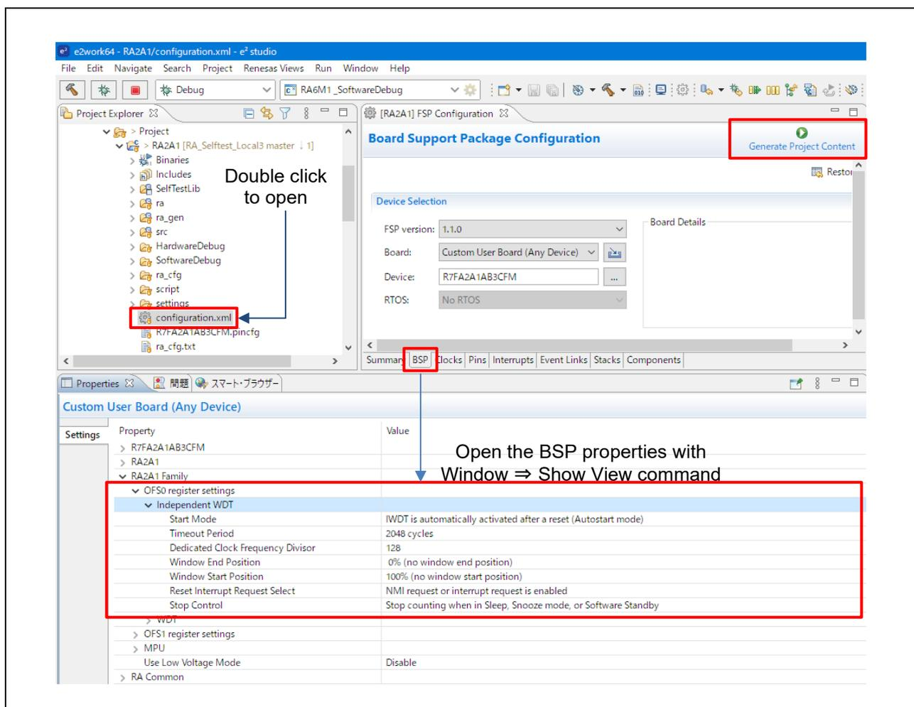
**Figure 2.8 Example of OFS0 Register Setting by Using FSP with e<sup>2</sup> studio**
