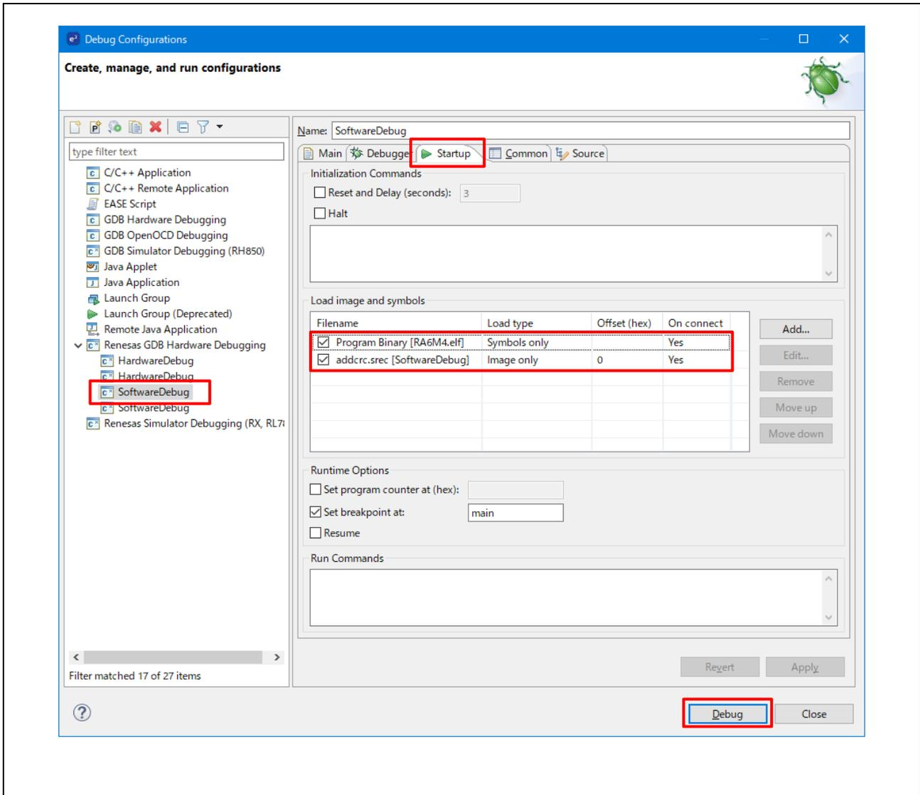
Figure 2.5 Load Image and Symbol Setting Example
