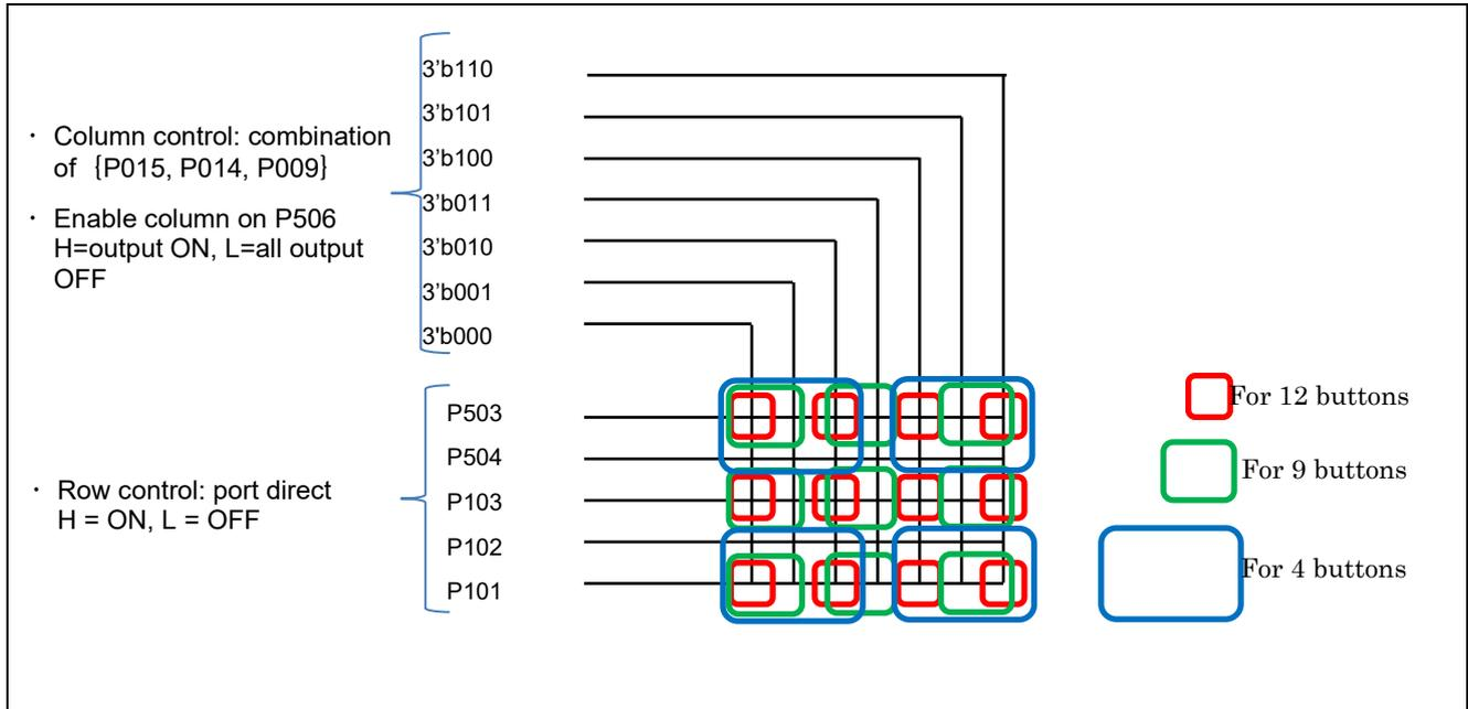
Figure 5.3 Correspondence of LED Control Ports and Each Electrode
