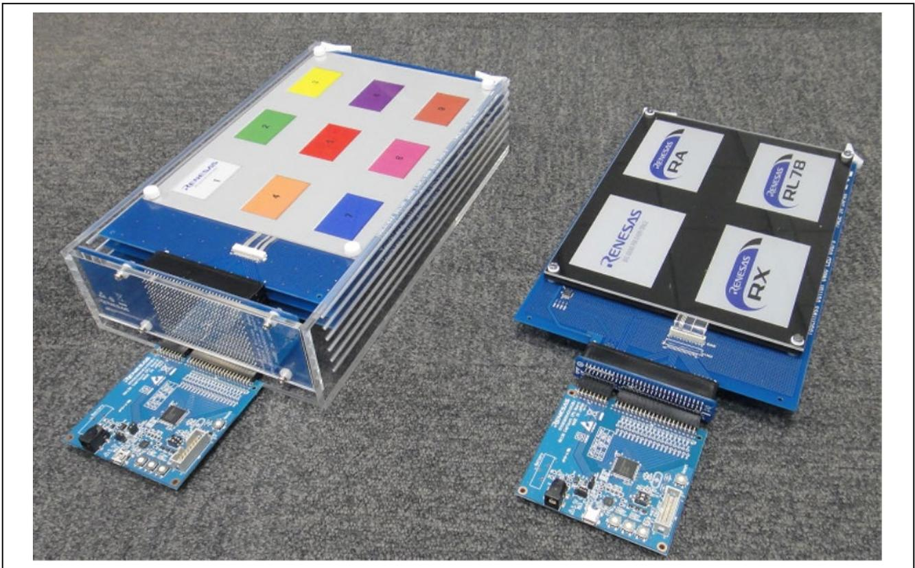
Figure 1.1 Touchless Button Electrode Board (Left: with housing, Right: without housing)
