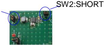
SW2:SHORT | Open SW 2 and SW 3, Connect the + side of the external DC power supply to "3.3V" pin and the - side to "GND" pin.<br><br>
