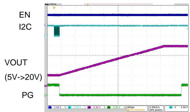
Figure 2.3 VOUT voltage change waveform (Up)
