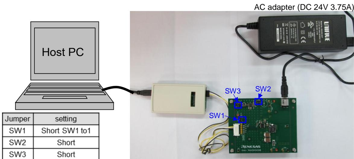
Figure 1.2 RAA230161GSB Evaluation Board connection example (using the AC adapter)
