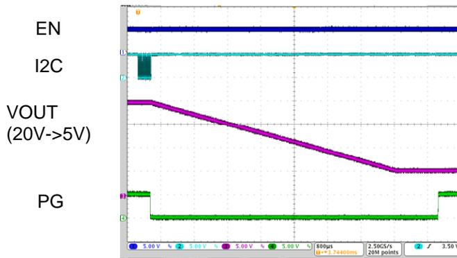
Figure 2.4 VOUT change waveform (Down)
