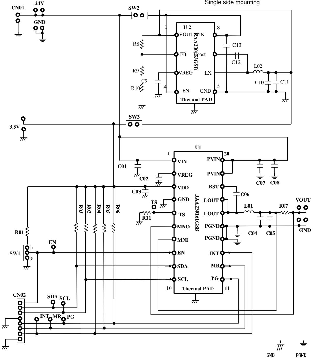
Figure 3.1 RAA230161GSB Evaluation Board circuit diagram
