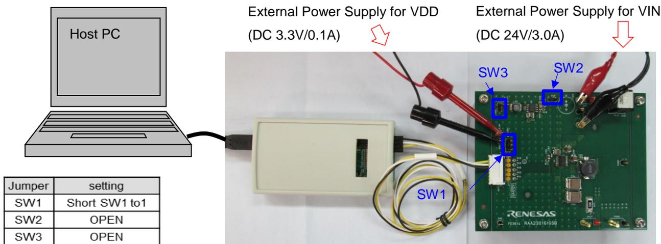
Figure 1.3 RAA230161GSB Evaluation Board connection example (using the external power supplies)
