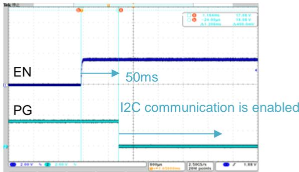
Figure 2.1 I2C communication available timing
