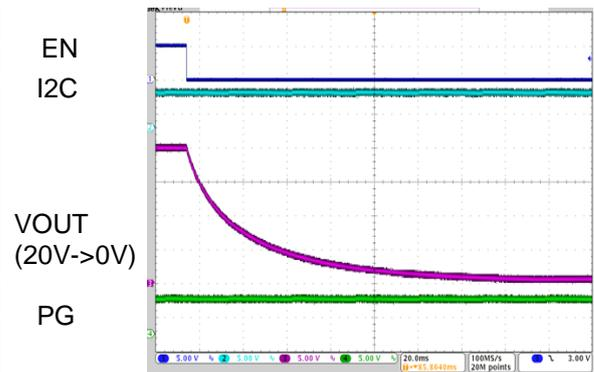
Figure 2.6 VOUT stop waveform (EN control)
