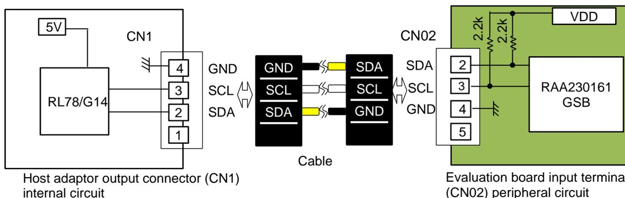
Figure 1.5 RTK0EF0029Z00001BJ CN1 internal circuit
