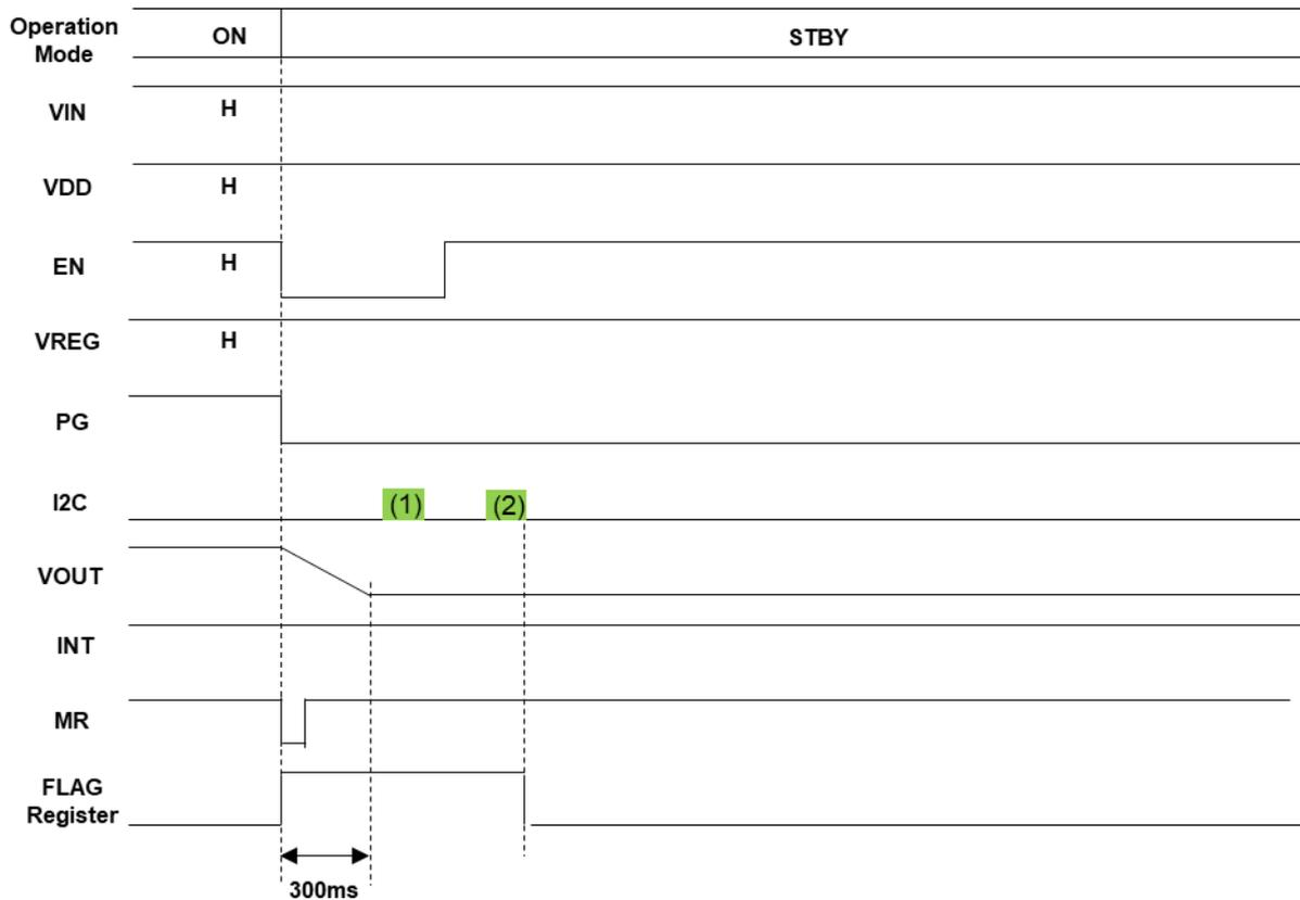
Figure 2.5 Protection function 2 (WDT detect)
