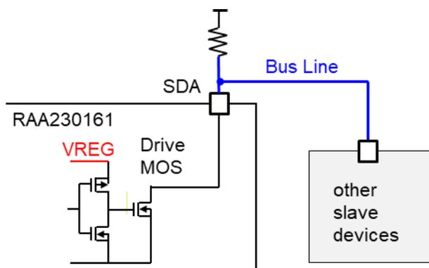
Figure 1.4 Internal circuit of the SDA terminal
