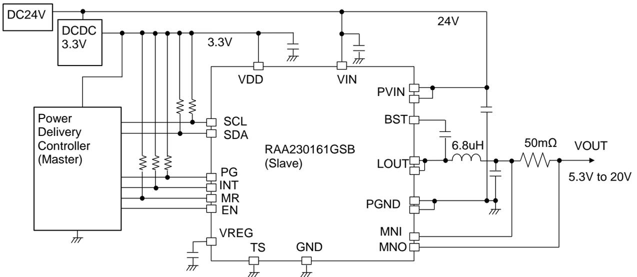
Figure 1.1 Connection of power supply system
