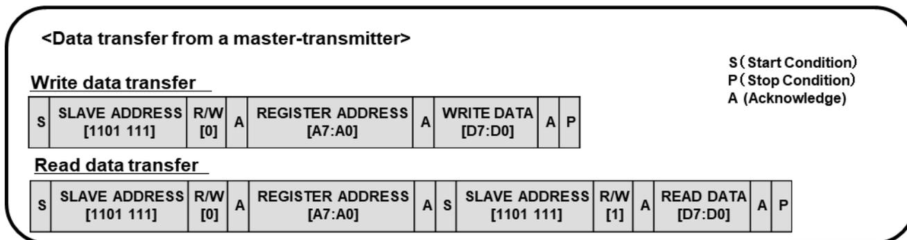
Figure 1.2 I2C Data transfer format
