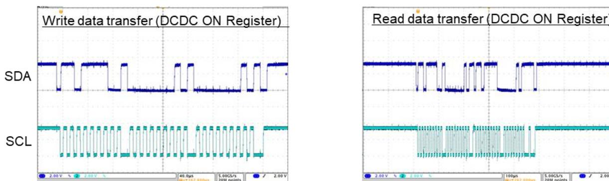
Figure 1.3 I2C reference waveform
