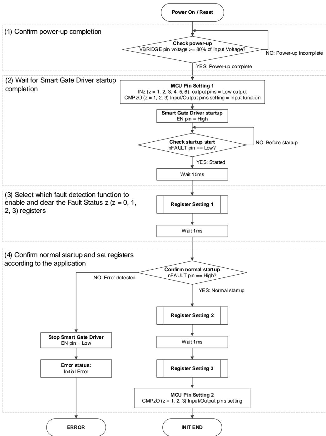
Figure 3-1 Smart Gate Driver Start-up Sequence Example
