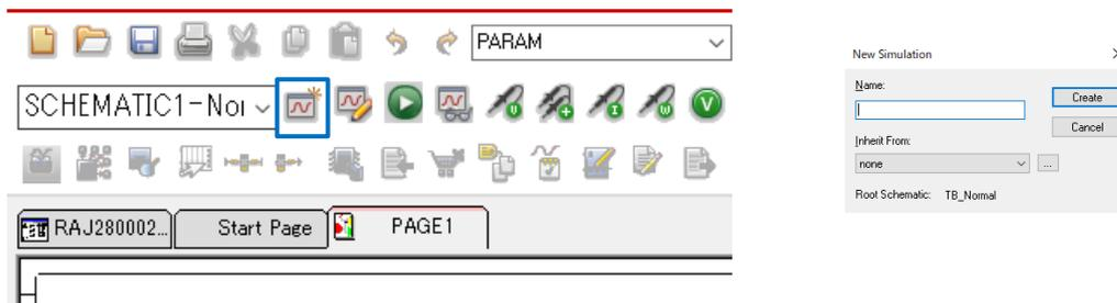
Figure.4 New simulation button and window
