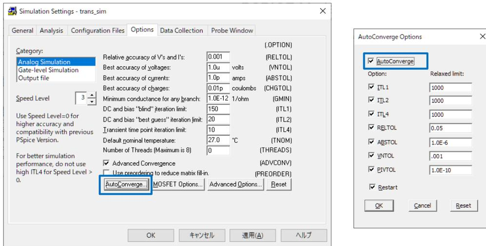
Figure. 13 Simulation settings screen (Location of “AutoConverge”)
