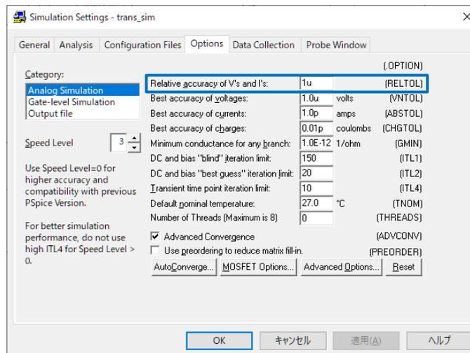
Figure. 14 Simulation settings screen (Where to adjust accuracy)
