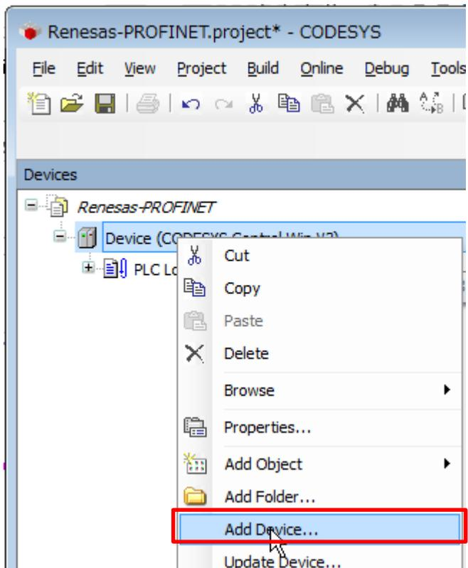
The "Add Device" dialog box opens. Select "Ethernet" under "Fieldbusses", "Profinet IO", then "Ethernet Adapter" and click on the "Add Device" button.
