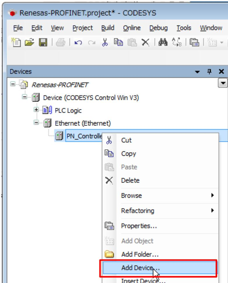
The "Add Device" dialog box opens. Select "Renesas\_PROFNET\_Device" under "Fieldbusses", "Profinet IO", then "Profinet IO Slave" and click on the "Add Device" button.
