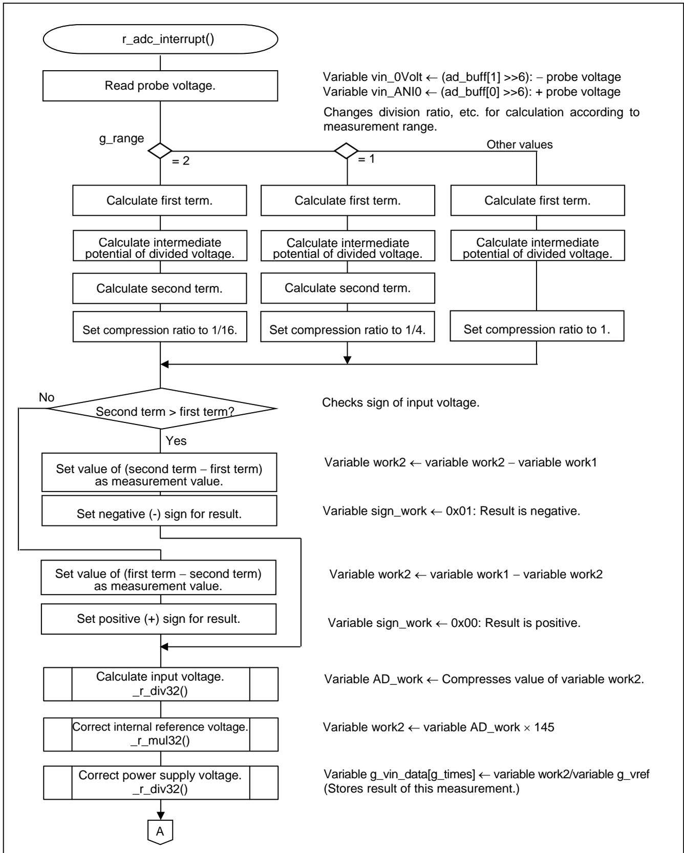
Figure 5.33 A/D Conversion End Interrupt Processing (1/2)
