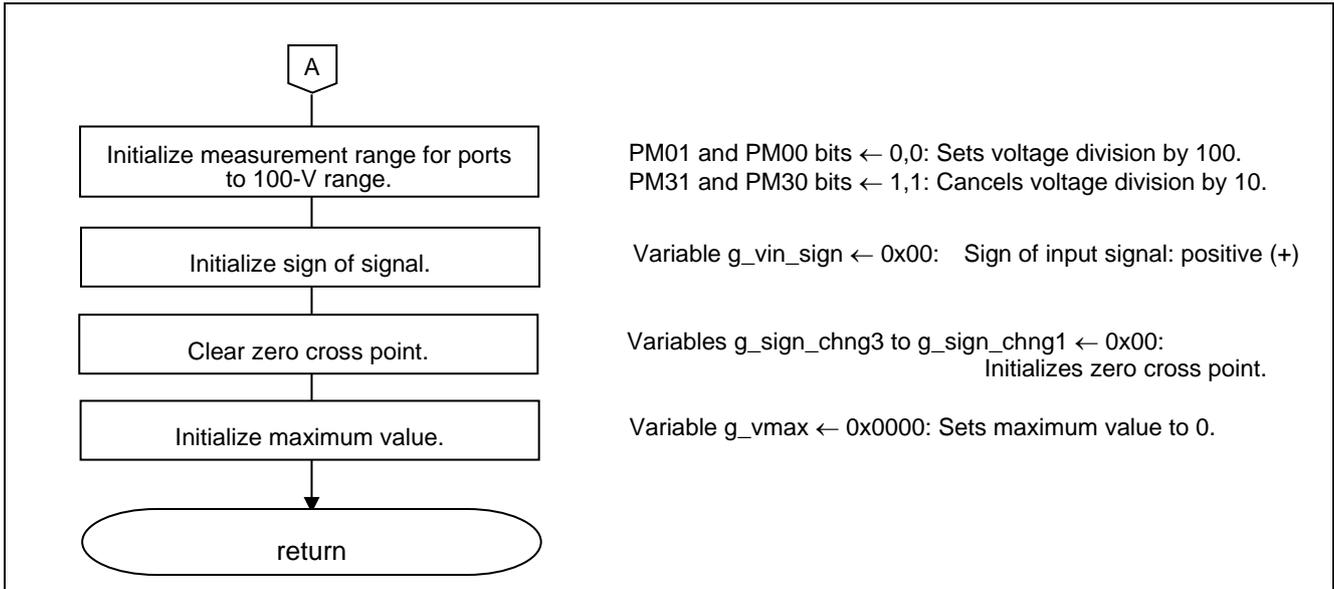
Figure 5.29 Checking Internal Reference Voltage (2/2)
