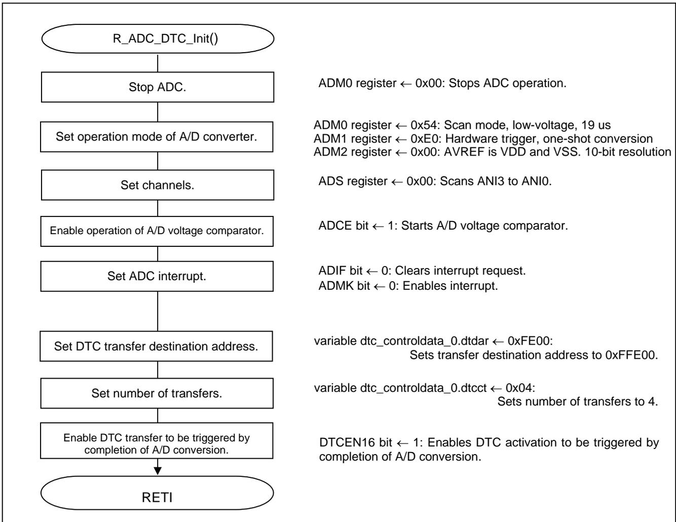
Figure 5.31 Setting ADC and DTC
