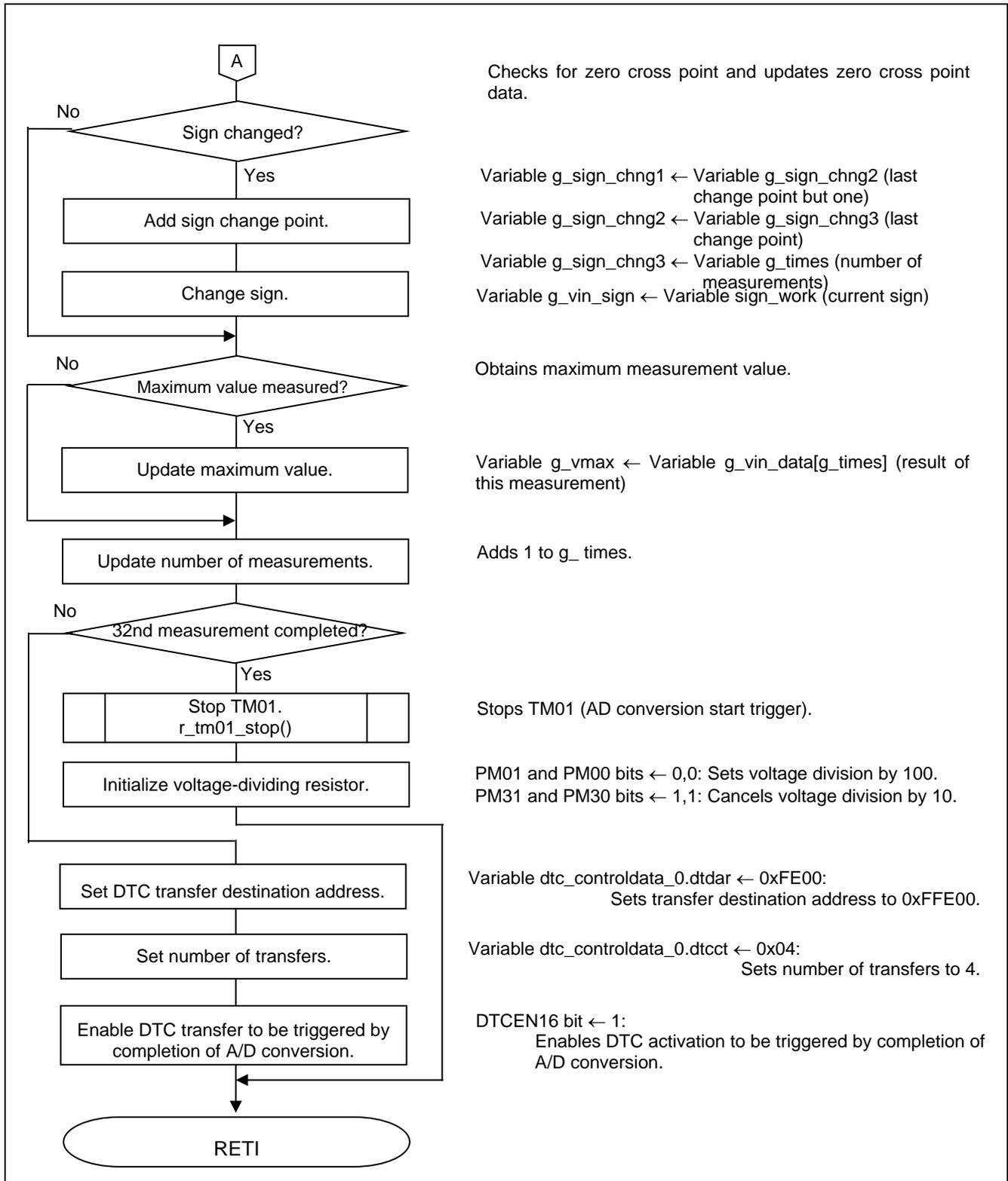
Figure 5.34 A/D Conversion End Interrupt Processing (2/2)
