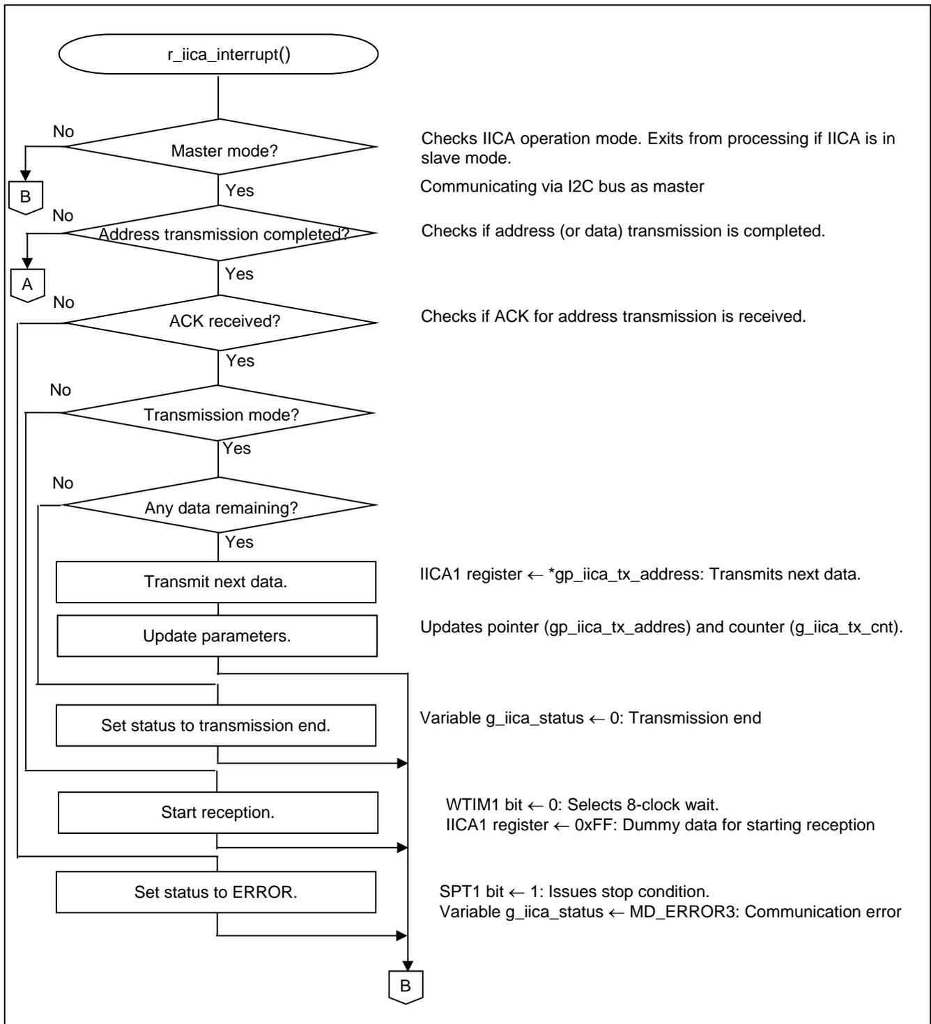
Figure 5.35 I2C Communication End Interrupt Processing (1/2)
