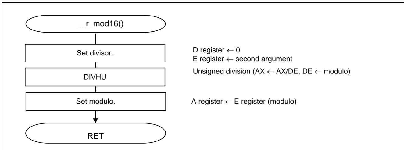
Figure 5.40 16-Bit Modulo Operation
