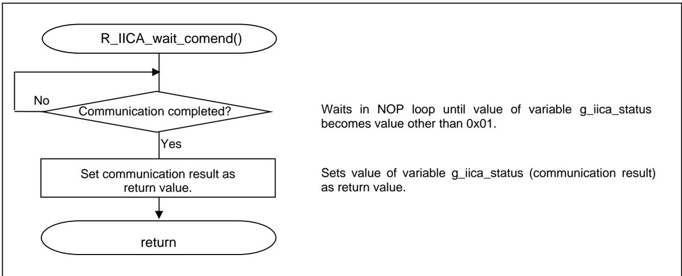
Figure 5.23 Waiting for Completion of I2C Communication
