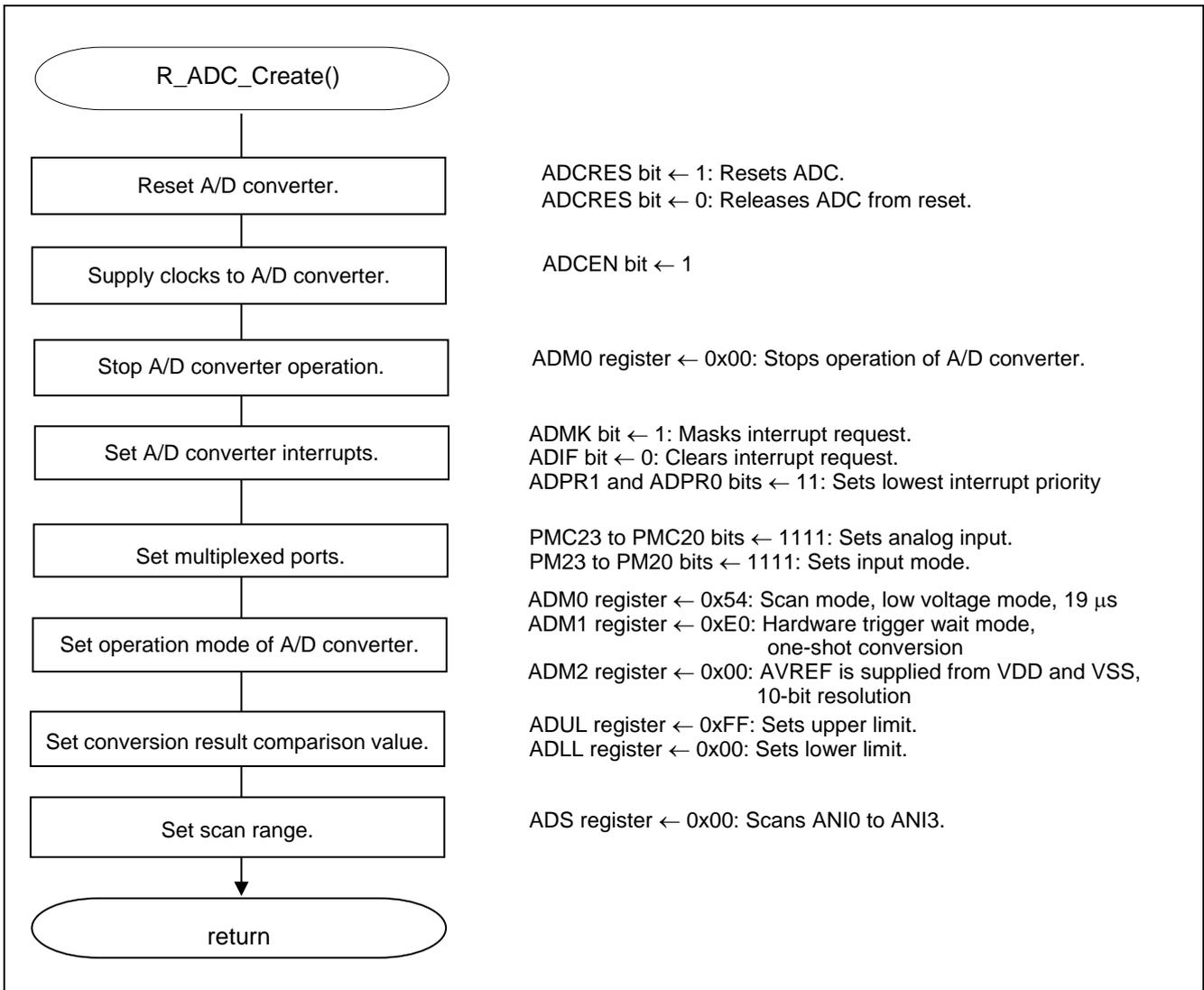
Figure 5.9 Setting A/D Converter
