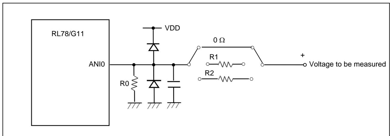
Figure 1.1 Analog Voltage Input Circuit
