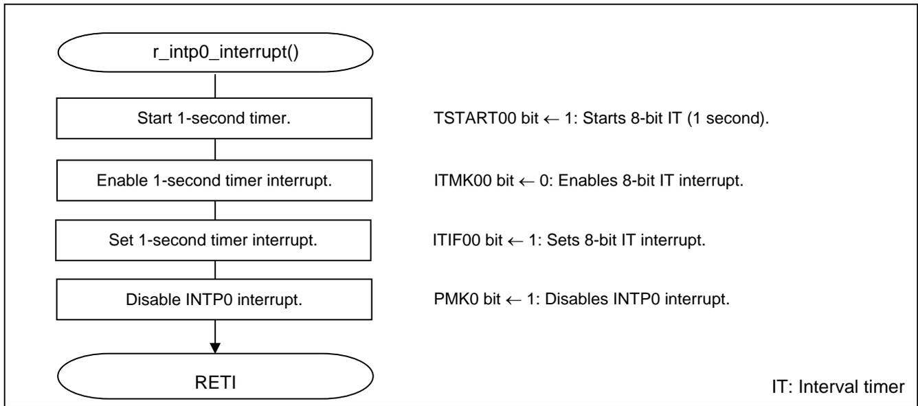
Figure 5.26 INTP0 Interrupt Processing
