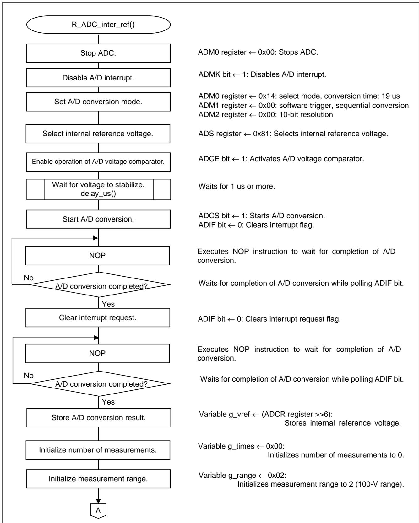
Figure 5.28 Checking Internal Reference Voltage (1/2)
