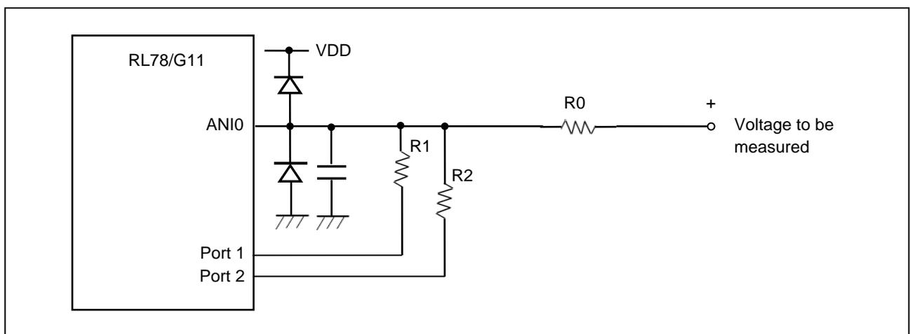
Figure 1.3 Automatic Measurement Range Switching
