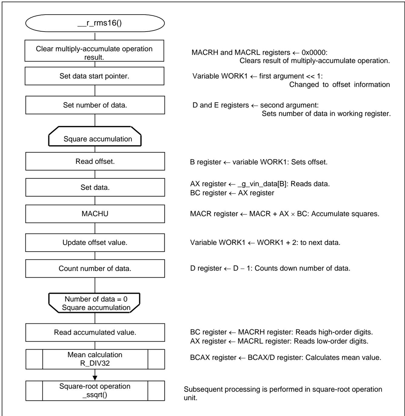
Figure 5.41 Root-Mean-Square Calculation for 16-Bit Data
