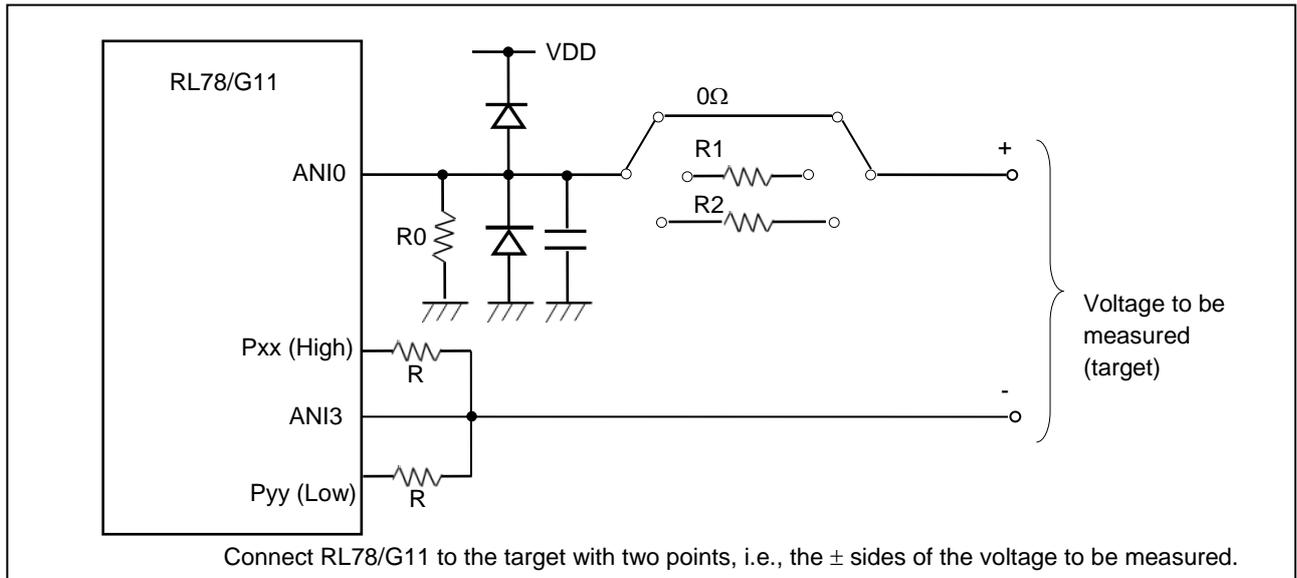
Figure 1.2 Handling Negative Voltage
