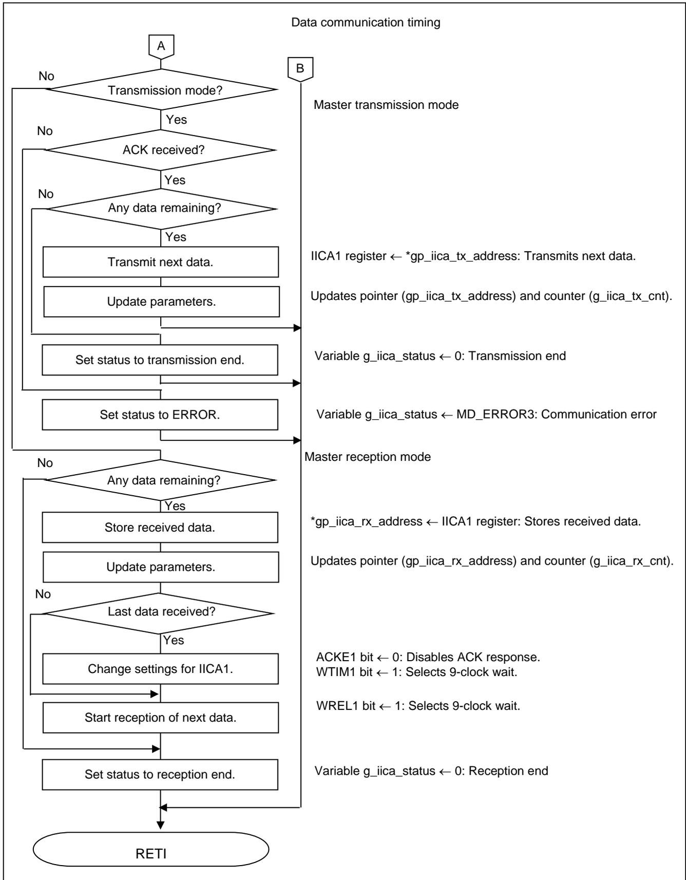
Figure 5.36 I2C Communication End Interrupt Processing (2/2)
