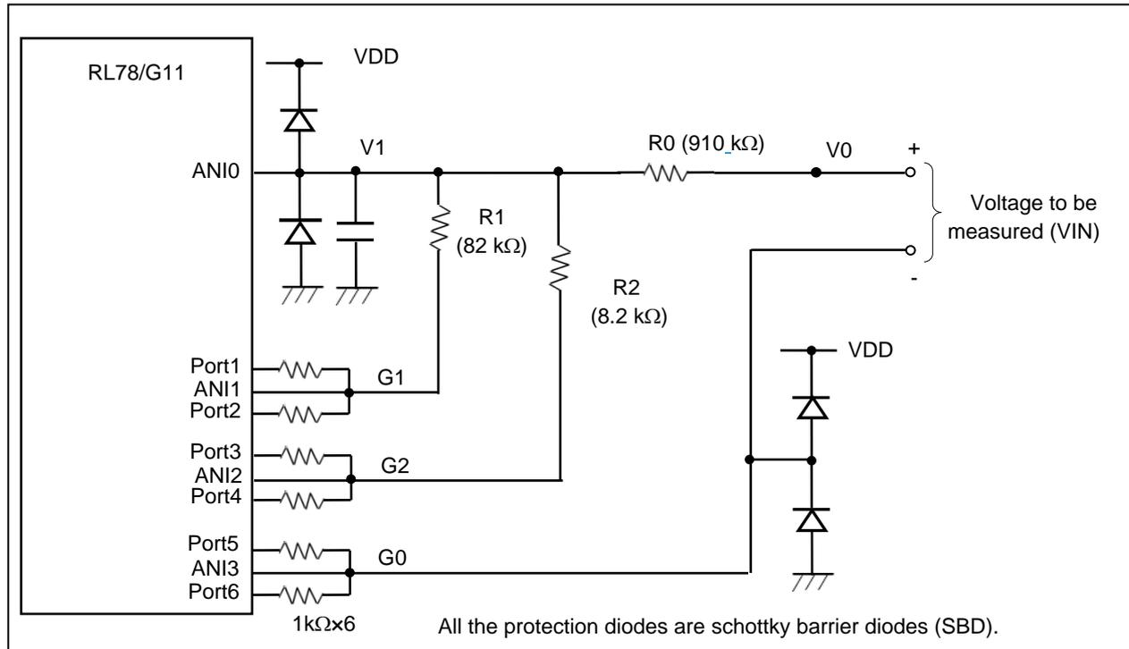
Figure 1.4 Measurement Circuit
