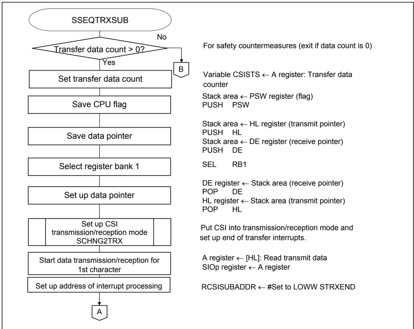
**Figure 5.33 Continuous Transmission/Reception Startup Processing (1/2)**
