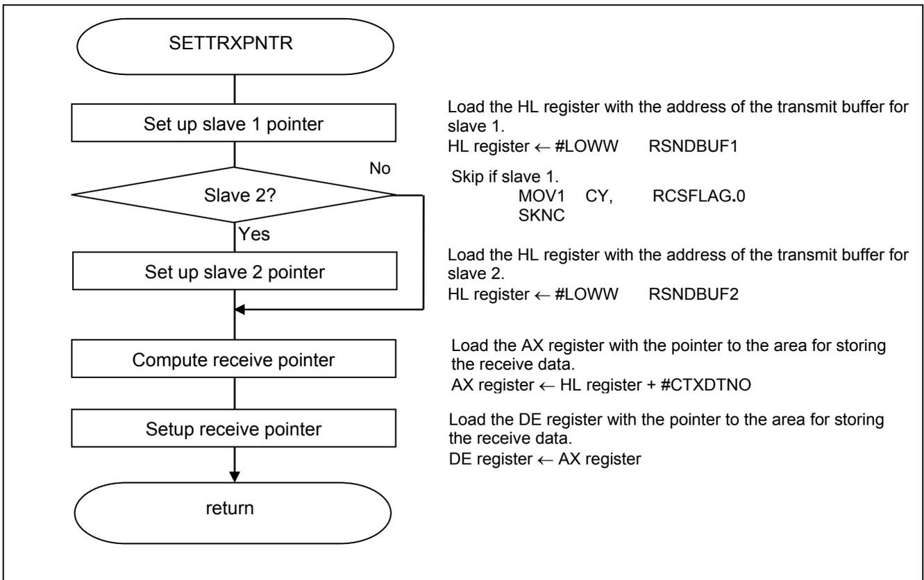
**Figure 5.25 Data Pointer Setup Processing**
