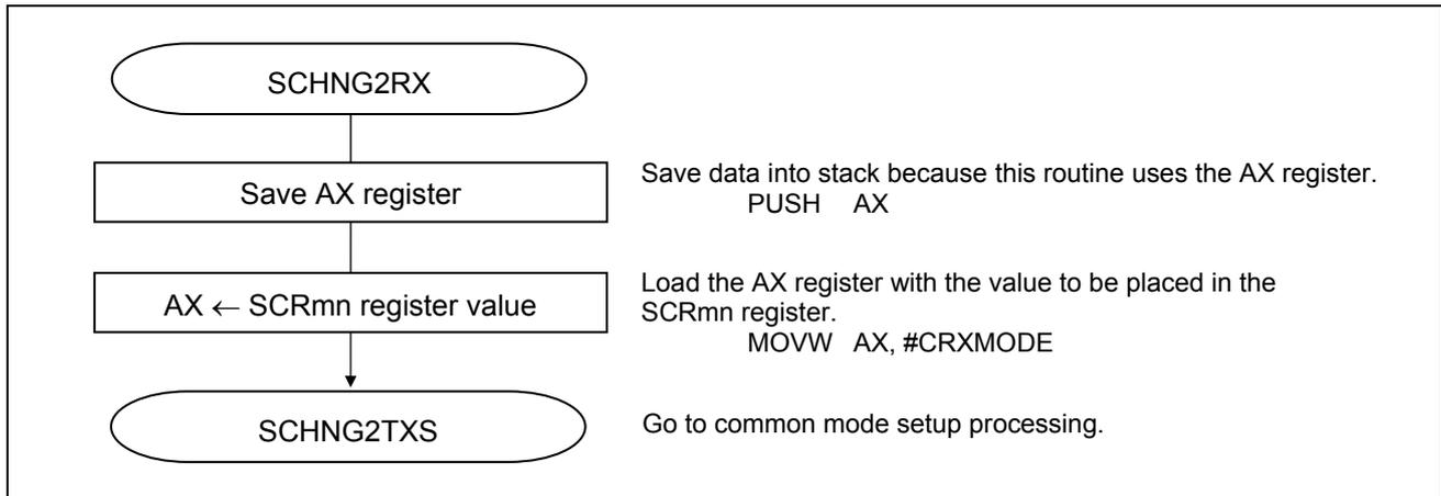
**Figure 5.39 Reception Mode Setup Processing**
