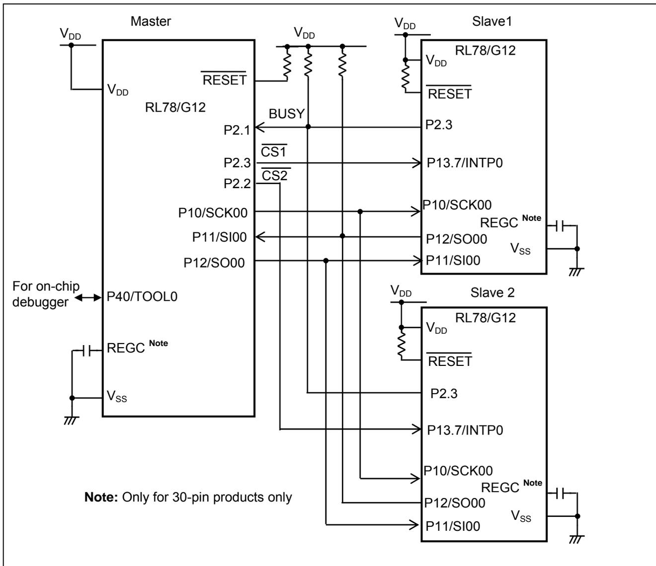
**Figure 4.1 Hardware Configuration**
