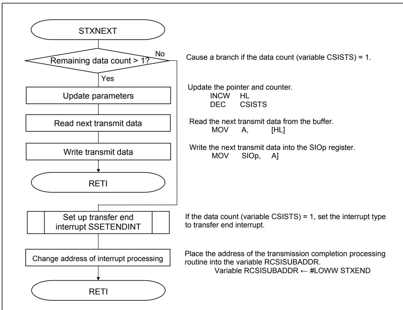
**Figure 5.46 Buffer Empty Interrupt Processing (Continuous Transmission Mode)**
