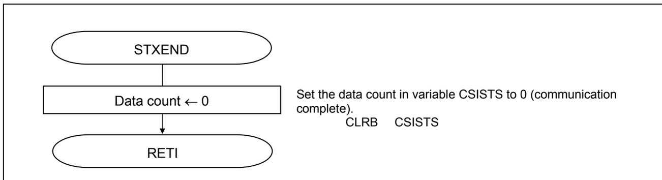
**Figure 5.47 Transmission End Interrupt Processing (Continuous Transmission Mode)**
