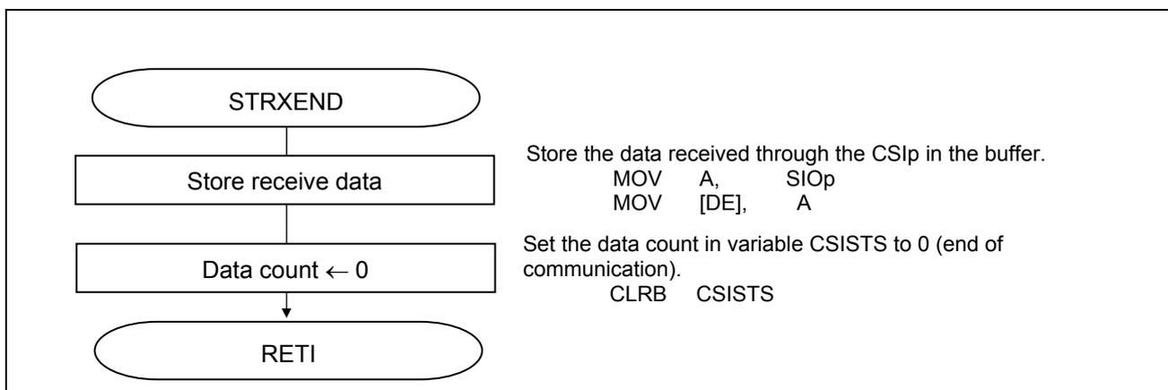
**Figure 5.49 Transfer End Interrupt Processing (Continuous Transmission/Reception Mode)**
