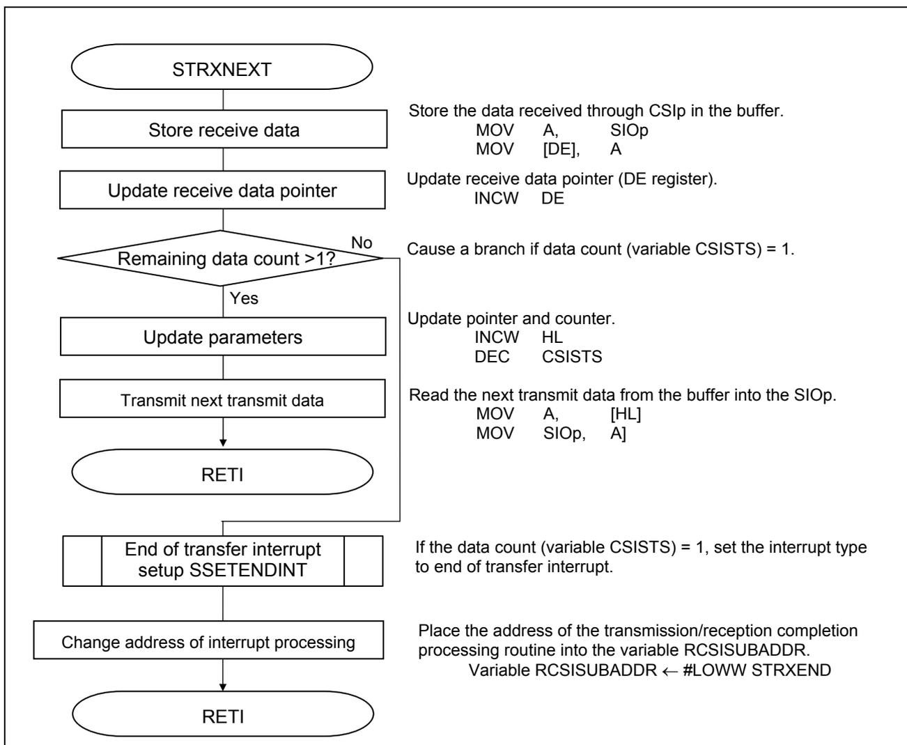
**Figure 5.48 Buffer Empty Interrupt Processing (Continuous Transmission Mode)**
