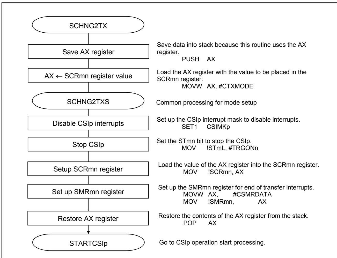
**Figure 5.38 Transmission Mode Setup Processing**
