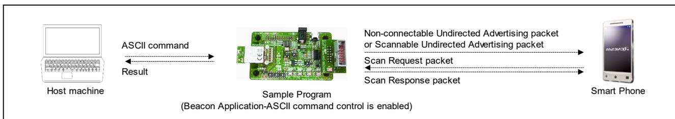
The Beacon Application-ASCII command control is executed when power is supplied from the DC jack (J1) or USB interface (CN3) of the evaluation board that contains the sample program firmware. The evaluation board waits for a control command from the host machine.
