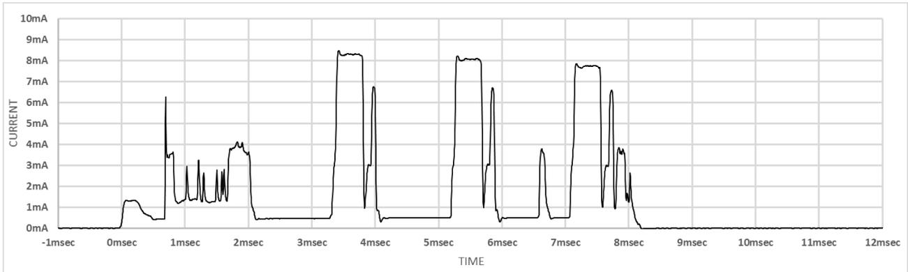
**Figure 9-16** Current Consumption Waveform of ADV\_SCAN\_IND at MCU Clock Frequency 16MHz
