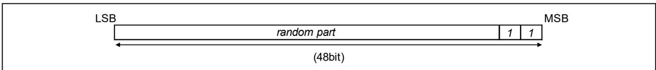
Figure 9-23 Static Device Address format
