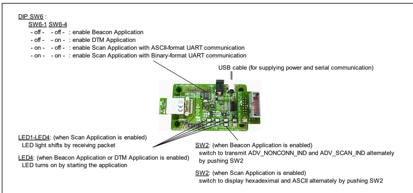
**Figure 4-2 Board Operating for Confirming Operation of the Sample Program**
