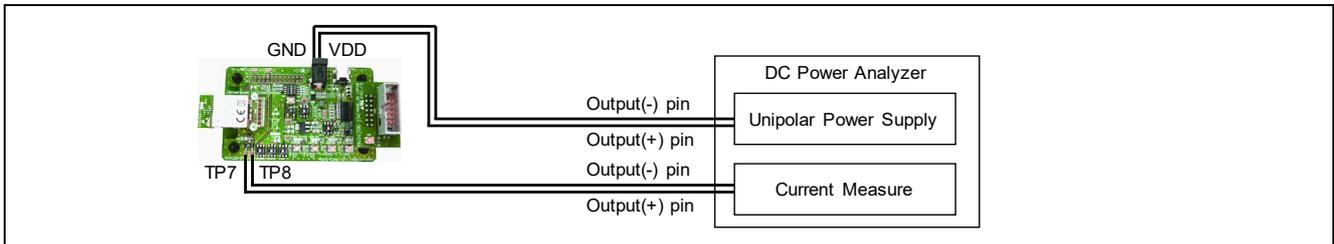
**Figure 9-1 Current Consumption Measurement Environment**
