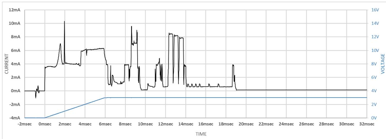
**Figure 9-4 Current Waveform of Starting-up Beacon Stack at MCU Clock Frequency 16MHz**
