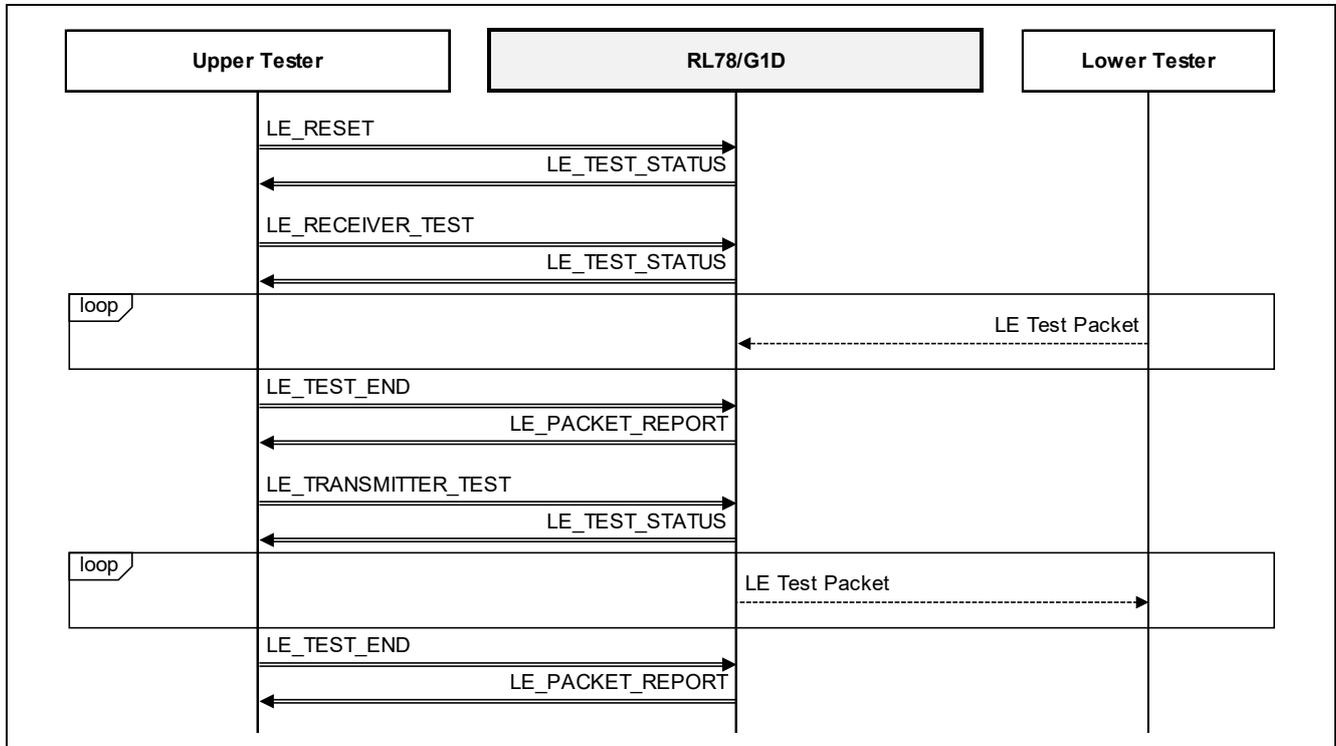
Figure 5-5 2-wire UART Direct Test Mode communication sequence
