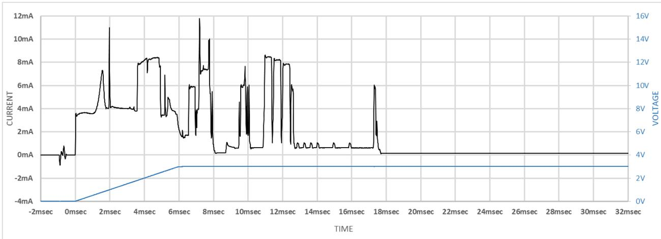
**Figure 9-5 Current Waveform of Starting-up Beacon Stack at MCU Clock Frequency 32MHz**
