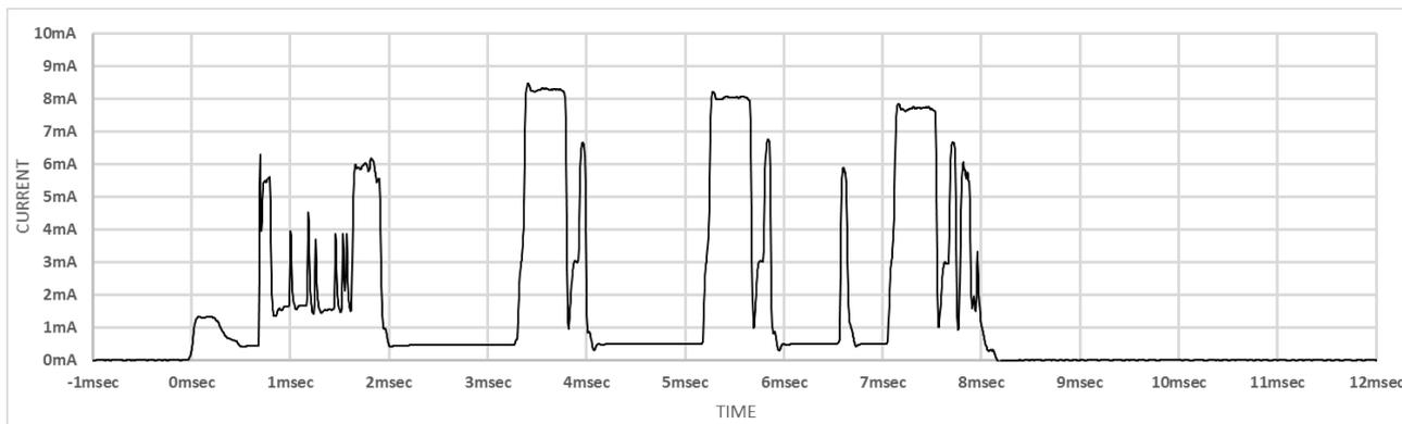
**Figure 9-20** Current Consumption Waveform of ADV\_SCAN\_IND at MCU Clock Frequency 32MHz
