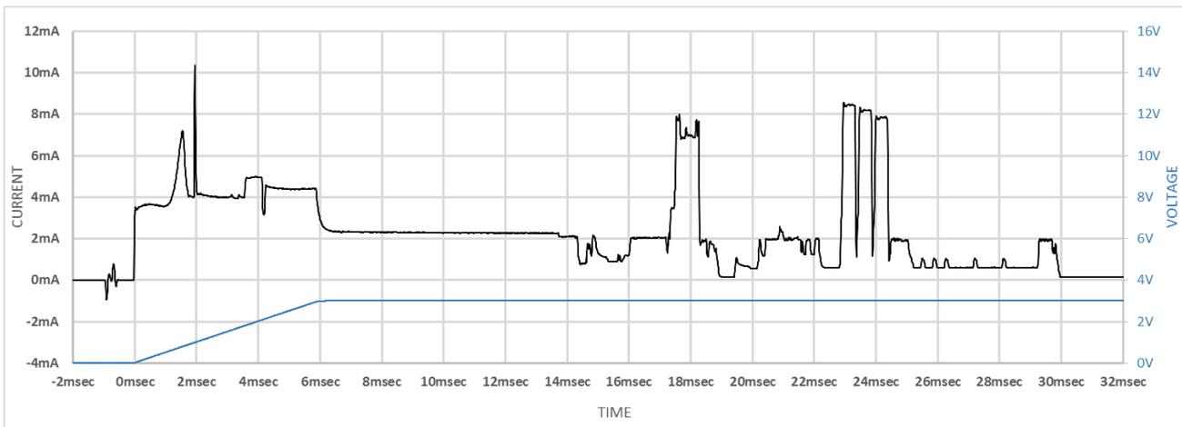
Figure 9-2 Current Waveform of Starting-up Beacon Stack at MCU Clock Frequency 4MHz
