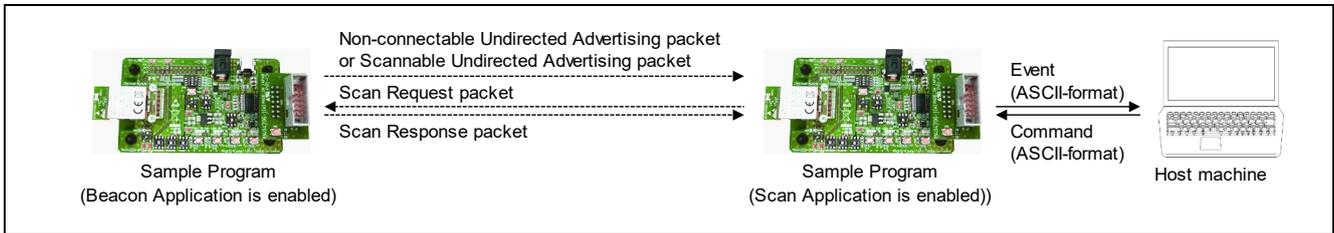
To run Beacon Application, switch both DIP switch SW6 position-1 and position-4 to OFF, and supply power via DC jack (J1) or USB interface (CN3). Similarly, to run Scan Application, switch DIP switch SW6 position-1 to ON and position-4 to OFF, and supply power via USB interface from Host machine.
