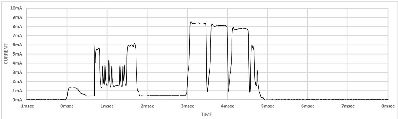
**Figure 9-18** Current Consumption Waveform of ADV\_NONCONN\_IND at MCU Clock Frequency 32MHz (not use DC-DC converter)
