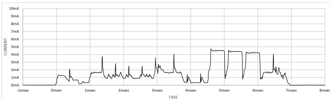
**Figure 9-7** Current Consumption Waveform of ADV\_NONCONN\_IND at MCU Clock Frequency 4MHz (use DC-DC converter)
