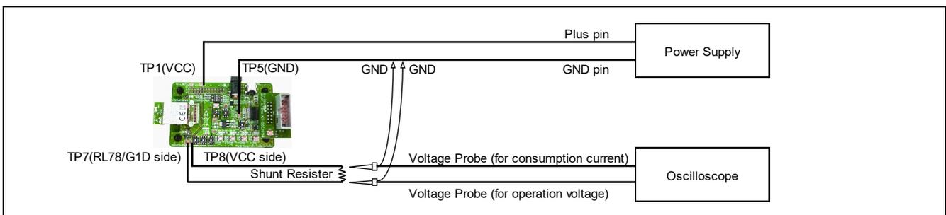
**Figure 4-4 Measurement Environment which uses the combination of Shunt Resistor and Voltage Probe**
