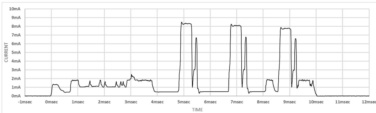
**Figure 9-8** Current Consumption Waveform of ADV\_SCAN\_IND at MCU Clock Frequency 4MHz
