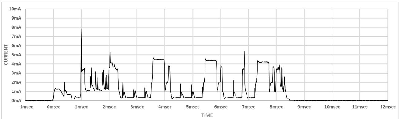
**Figure 9-17** Current Consumption Waveform of ADV\_SCAN\_IND at MCU Clock Frequency 16MHz
