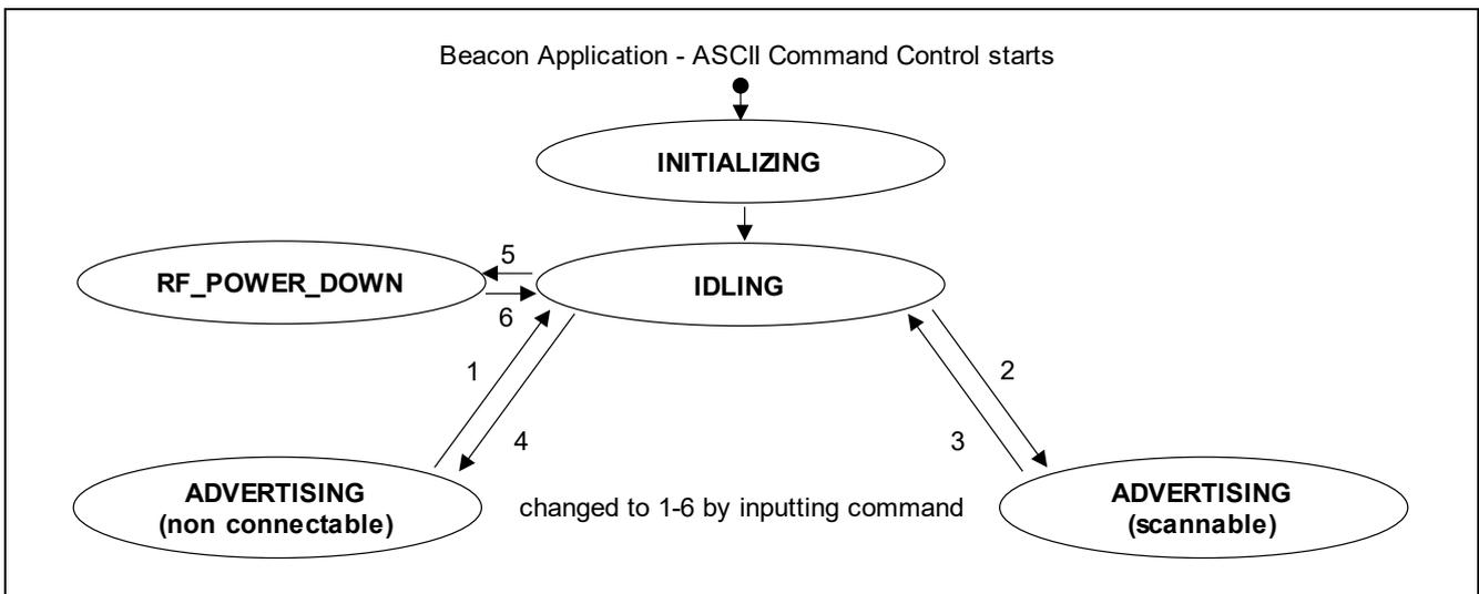
Figure 8-4 State Transition of Beacon Application-ASCII command control
