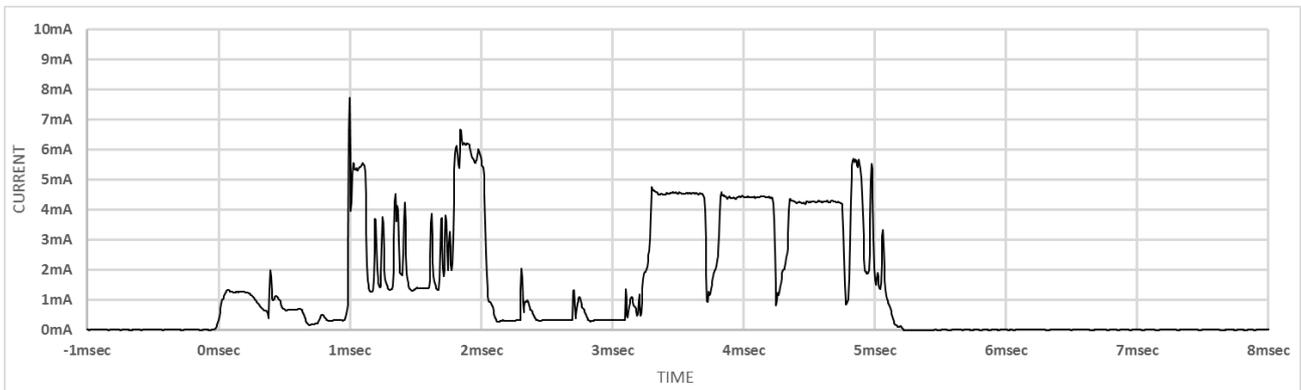
**Figure 9-19** Current Consumption Waveform of ADV\_NONCONN\_IND at MCU Clock Frequency 32MHz (use DC-DC converter)
