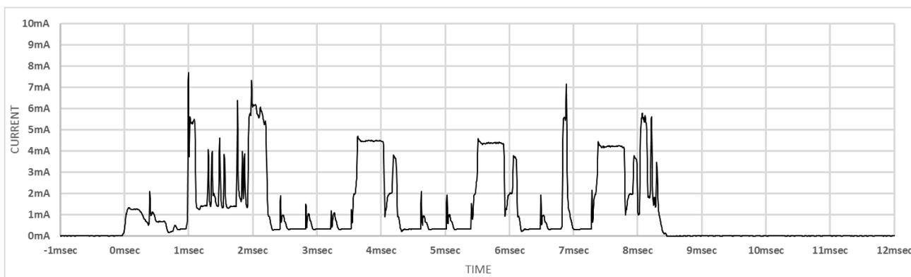
**Figure 9-21** Current Consumption Waveform of ADV\_SCAN\_IND at MCU Clock Frequency 32MHz
