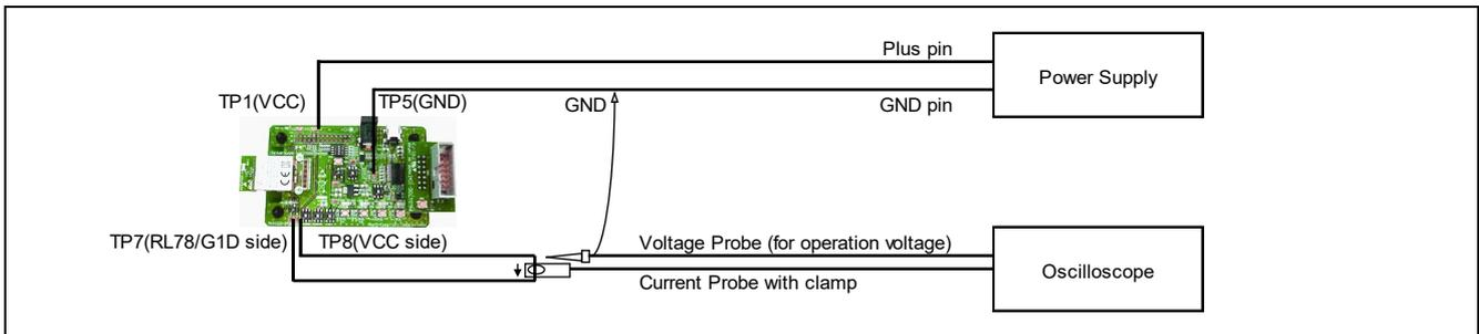
**Figure 4-3 Measurement Environment which uses Current Probe**
