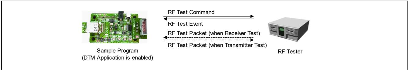
To run DTM Application, switch DIP switch SW6 position-1 to OFF and position-4 to ON, and supply power through DC jack (J1) or USB interface (CN3). DTM Application executes Direct Test Mode by receiving RF Test commands through UART. By connecting RL78/G1D Evaluation Board to RF Tester, it is possible to evaluate RF characteristic of RL78/G1D.
