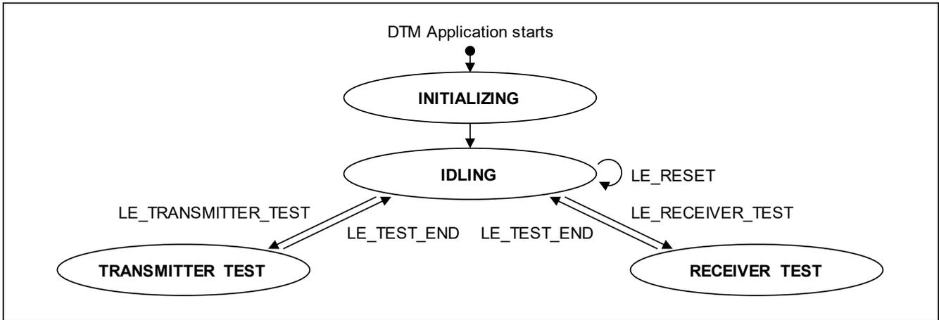
Figure 8-3 State Transition of DTM Application
