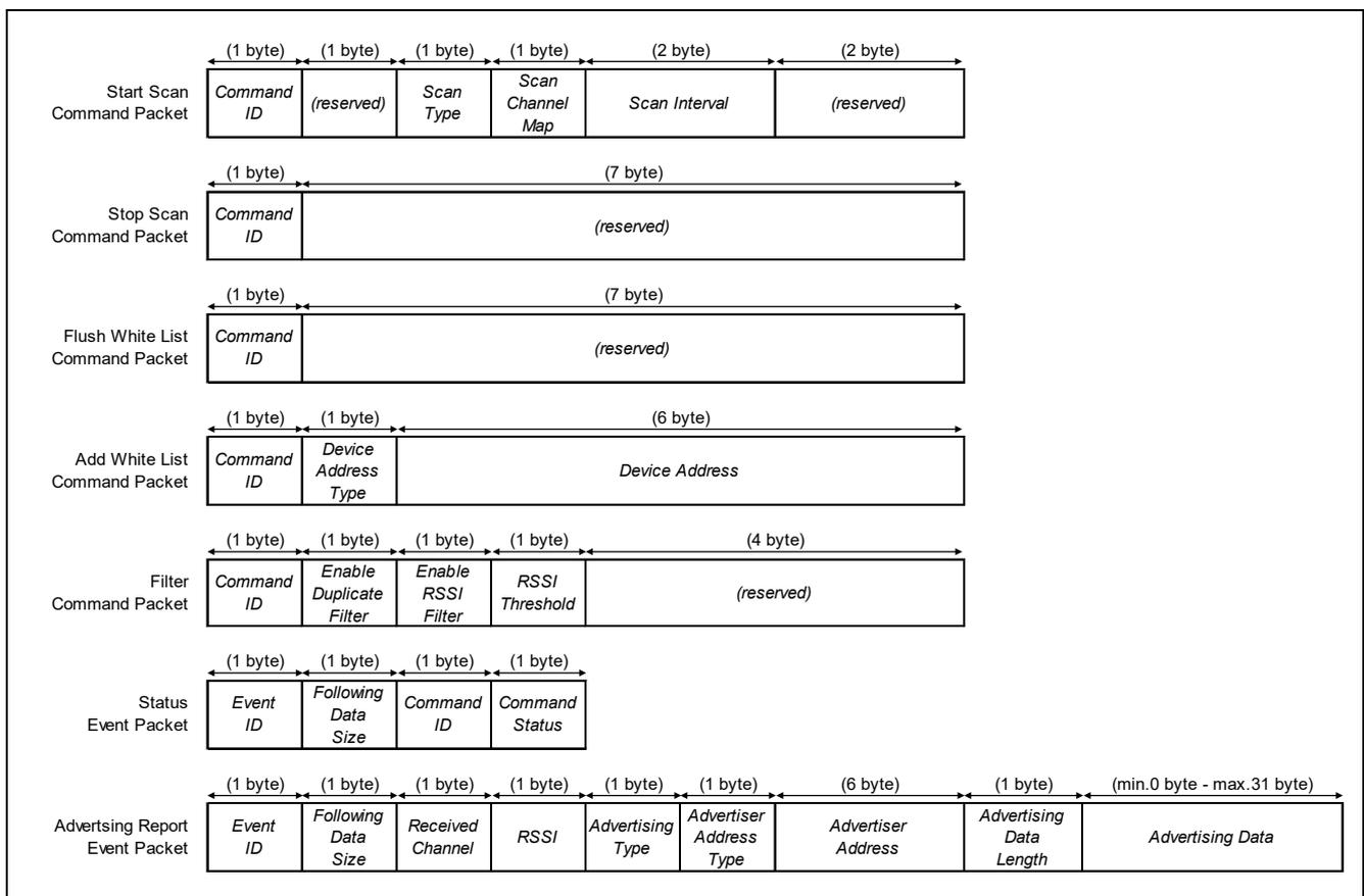
**Figure 5-2 Packet Format of the Binary-format UART communication**
