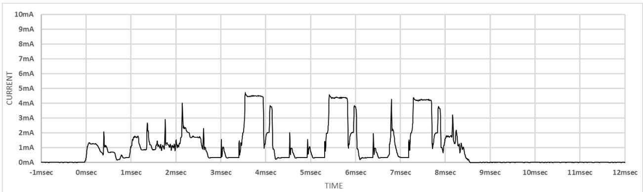
**Figure 9-13** Current Consumption Waveform of ADV\_SCAN\_IND at MCU Clock Frequency 8MHz
