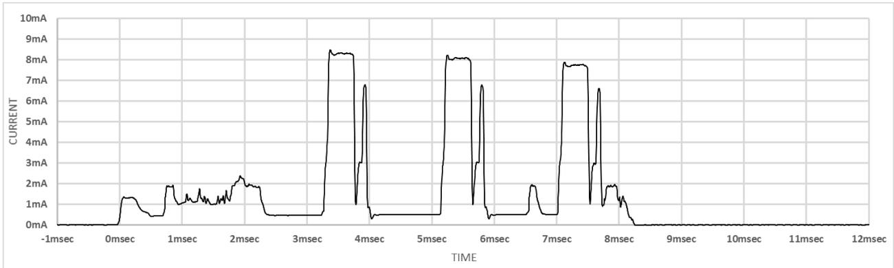
**Figure 9-12** Current Consumption Waveform of ADV\_SCAN\_IND at MCU Clock Frequency 8MHz
