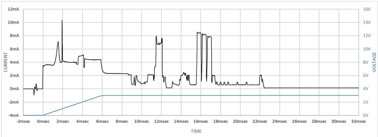
**Figure 9-3 Current Waveform of Starting-up Beacon Stack at MCU Clock Frequency 8MHz**
