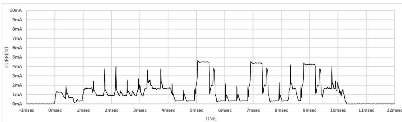
**Figure 9-9** Current Consumption Waveform of ADV\_SCAN\_IND at MCU Clock Frequency 4MHz
