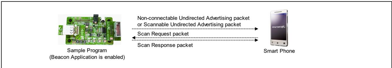
To run Beacon Application, switch both DIP switch SW6 position-1 and position-4 to OFF, and supply power via either DC jack (J1) or USB interface (CN3). After power up, Beacon Application transmits Eddystone-URL packet by default. Using smart phone application, you can receive the advertising packet. The smart phone application procedure is very much similar for both iOS device and Android device.
