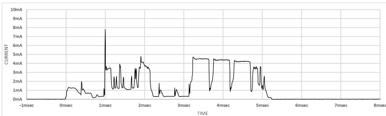
**Figure 9-15** Current Consumption Waveform of ADV\_NONCONN\_IND at MCU Clock Frequency 16MHz
