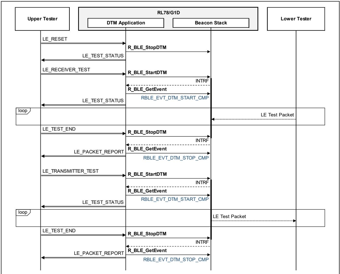
Figure 8-8 DTM Application Sequence
