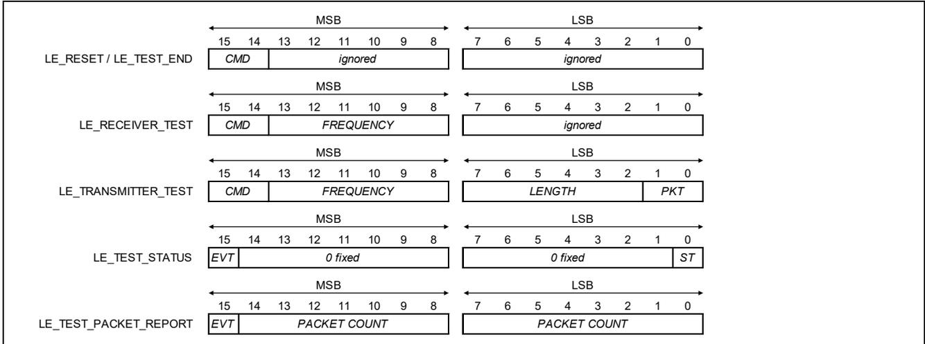
Figure 5-4 RF Test packet format
