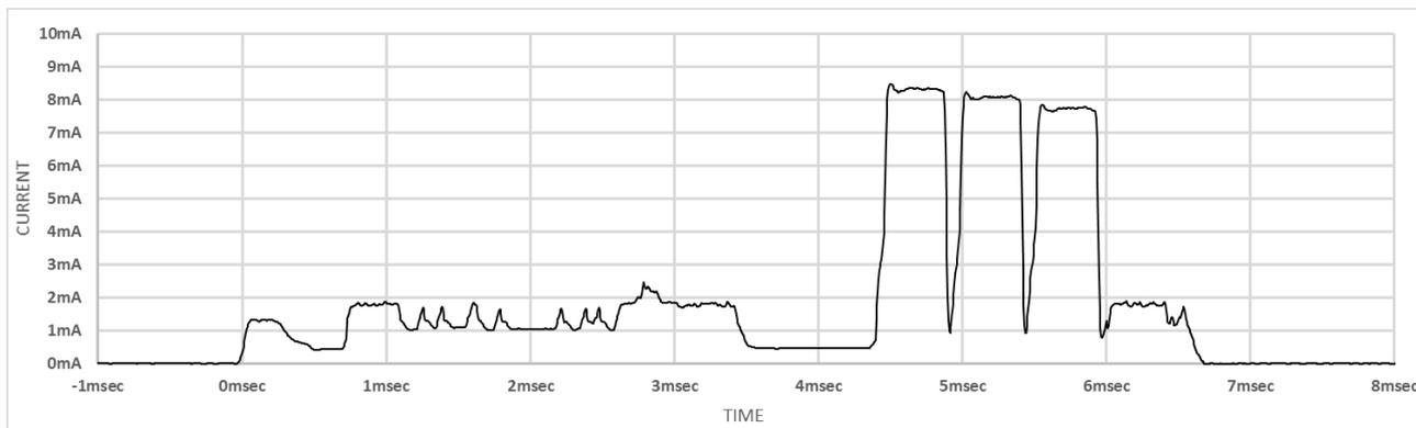
**Figure 9-6** Current Consumption Waveform of ADV\_NONCONN\_IND at MCU Clock Frequency 4MHz (not use DC-DC converter)
