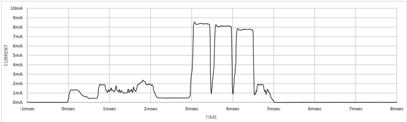
**Figure 9-10** Current Consumption Waveform of ADV\_NONCONN\_IND at MCU Clock Frequency 8MHz (not use DC-DC converter)
