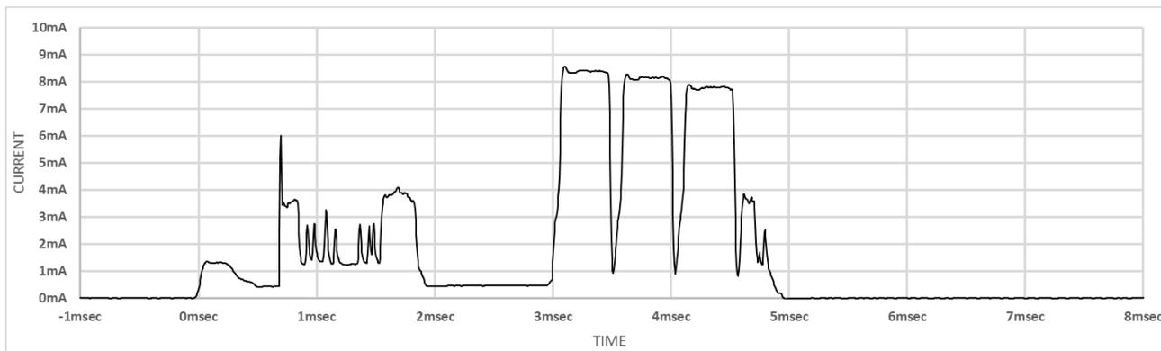
**Figure 9-14** Current Consumption Waveform of ADV\_NONCONN\_IND at MCU Clock Frequency 16MHz
