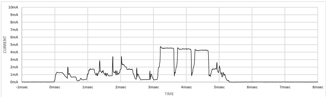
**Figure 9-11** Current Consumption Waveform of ADV\_NONCONN\_IND at MCU Clock Frequency 8MHz (use DC-DC converter)
