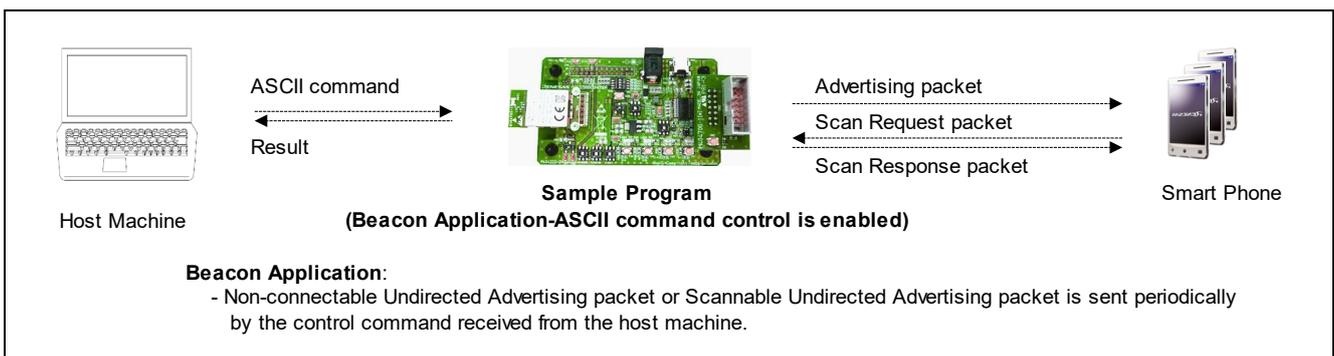
Figure 1-3 Overview of Beacon Application-ASCII command control
