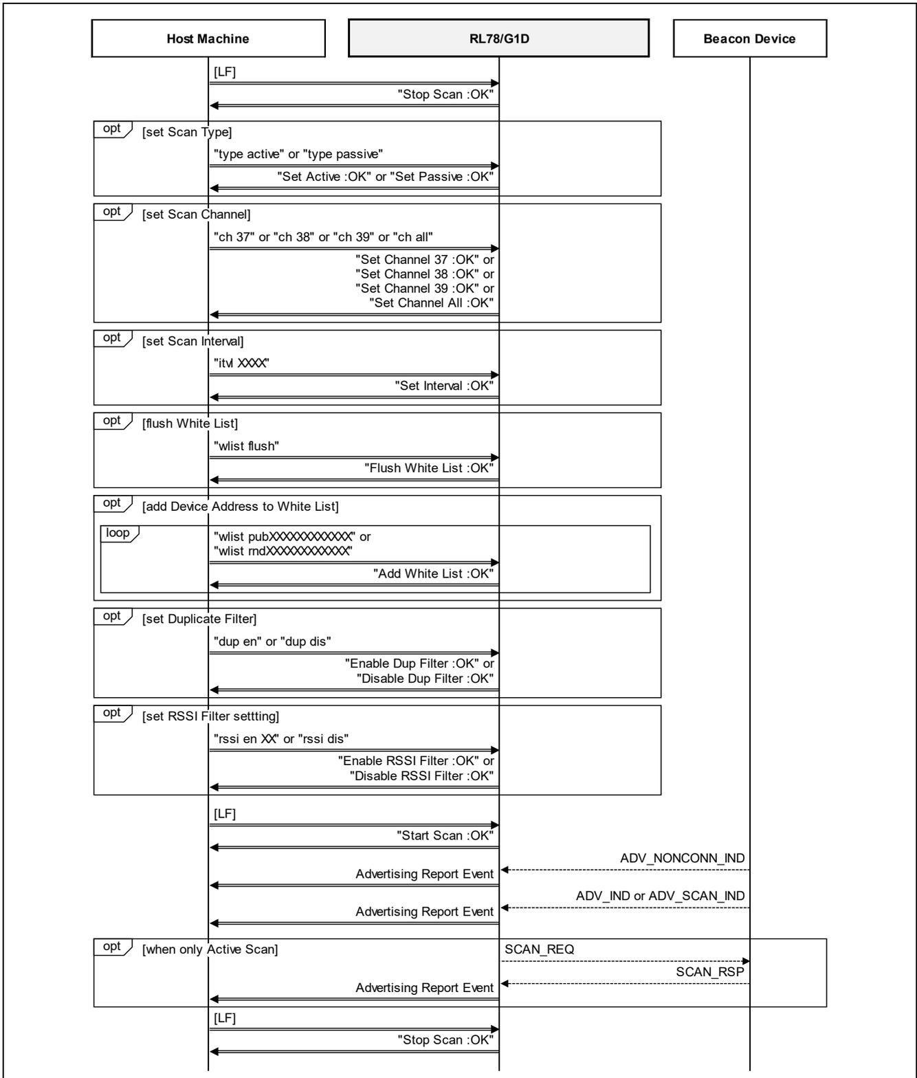
Figure 5-1 ASCII-format UART communication Sequence
